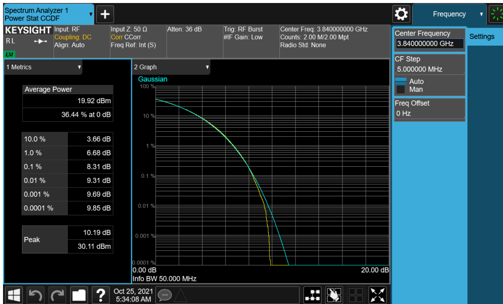
Plot 7-221. PAR Plot (NR Band n77 - 50MHz CP-OFDM 256-QAM - Full RB - ANT F)
