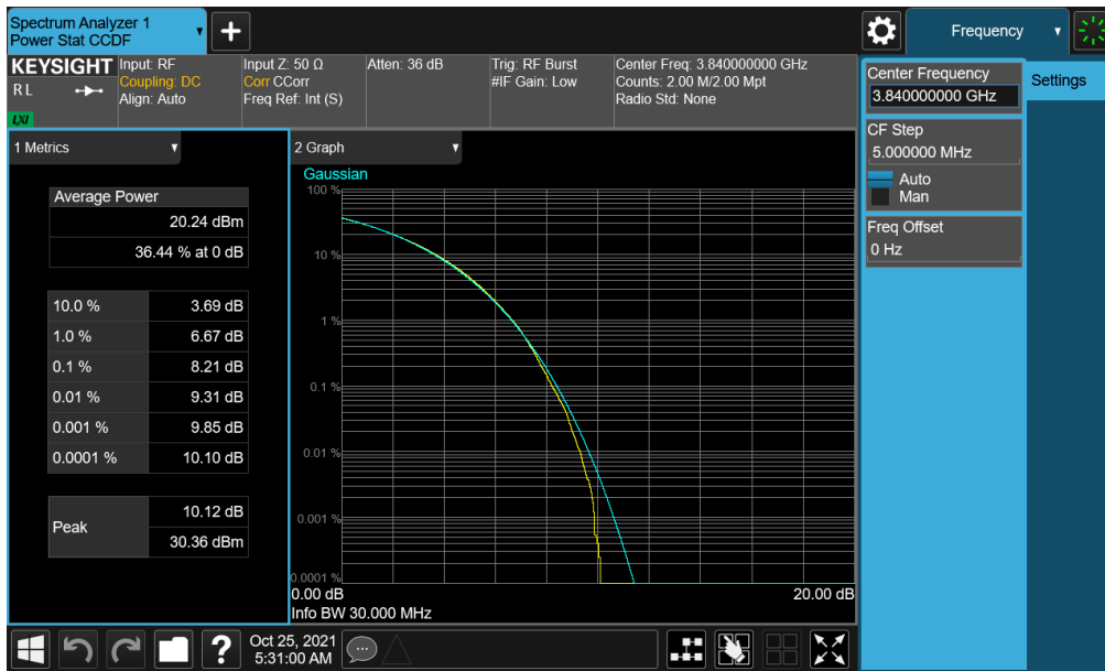
Plot 7-227. PAR Plot (NR Band n77 - 30MHz CP-OFDM 256-QAM - Full RB - ANT F)
