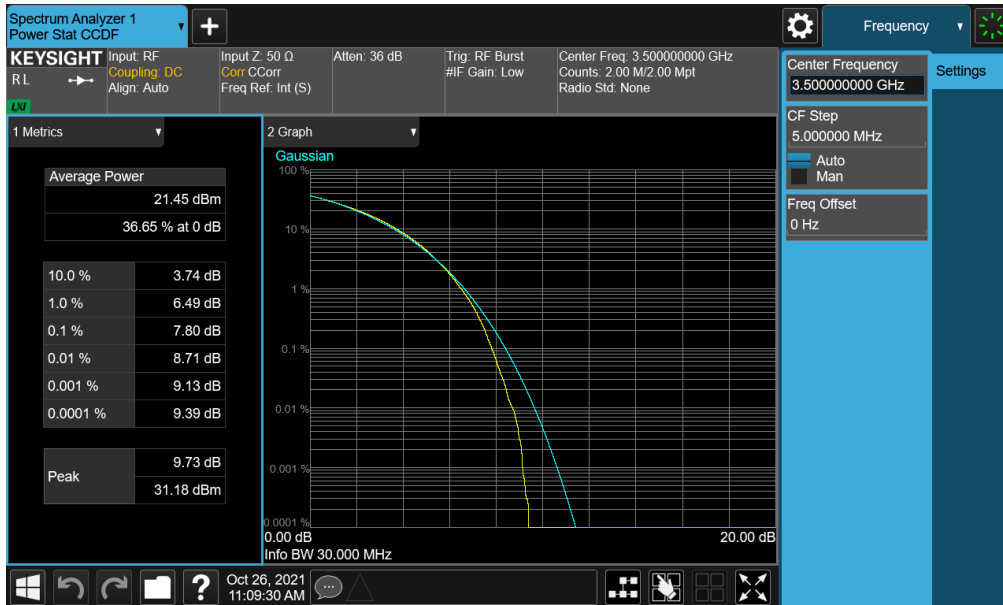
Plot 7-194. PAR Plot (NR Band n77 (DoD) - 30MHz CP-OFDM 256-QAM - Full RB - ANT F)
