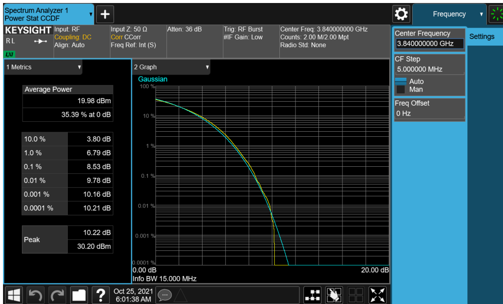
Plot 7-233. PAR Plot (NR Band n77 - 15MHz CP-OFDM 256-QAM - Full RB - ANT F)
