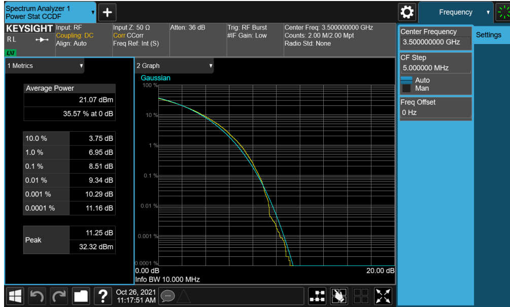
Plot 7-203. PAR Plot (NR Band n77 (DoD) - 10MHz CP-OFDM 256-QAM - Full RB - ANT F)
