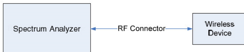
Figure 7-5. Test Instrument & Measurement Setup
