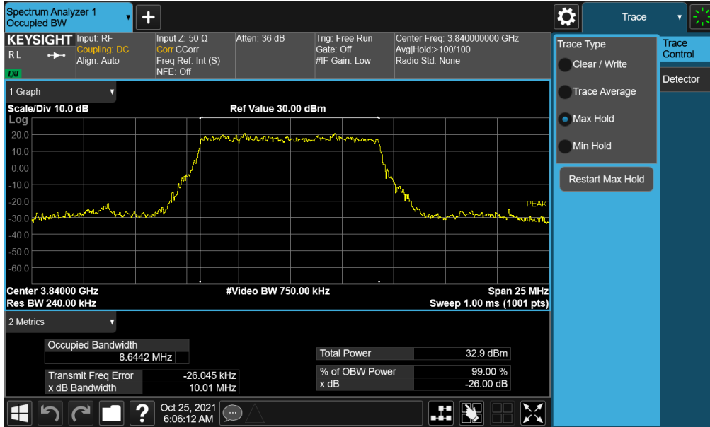
Plot 7-64. Occupied Bandwidth Plot (NR Band n77 - 10MHz \pi/2 BPSK - Full RB - ANT F)
