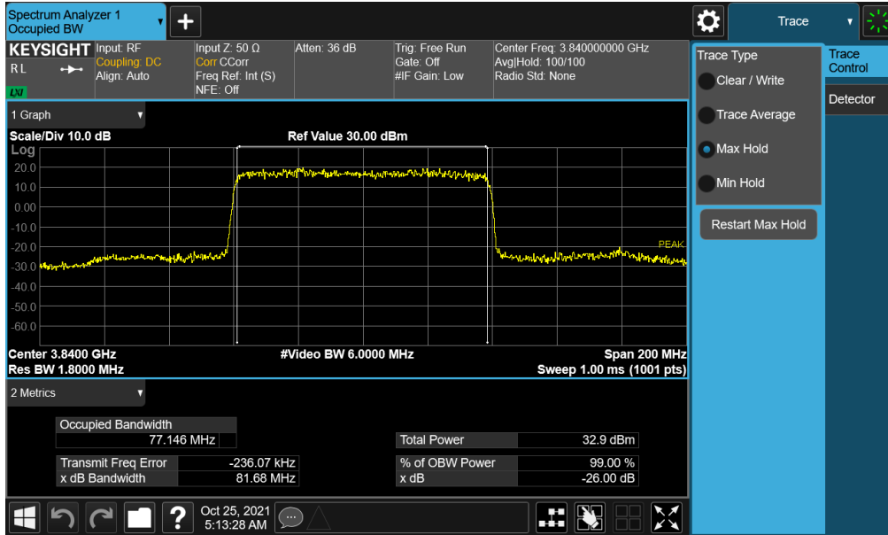
Plot 7-40. Occupied Bandwidth Plot (NR Band n77 - 80MHz \pi/2 BPSK - Full RB - ANT F)
