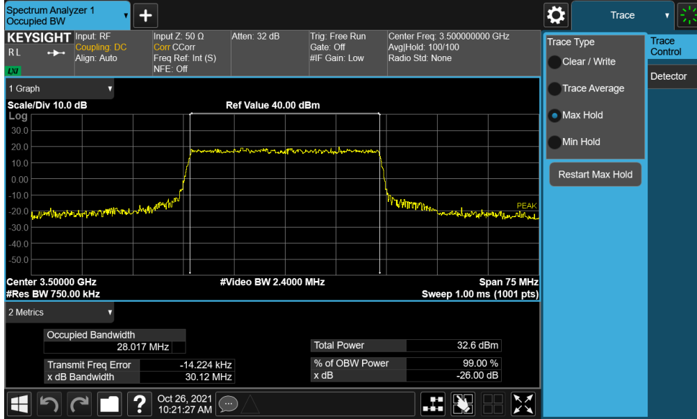
Plot 7-23. Occupied Bandwidth Plot (NR Band n77 (DoD) - 30MHz QPSK - Full RB - ANT F)
