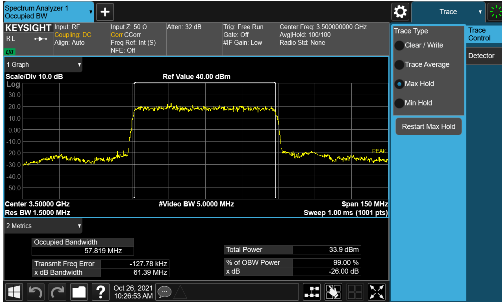
Plot 7-13. Occupied Bandwidth Plot (NR Band n77 (DoD) - 60MHz \pi/2 BPSK - Full RB - ANT F)
