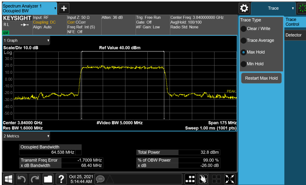
Plot 7-43. Occupied Bandwidth Plot (NR Band n77 - 70MHz \pi/2 BPSK - Full RB - ANT F)
