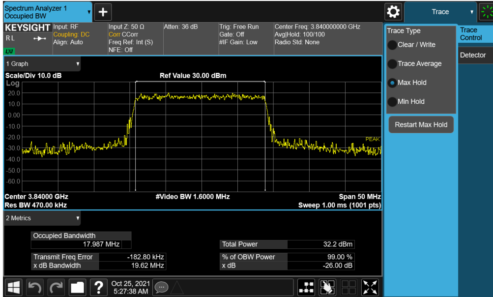
Plot 7-58. Occupied Bandwidth Plot (NR Band n77 - 20MHz \pi/2 BPSK - Full RB - ANT F)
