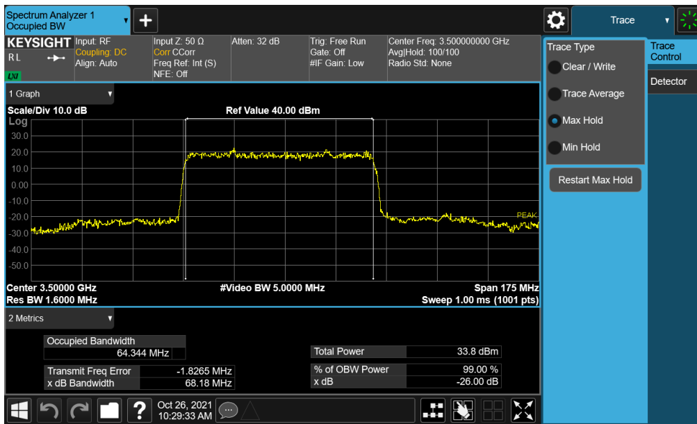
Plot 7-10. Occupied Bandwidth Plot (NR Band n77 (DoD) - 70MHz π/2 BPSK - Full RB - ANT F)
