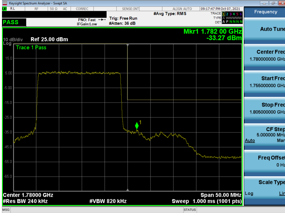
Plot 7-278. Upper Band Edge Plot (NR Band n66 – 20.0MHz - Full RB - Ant I)
