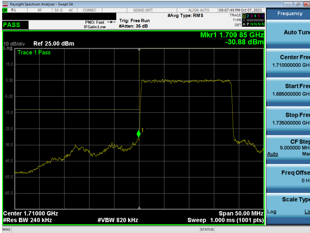
Plot 7-276. Lower Band Edge Plot (NR Band n66 – 20.0MHz - Full RB - Ant I)
