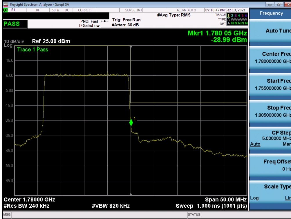
Plot 7-254. Upper Band Edge Plot (NR Band n66 – 20.0MHz - Full RB - Ant A)
