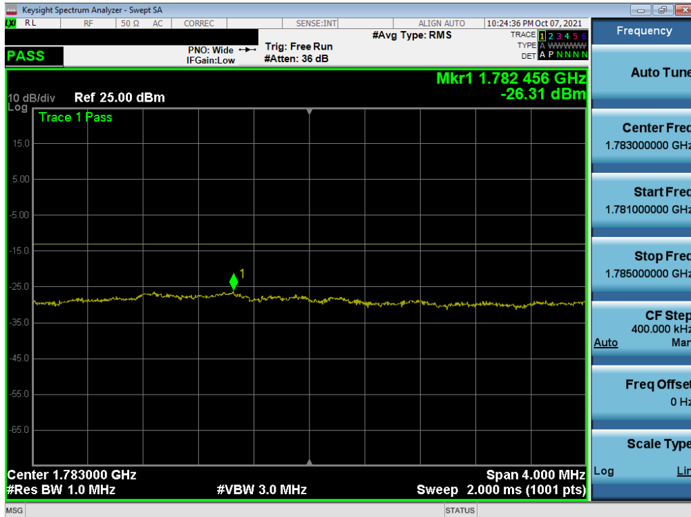
Plot 7-283. Upper Extended Band Edge Plot (NR Band n66 - 15.0MHz - Full RB - Ant I)
