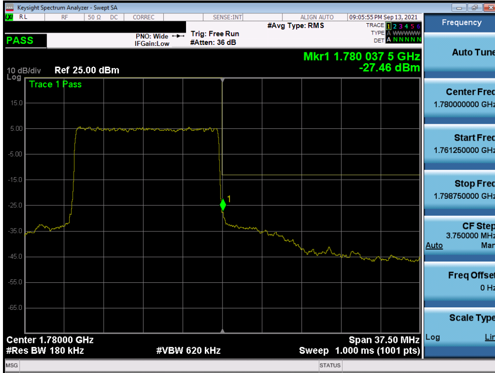
Plot 7-258. Upper Band Edge Plot (NR Band n66 – 15.0MHz - Full RB - Ant A)
