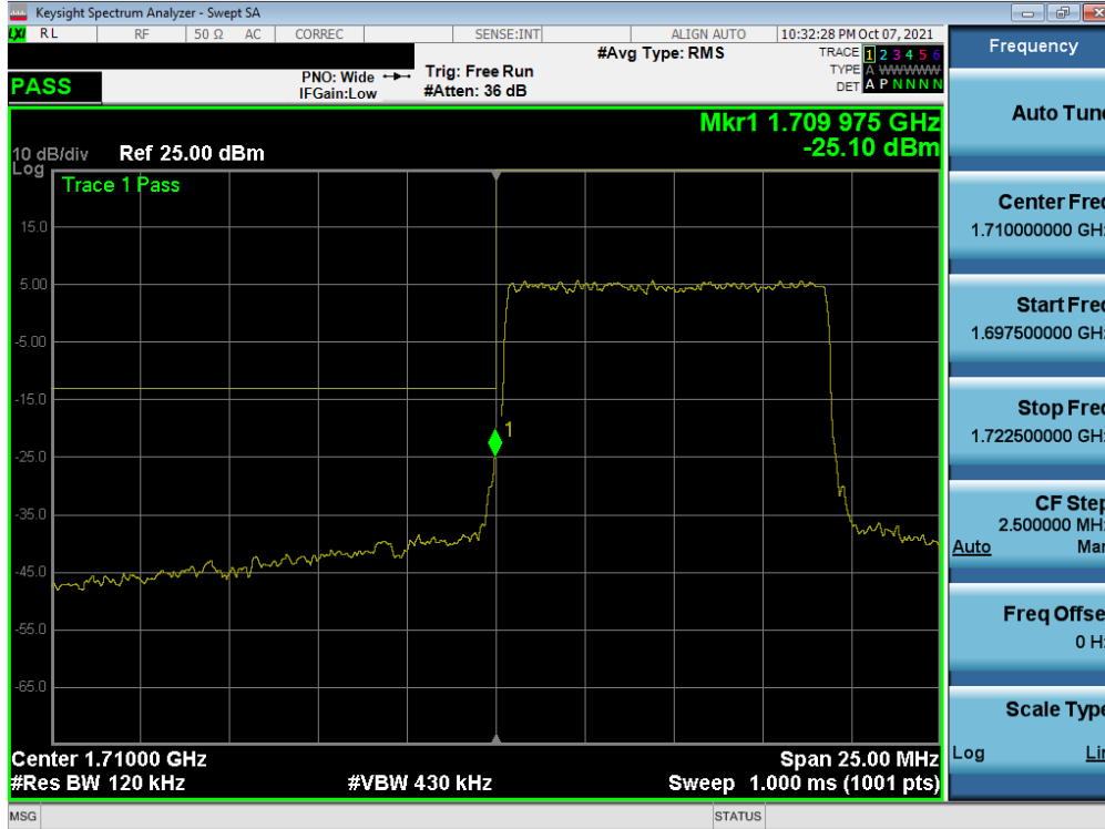
Plot 7-284. Lower Band Edge Plot (NR Band n66 – 10.0MHz - Full RB - Ant I)
