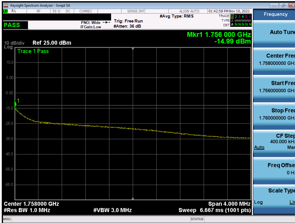
Plot 7-229. Upper Extended Band Edge Plot (LTE Band 4 - 5MHz QPSK – Full RB)
