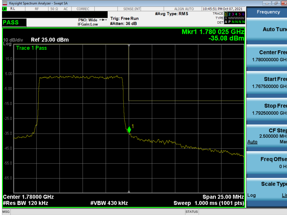
Plot 7-286. Upper Band Edge Plot (NR Band n66 – 10.0MHz - Full RB - Ant I)
