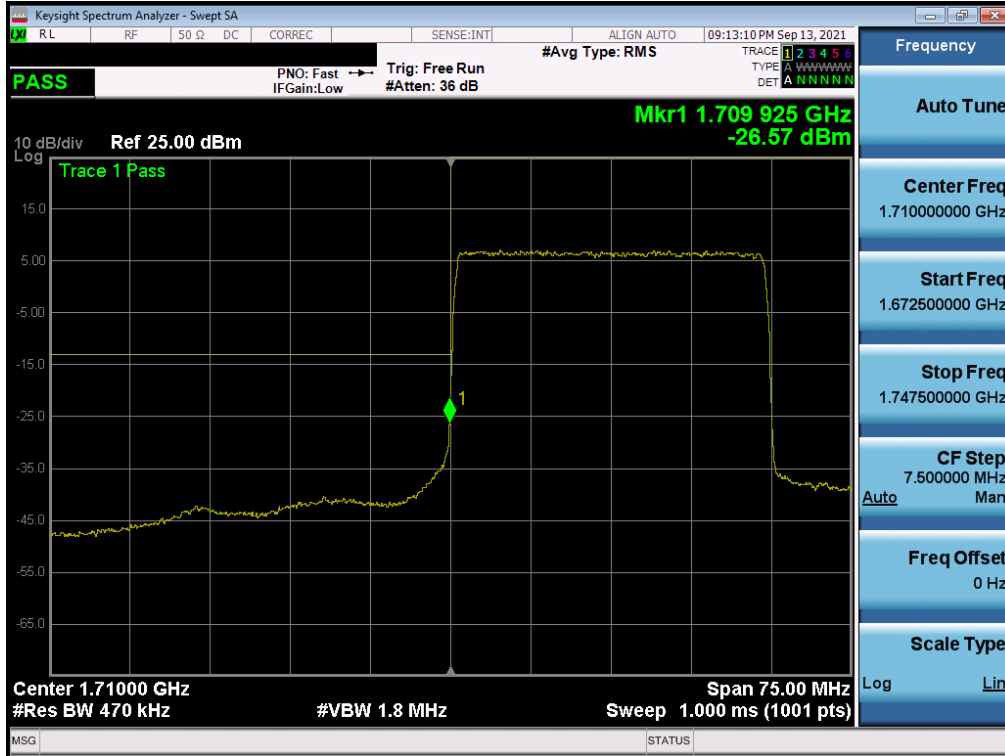
Plot 7-248. Lower Band Edge Plot (NR Band n66 – 30.0MHz - Full RB - Ant A)
