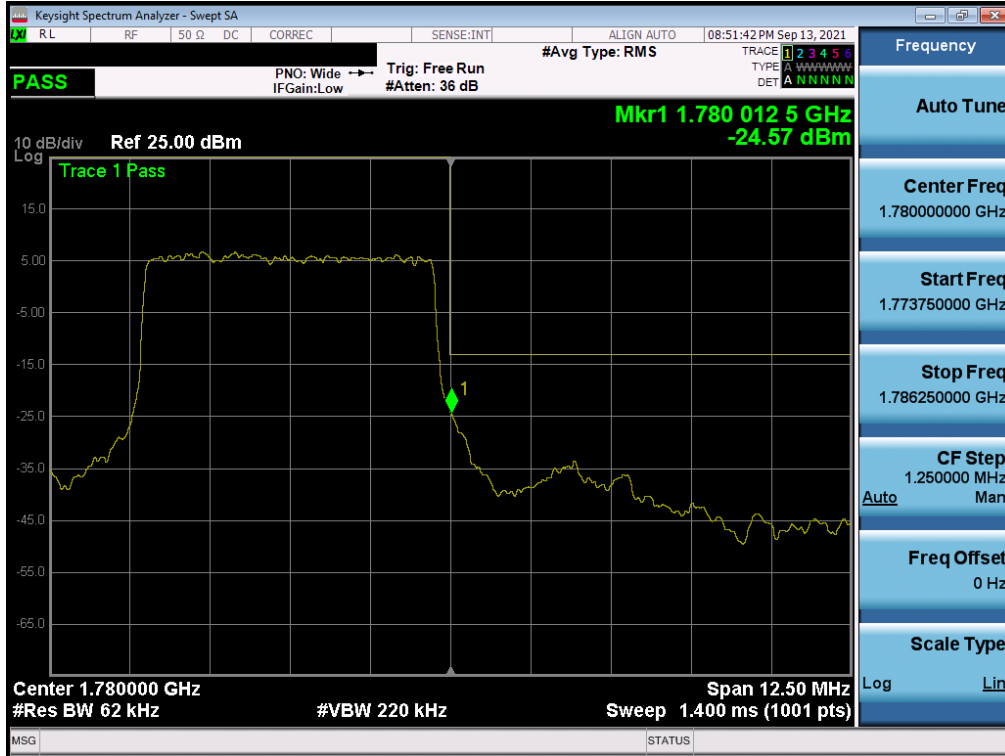
Plot 7-266. Upper Band Edge Plot (NR Band n66 – 5.0MHz - Full RB - Ant A)
