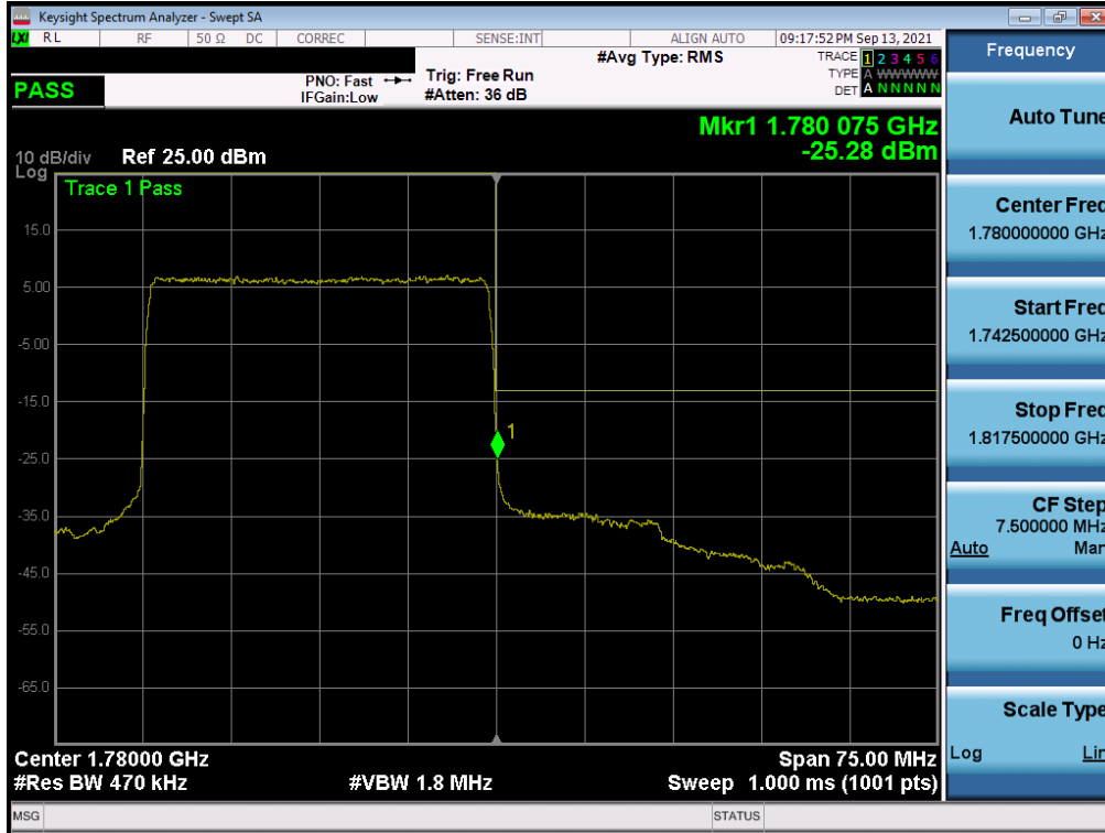
Plot 7-250. Upper Band Edge Plot (NR Band n66 – 30.0MHz - Full RB - Ant A)
