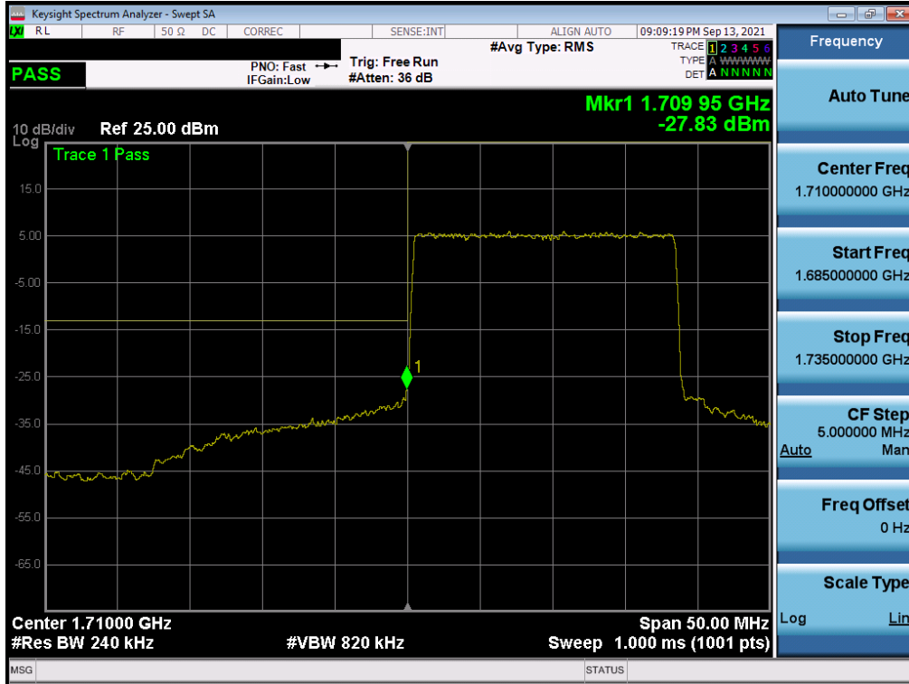
Plot 7-252. Lower Band Edge Plot (NR Band n66 – 20.0MHz - Full RB - Ant A)
