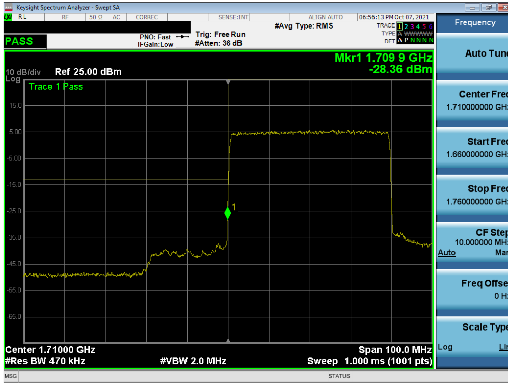
Plot 7-268. Lower Band Edge Plot (NR Band n66 – 40.0MHz - Full RB – Ant I)
