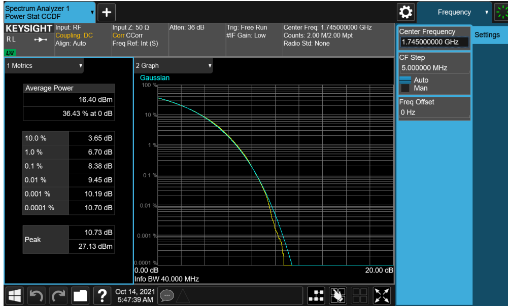
Plot 7-325. PAR Plot (NR Band n66 - 40.0MHz CP-OFDM 256-QAM - Full RB - Ant I)
