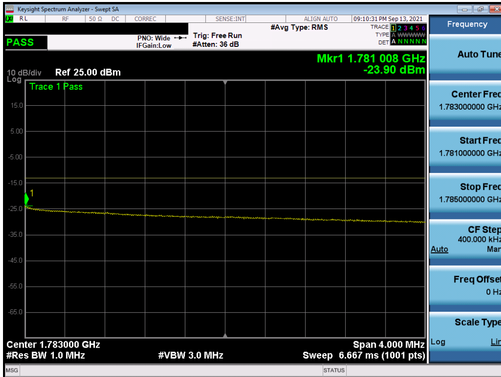
Plot 7-255. Upper Extended Band Edge Plot (NR Band n66 – 20.0MHz - Full RB - Ant A)
