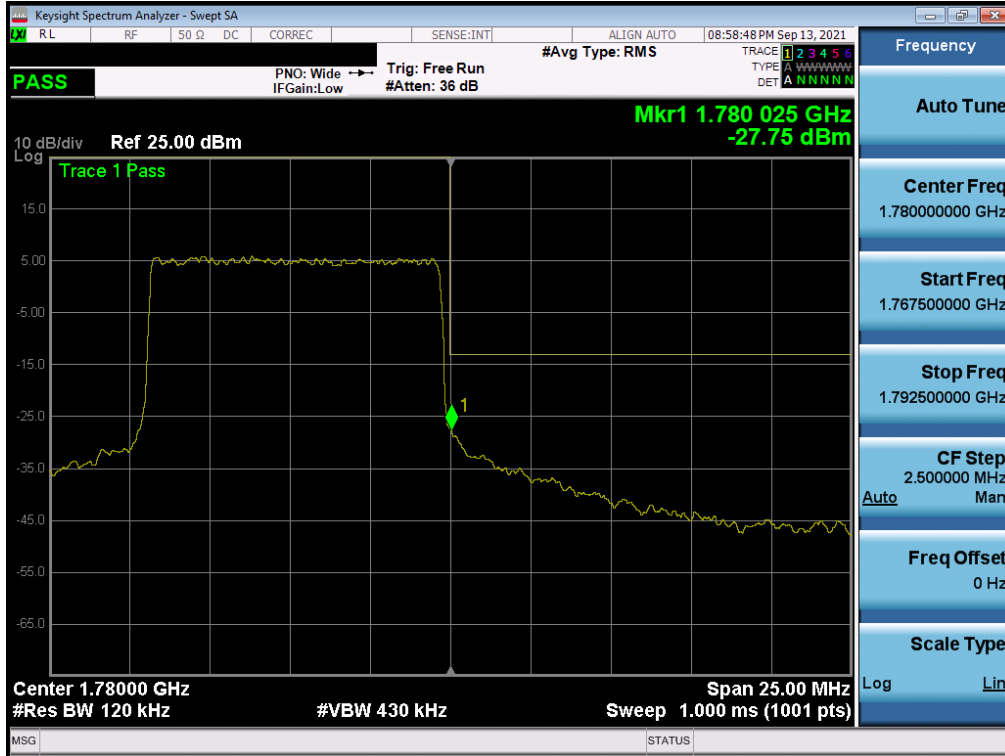
Plot 7-262. Upper Band Edge Plot (NR Band n66 – 10.0MHz - Full RB - Ant A)
