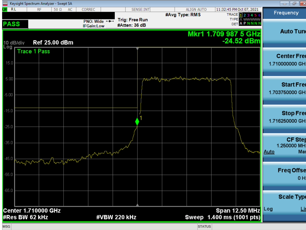
Plot 7-288. Lower Band Edge Plot (NR Band n66 – 5.0MHz - Full RB - Ant I)
