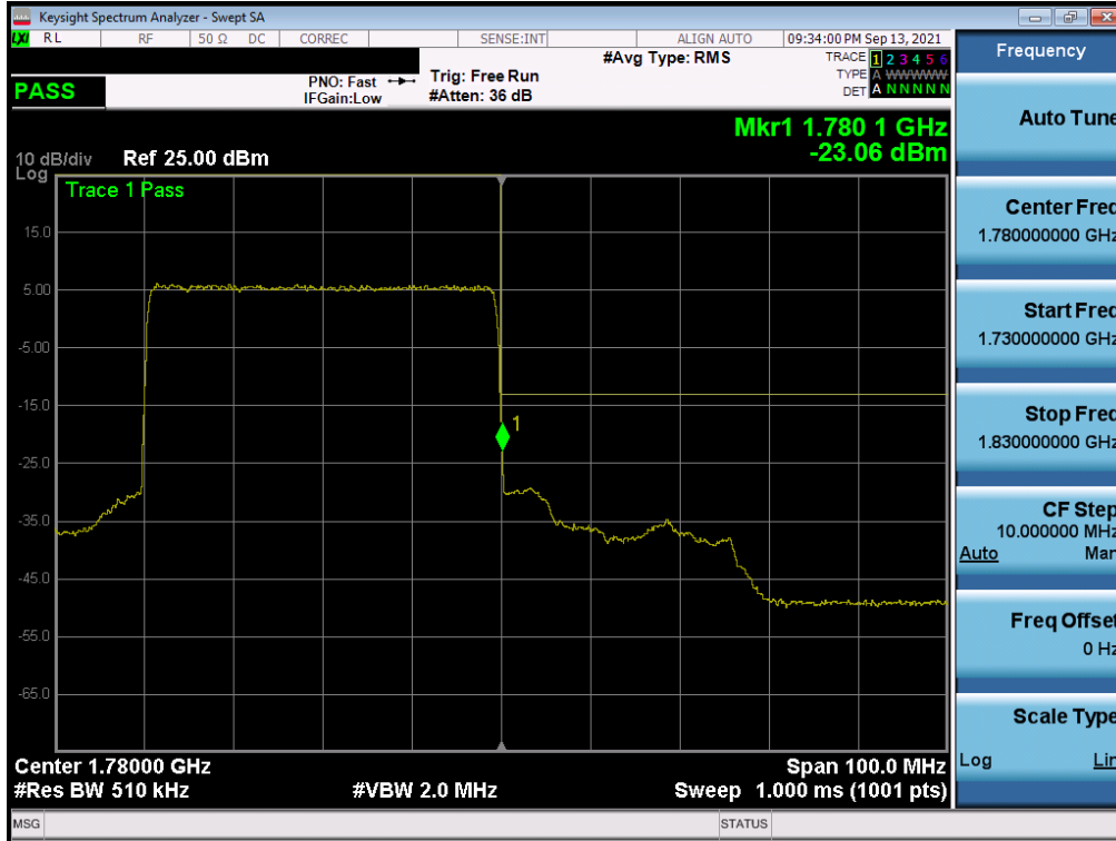
Plot 7-246. Upper Band Edge Plot (NR Band n66 – 40.0MHz - Full RB - Ant A)
