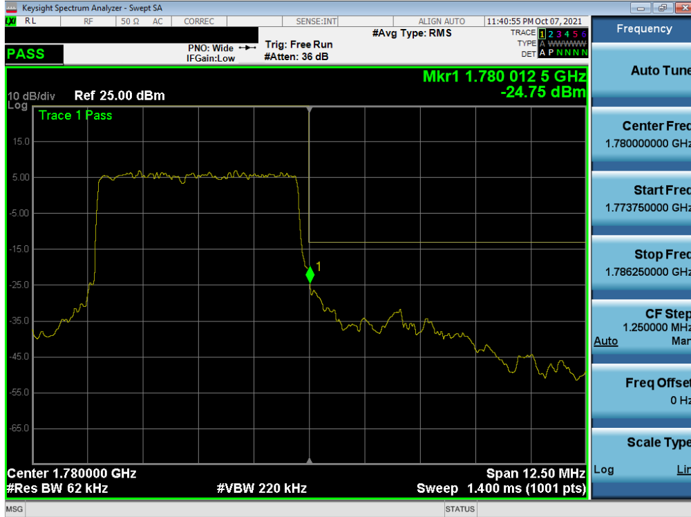
Plot 7-290. Upper Band Edge Plot (NR Band n66 – 5.0MHz - Full RB - Ant I)
