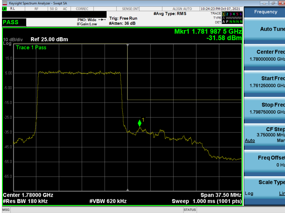
Plot 7-282. Upper Band Edge Plot (NR Band n66 - 15.0MHz - Full RB - Ant I)
