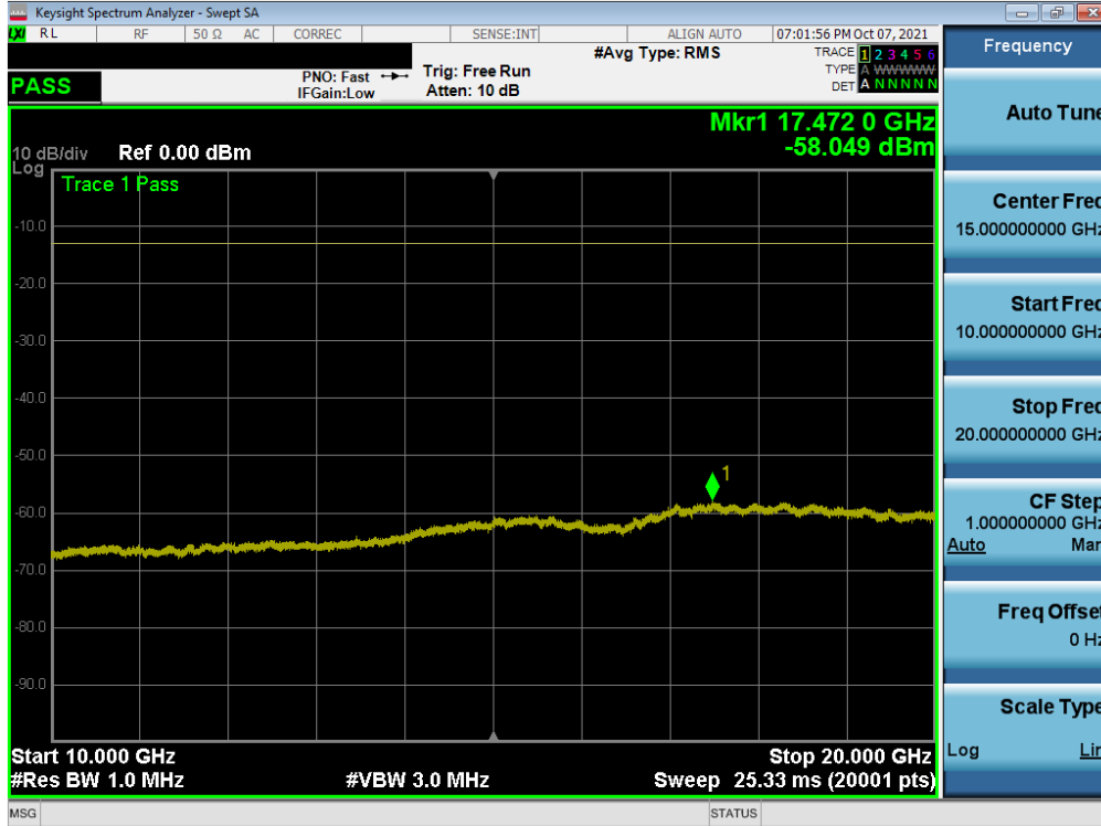
Plot 7-159. Conducted Spurious Plot (NR Band n66 - 40.0MHz - 1 RB - Low Channel - Ant I)
