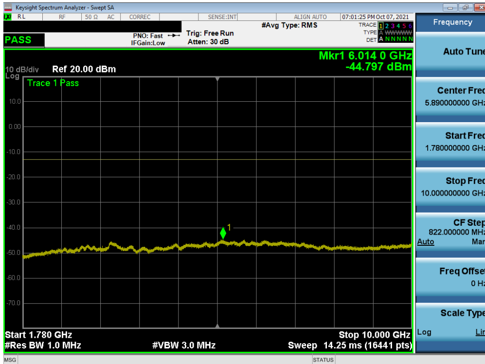
Plot 7-158. Conducted Spurious Plot (NR Band n66 - 40.0MHz - 1 RB - Low Channel - Ant I)
