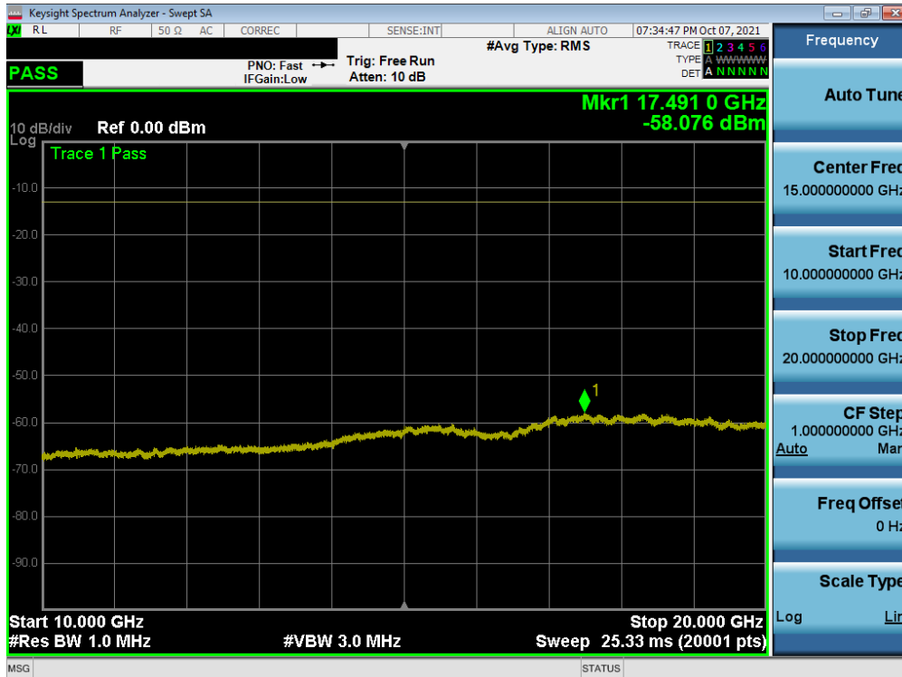
Plot 7-162. Conducted Spurious Plot (NR Band n66 - 40.0MHz - 1 RB - Mid Channel - Ant I)
