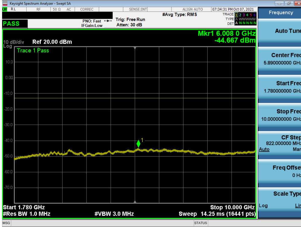
Plot 7-161. Conducted Spurious Plot (NR Band n66 - 40.0MHz - 1 RB - Mid Channel - Ant I)
