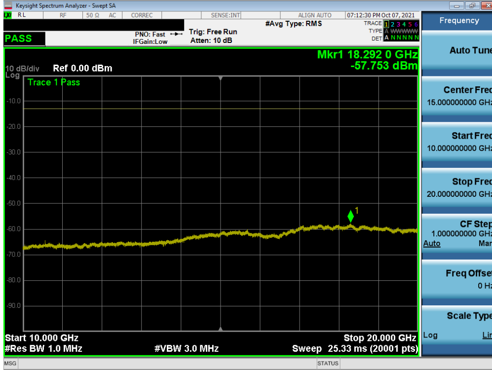
Plot 7-165. Conducted Spurious Plot (NR Band n66 - 40.0MHz - 1 RB - High Channel - Ant I)
