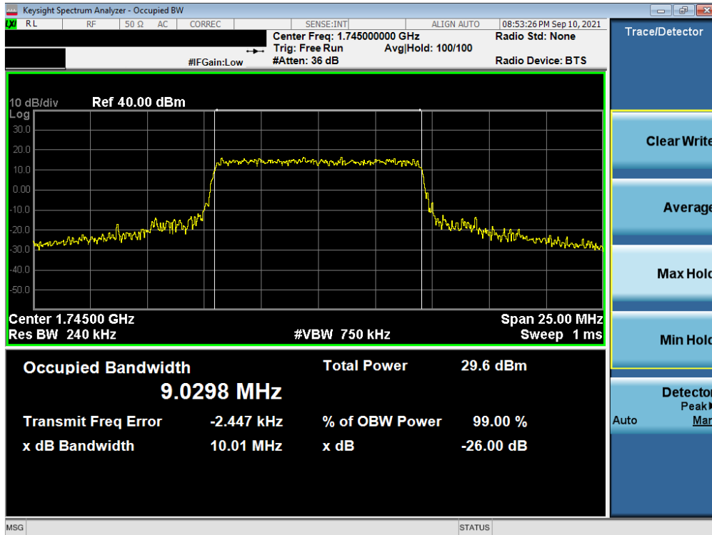
Plot 7-48. Occupied Bandwidth Plot (LTE Band 66/4 - 10MHz 16-QAM - Full RB)
