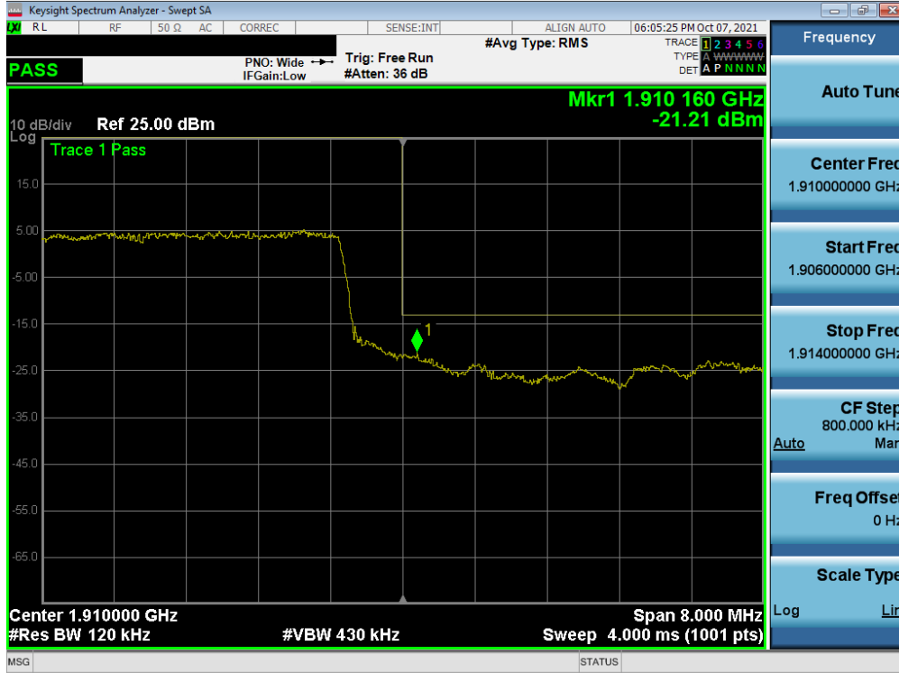
Plot 7-201. Upper Band Edge Plot (NR Band n2 - 10MHz QPSK – Full RB)
