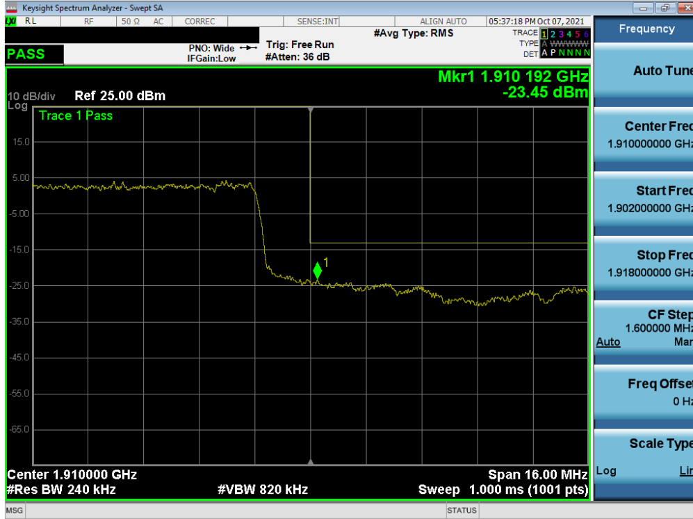
Plot 7-189. Upper Band Edge Plot (NR Band n2 - 20MHz QPSK – Full RB)
