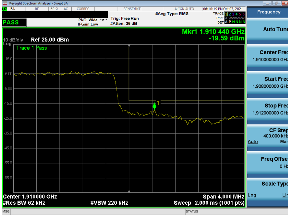
Plot 7-207. Upper Band Edge Plot (NR Band n2 – 5MHz QPSK – Full RB)
