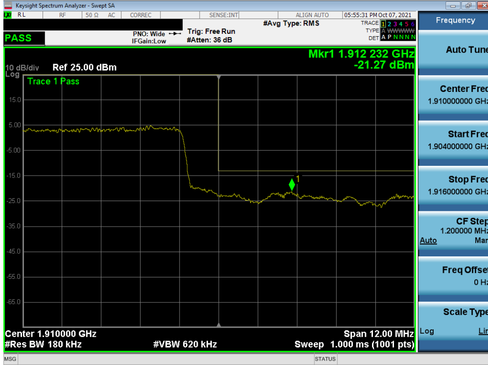
Plot 7-195. Upper Band Edge Plot (NR Band n2 - 15MHz QPSK – Full RB)
