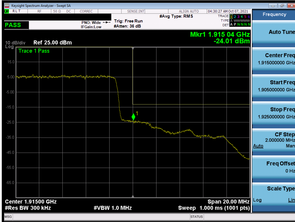
Plot 7-185. Upper Band Edge Plot (NR Band n25 - 25MHz QPSK – Full RB)
