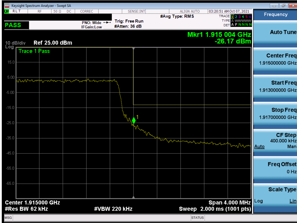
Plot 7-209. Upper Band Edge Plot (NR Band n25 – 5MHz QPSK – Full RB)
