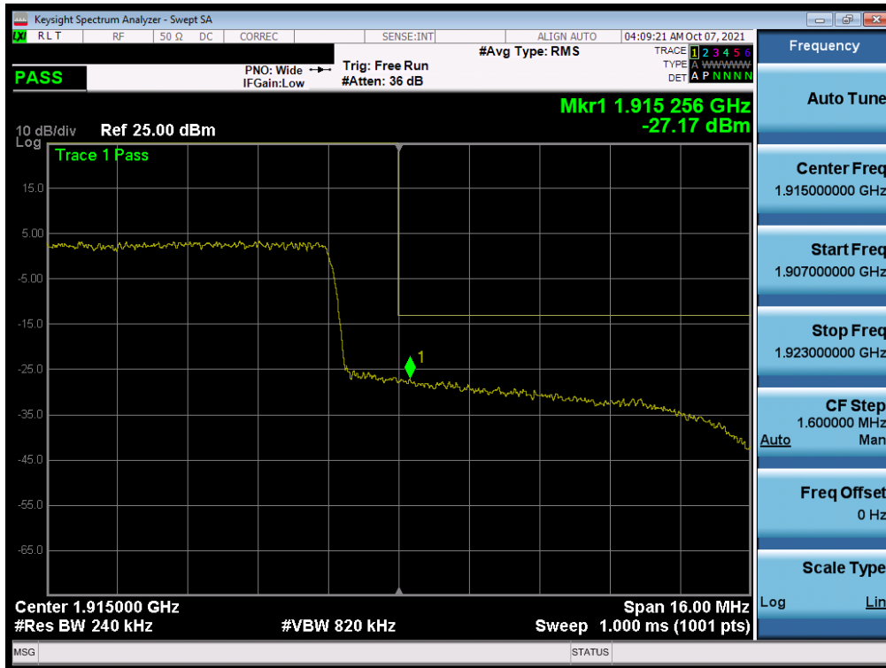
Plot 7-191. Upper Band Edge Plot (NR Band n25 - 20MHz QPSK – Full RB)
