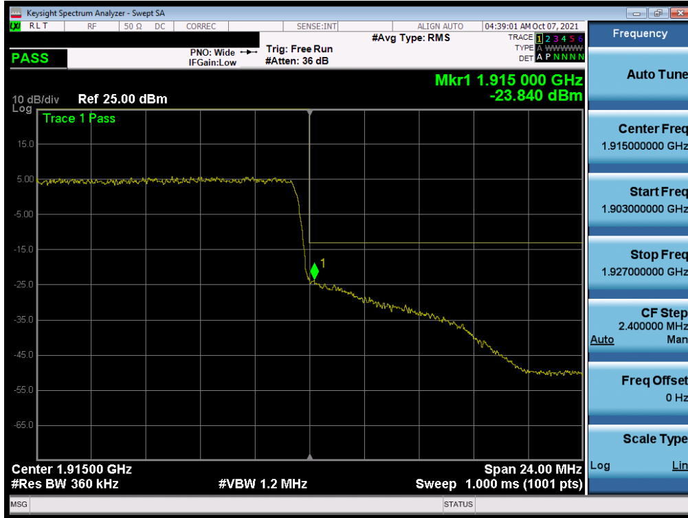
Plot 7-181. Upper Band Edge Plot (NR Band n25 - 30MHz QPSK – Full RB)
