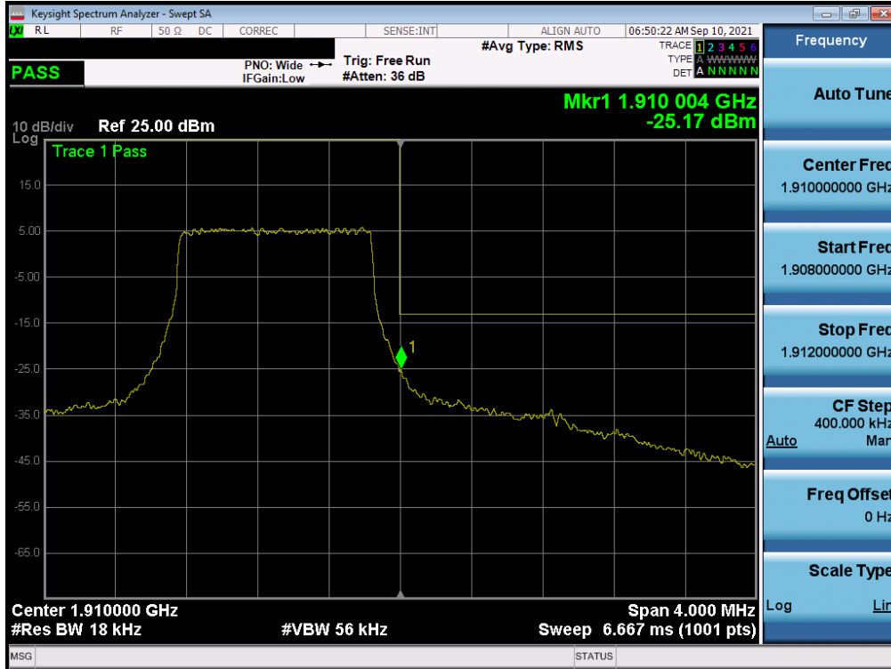
Plot 7-135. Upper Band Edge Plot (LTE Band 2 – 1.4MHz QPSK – Full RB)
