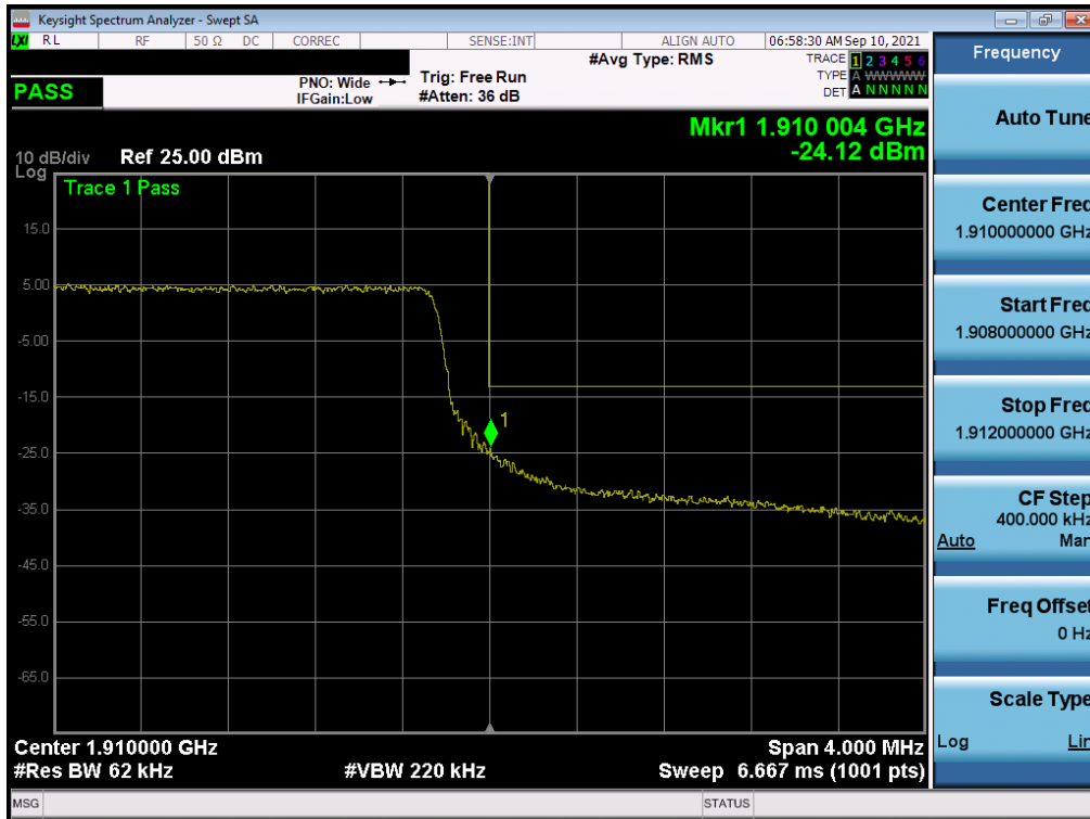
Plot 7-123. Upper Band Edge Plot (LTE Band 2 - 5MHz QPSK – Full RB)
