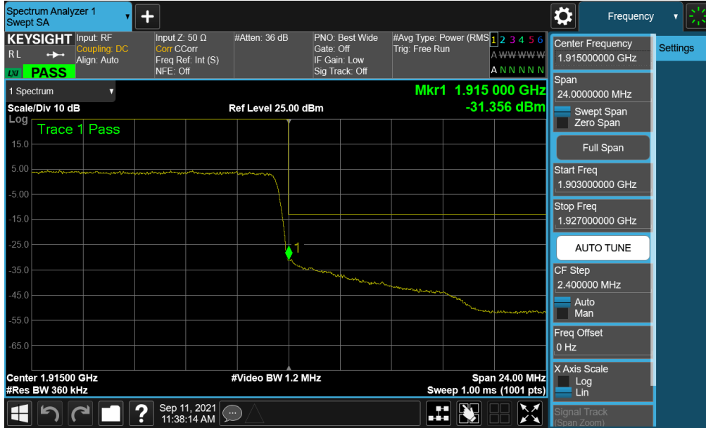
Plot 7-145. Upper Band Edge Plot (NR Band n25 - 30MHz QPSK – Full RB)
