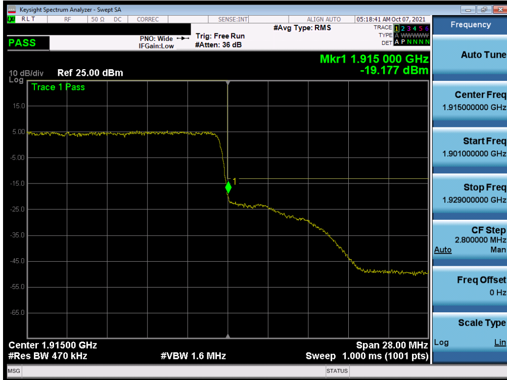
Plot 7-177. Upper Band Edge Plot (NR Band n25 - 40MHz QPSK – Full RB)
