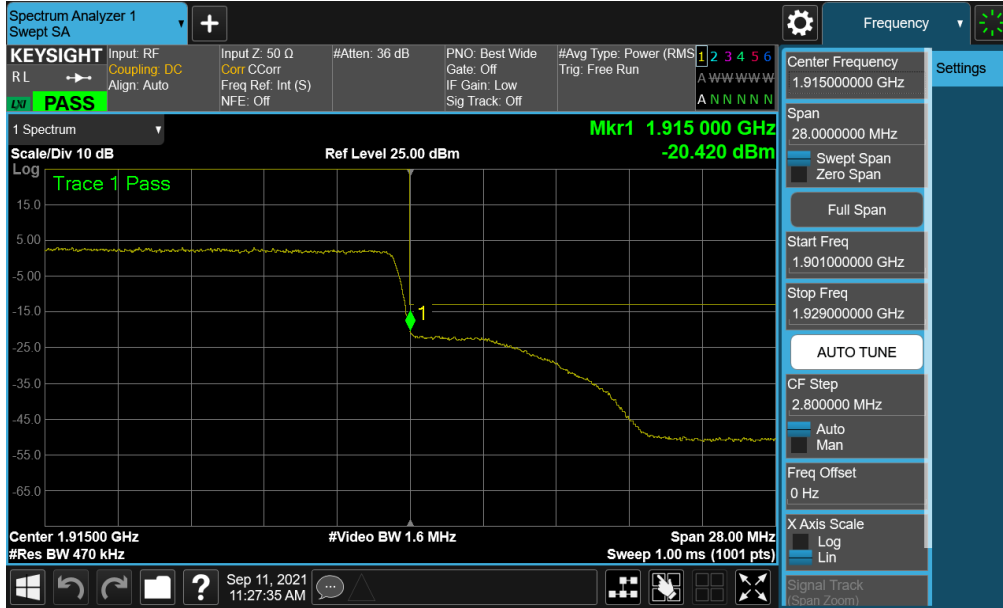
Plot 7-141. Upper Band Edge Plot (NR Band n25 - 40MHz QPSK – Full RB)
