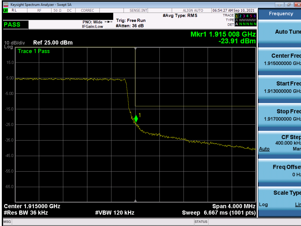
Plot 7-131. Upper Band Edge Plot (LTE Band 25 - 3MHz QPSK – Full RB)
