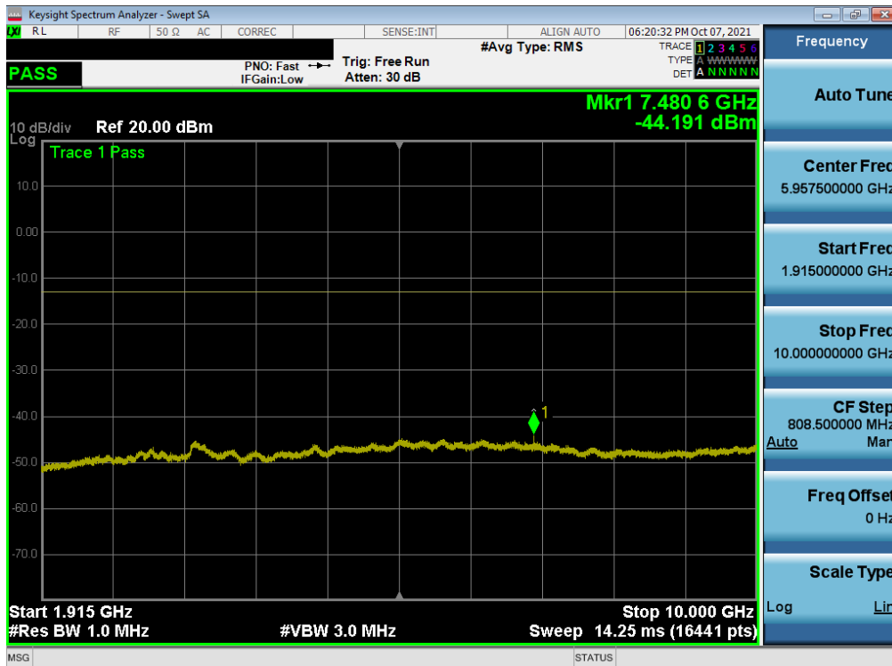
Plot 7-77. Conducted Spurious Plot (NR Band n25 - 40.0MHz - 1RB - Low Channel)
