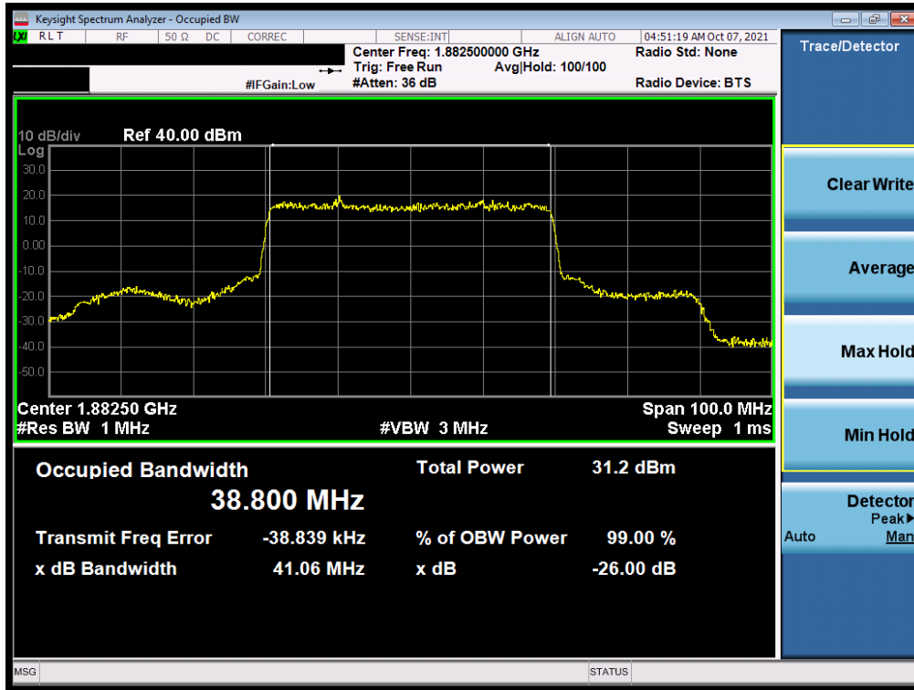
Plot 7-34. Occupied Bandwidth Plot (NR Band n25 - 40.0MHz DFT-s-OFDM BPSK - Full RB)
