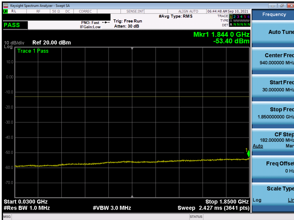
Plot 7-61. Conducted Spurious Plot (LTE Band 25/2 - 20MHz QPSK - 1RB - Mid Channel)
