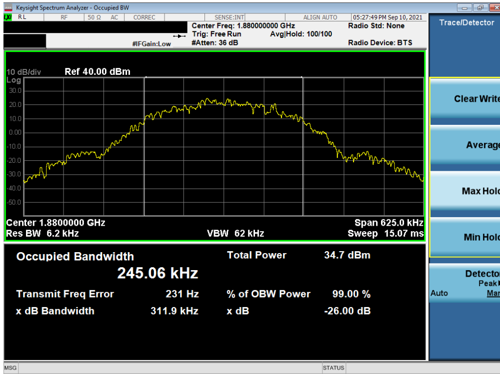
Plot 7-55. Occupied Bandwidth Plot (GPRS, Ch. 661)
