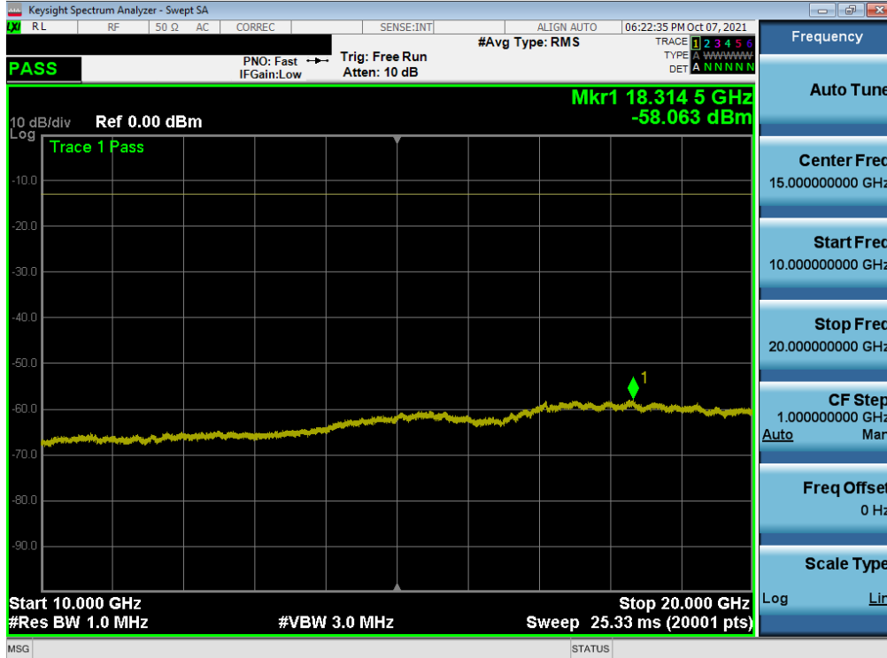
Plot 7-84. Conducted Spurious Plot (NR Band n25 - 40.0MHz - 1RB - High Channel)
