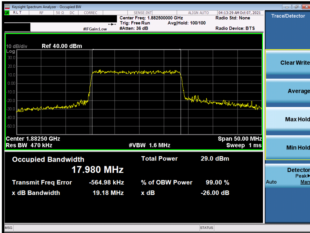
Plot 7-45. Occupied Bandwidth Plot (NR Band n25/2 - 20.0MHz CP-OFDM 16QAM - Full RB)
