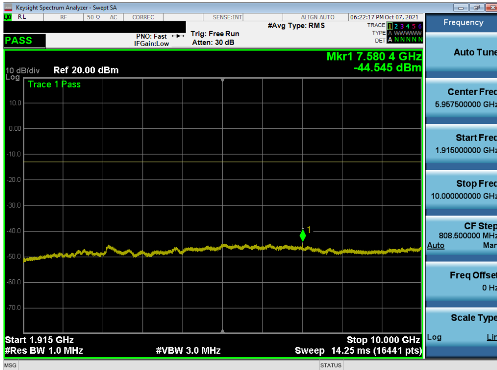
Plot 7-83. Conducted Spurious Plot (NR Band n25 - 40.0MHz - 1RB - High Channel)
