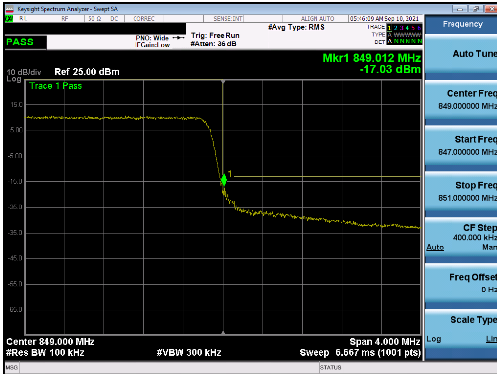
Plot 7-73. Upper Band Edge Plot (LTE Band 26/5 - 3MHz QPSK – Full RB)
