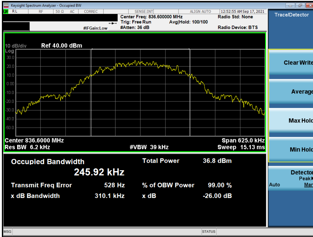
Plot 7-1. Occupied Bandwidth Plot (GPRS, Ch. 190)
