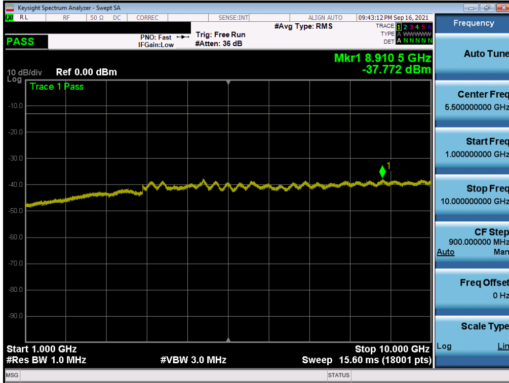
Plot 7-55. Conducted Spurious Plot (NR Band n5 - 20.0MHz - 1 RB - Low Channel)
