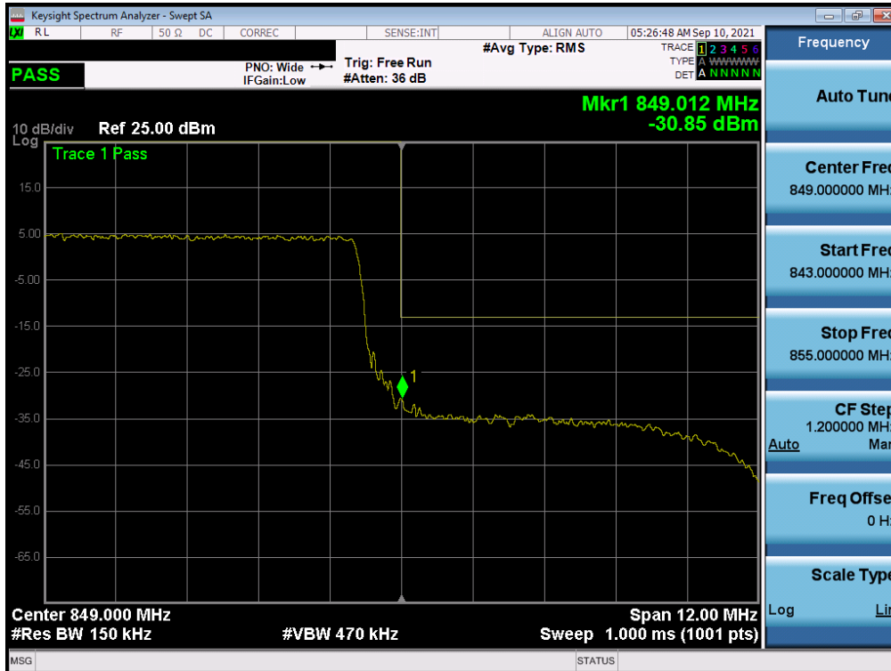
Plot 7-67. Upper Band Edge Plot (LTE Band 26 - 15MHz QPSK – Full RB)
