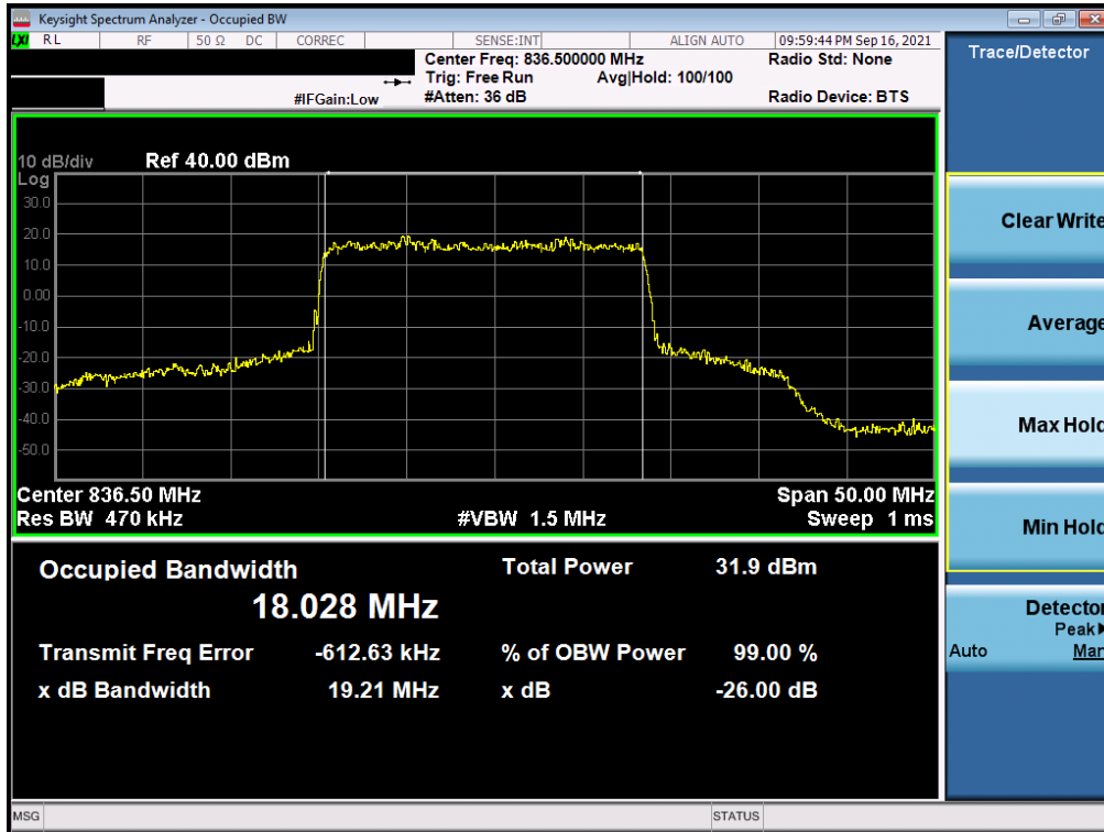
Plot 7-14. Occupied Bandwidth Plot (NR Band n5 - 20MHz \pi/2 BPSK - Full RB)
