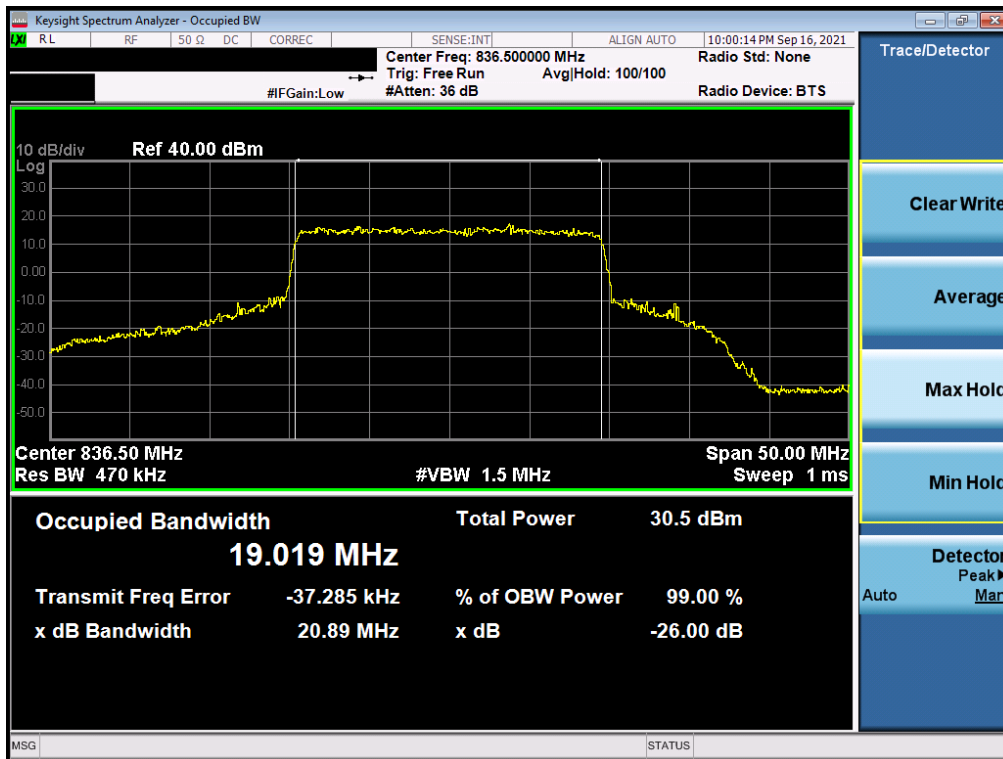
Plot 7-15. Occupied Bandwidth Plot (NR Band n5 - 20MHz QPSK - Full RB)
