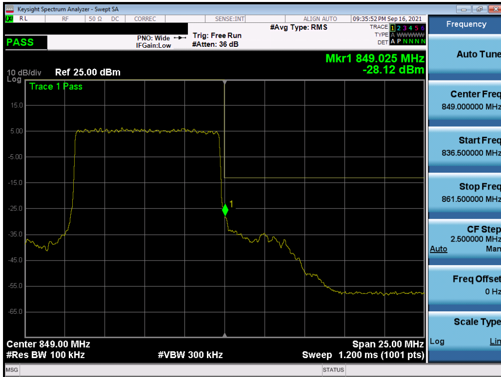
Plot 7-81. Upper Band Edge Plot (NR Band n5 – 10.0MHz - Full RB)
