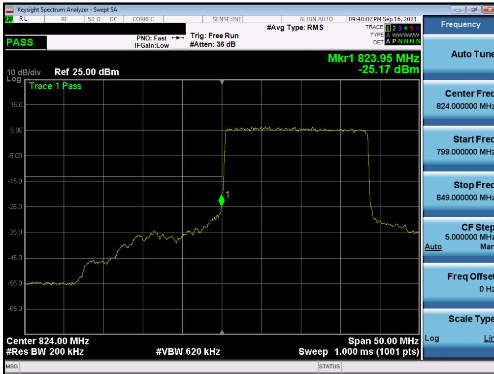
Plot 7-76. Lower Band Edge Plot (NR Band n5 – 20.0MHz - Full RB)
