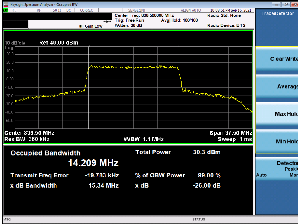
Plot 7-18. Occupied Bandwidth Plot (NR Band n5 - 15MHz QPSK - Full RB)
