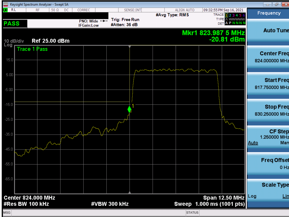
Plot 7-82. Lower Band Edge Plot (NR Band n5 – 5.0MHz - Full RB)
