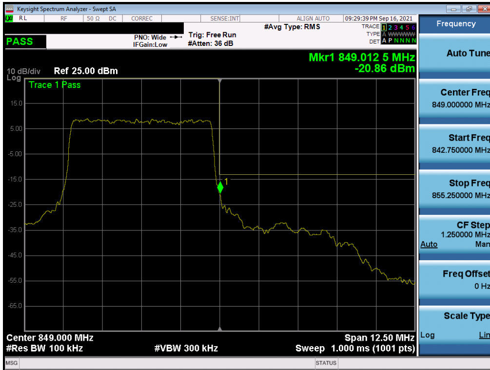
Plot 7-83. Upper Band Edge Plot (NR Band n5 – 5.0MHz - Full RB)
