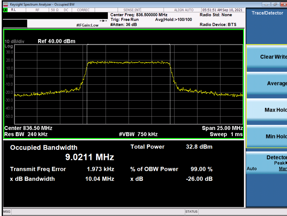
Plot 7-6. Occupied Bandwidth Plot (LTE Band 26/5 - 10MHz QPSK - Full RB)
