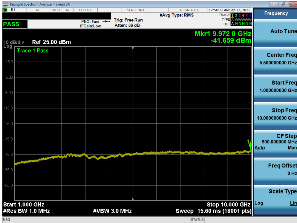
Plot 7-95. Conducted Spurious Plot (Band 5 – 10.0MHz QPSK – PCC 1/0 SCC 1/49 – High Channel)
