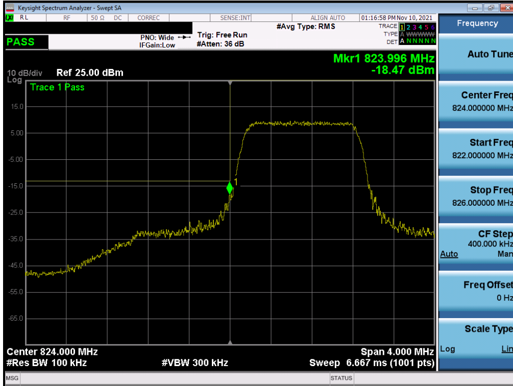
Plot 7-74. Lower Band Edge Plot (LTE Band 26/5 – 1.4MHz QPSK – Full RB)
