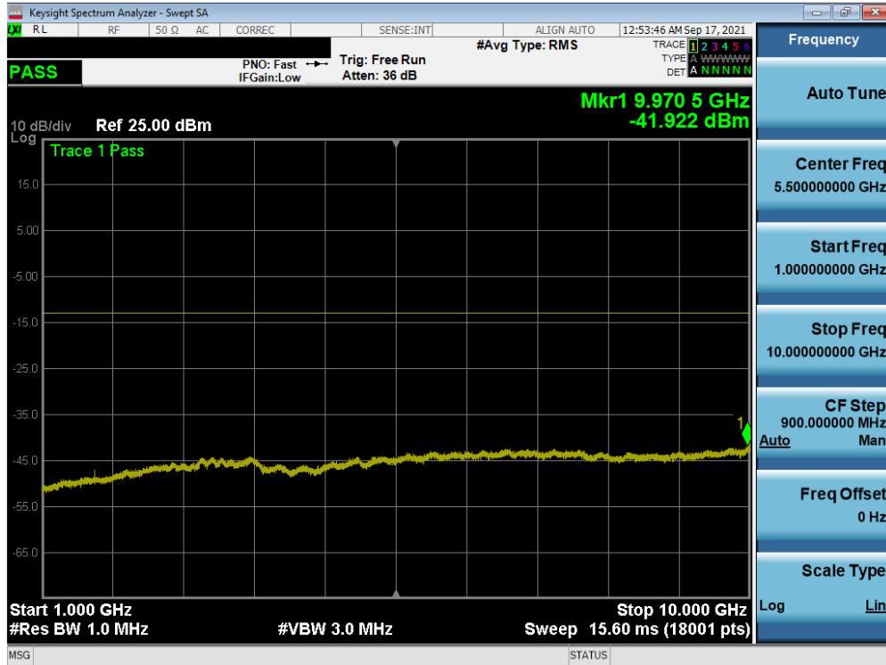
Plot 7-91. Conducted Spurious Plot (Band 5 – 10.0MHz QPSK – PCC 1/49 SCC 1/0 – Mid Channel)
