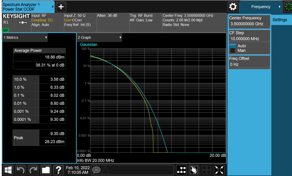
Plot 7-197. PAR Plot (NR Band n77 (DoD)- 20MHz CP-OFDM 256-QAM - Full RB - Ant F)
