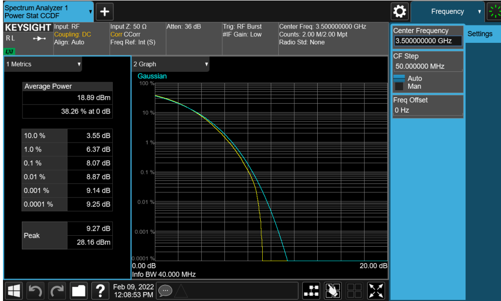
Plot 7-191. PAR Plot (NR Band n77 (DoD)- 40MHz CP-OFDM 256-QAM - Full RB - Ant F)
