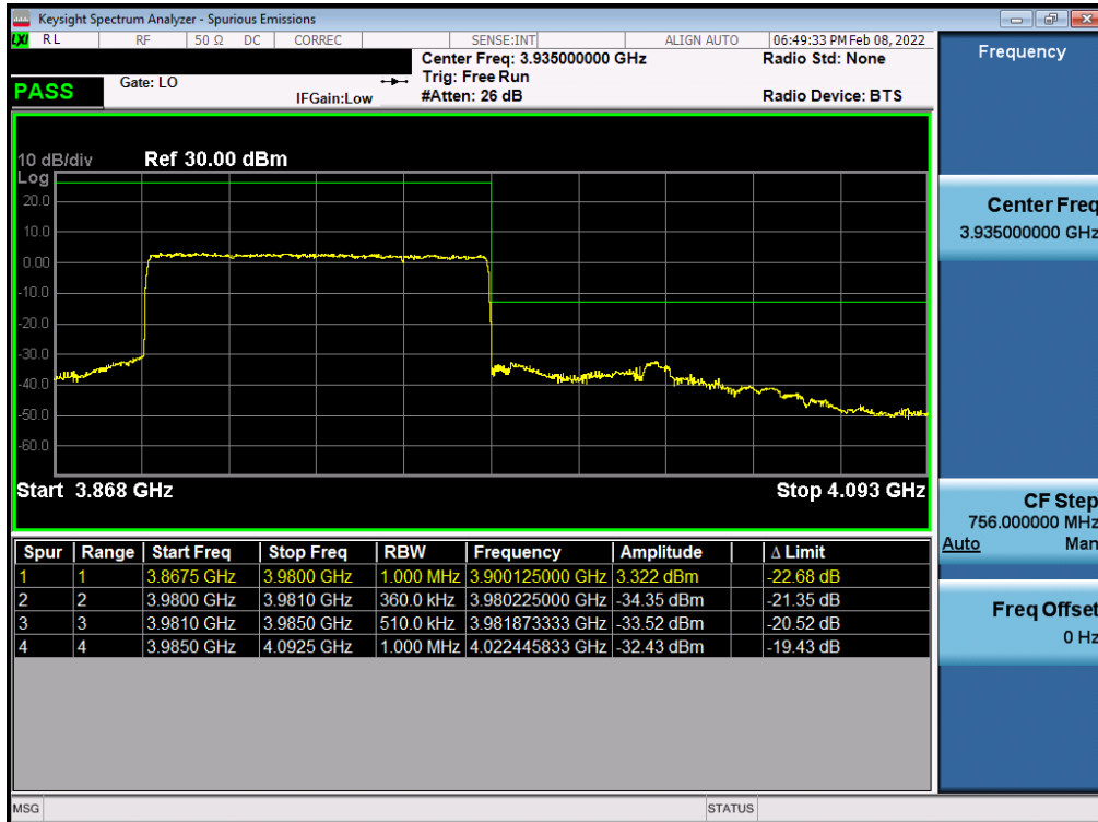
Plot 7-140. Upper ACP Plot (NR Band n77 - 90MHz CP-OFDM-QPSK – Full RB - Ant F)
