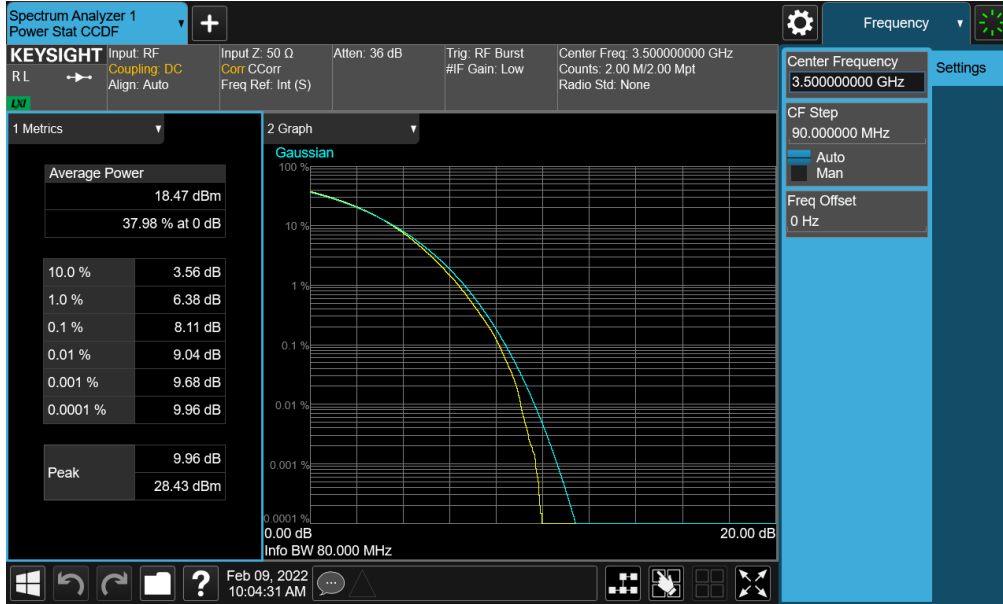
Plot 7-179. PAR Plot (NR Band n77 (DoD)- 80MHz CP-OFDM 256-QAM - Full RB - Ant F)
