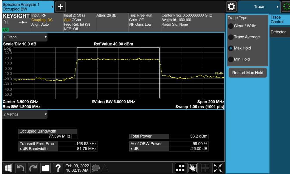
Plot 7-7. Occupied Bandwidth Plot (NR Band n77 - 80MHz \pi/2 BPSK - Full RB - Ant F)
