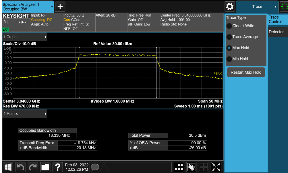
Plot 7-60. Occupied Bandwidth Plot (NR Band n77 - 20MHz 16-QAM - Full RB - Ant F)
