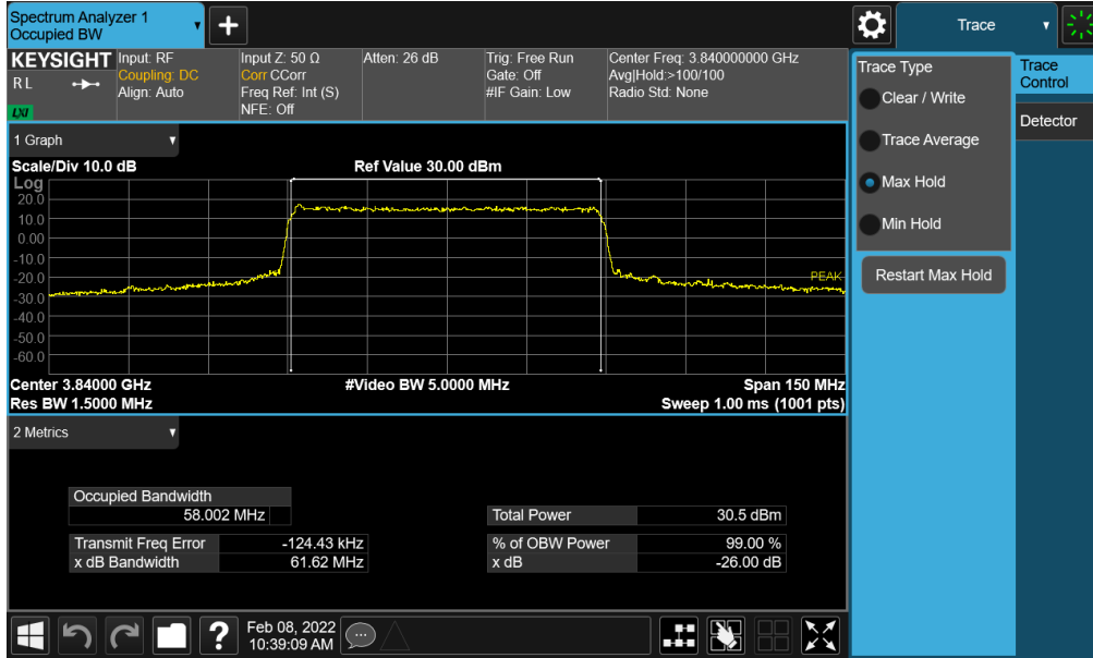
Plot 7-48. Occupied Bandwidth Plot (NR Band n77 - 60MHz 16-QAM - Full RB - Ant F)
