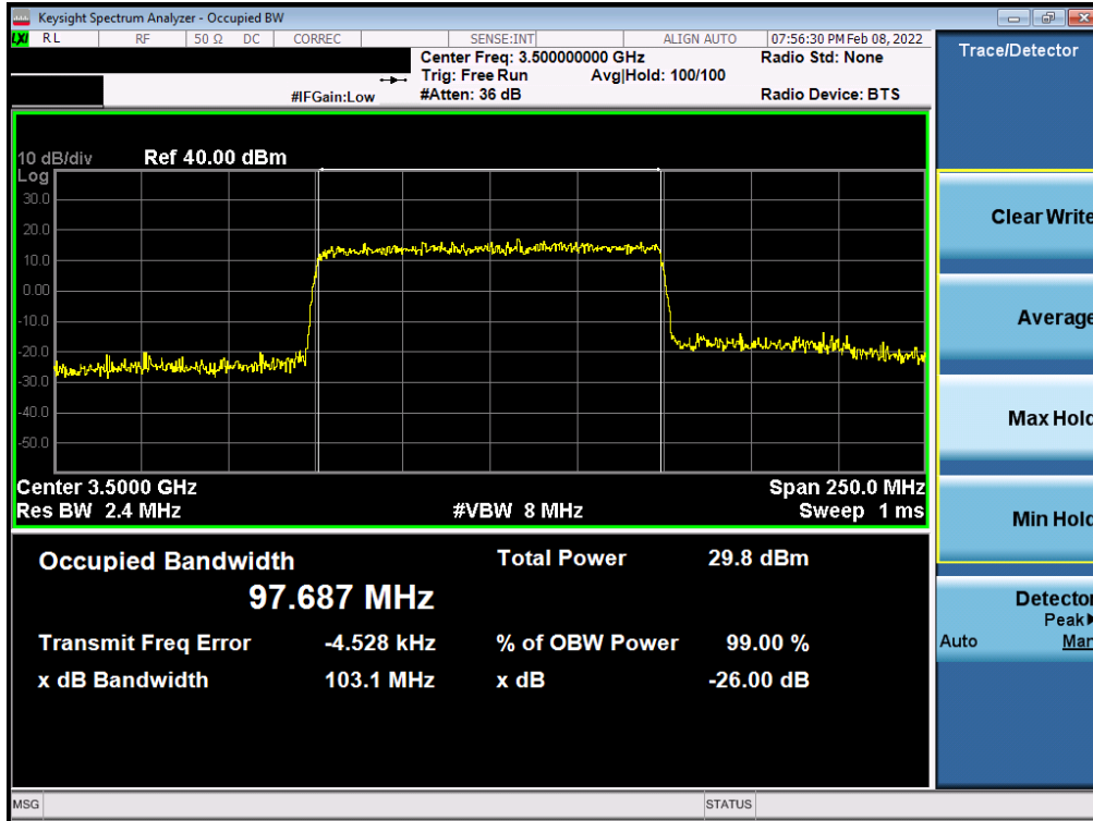
Plot 7-3. Occupied Bandwidth Plot (NR Band n77 - 100MHz 16-QAM - Full RB - Ant F)
