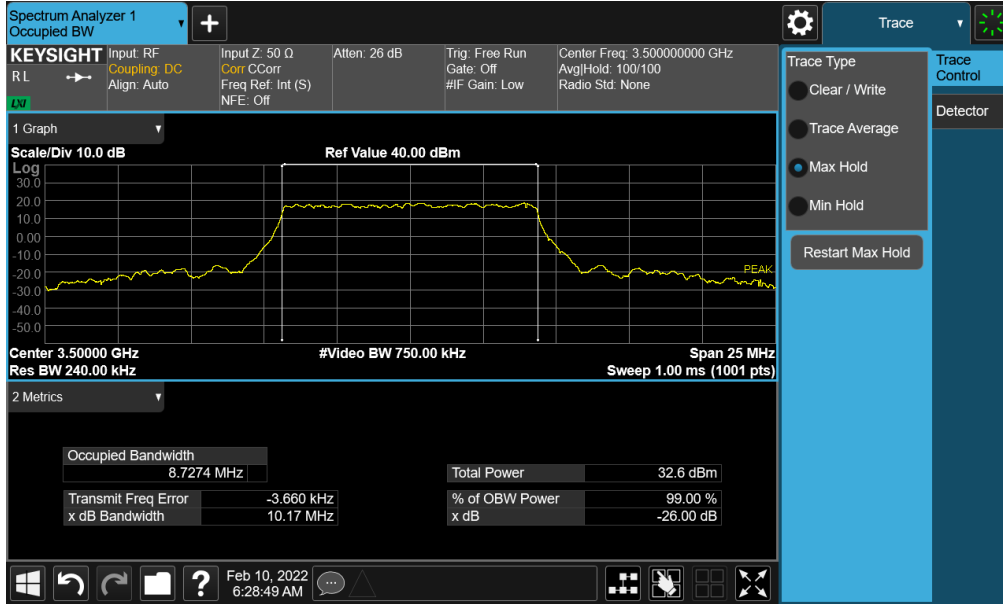
Plot 7-31. Occupied Bandwidth Plot (NR Band n77 - 10MHz \pi/2 BPSK - Full RB - Ant F)
