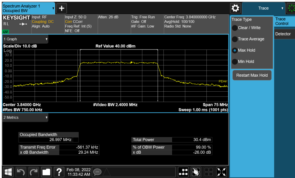
Plot 7-57. Occupied Bandwidth Plot (NR Band n77 - 30MHz 16-QAM - Full RB - Ant F)
