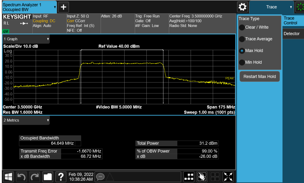
Plot 7-11. Occupied Bandwidth Plot (NR Band n77 - 70MHz QPSK - Full RB - Ant F)
