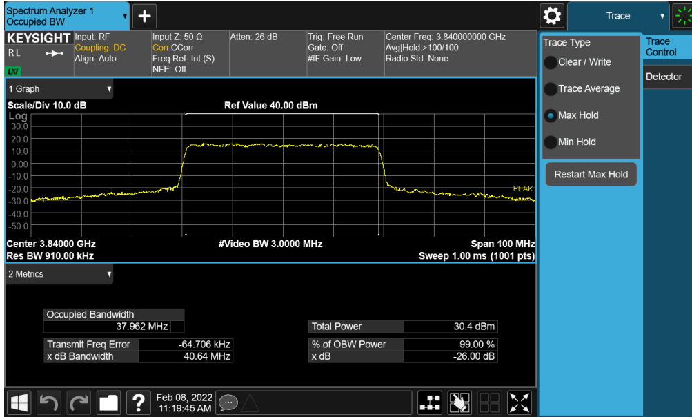
Plot 7-54. Occupied Bandwidth Plot (NR Band n77 - 40MHz 16-QAM - Full RB - Ant F)
