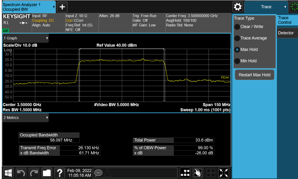
Plot 7-13. Occupied Bandwidth Plot (NR Band n77 - 60MHz \pi/2 BPSK - Full RB - Ant F)
