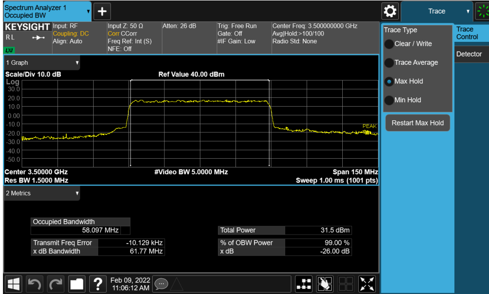
Plot 7-15. Occupied Bandwidth Plot (NR Band n77 - 60MHz 16-QAM - Full RB - Ant F)
