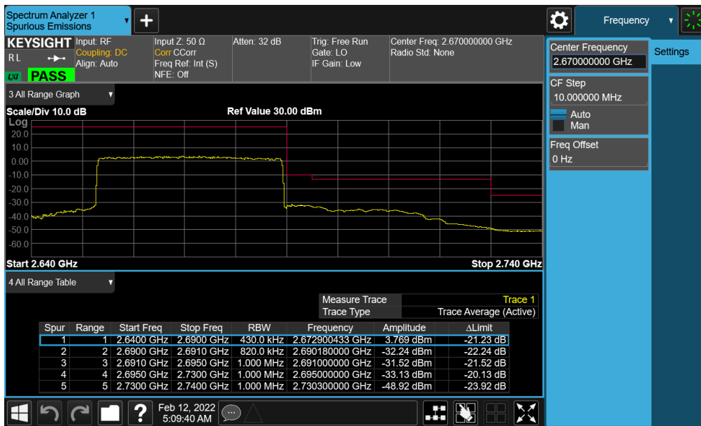
Plot 7-72. Upper ACP Plot (NR Band n41 - 40MHz CP-OFDM-QPSK – Full RB - Ant I)
