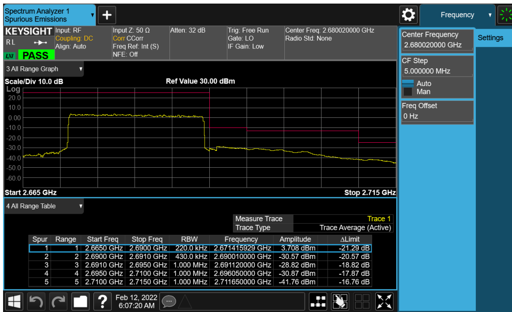
Plot 7-74. Upper ACP Plot (NR Band n41 - 20MHz CP-OFDM-QPSK – Full RB - Ant I)
