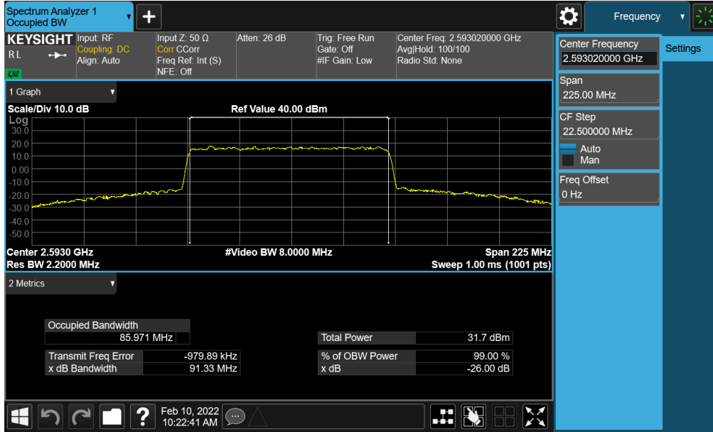
Plot 7-5. Occupied Bandwidth Plot (NR Band n41 - 90MHz QPSK - Full RB - Ant I)
