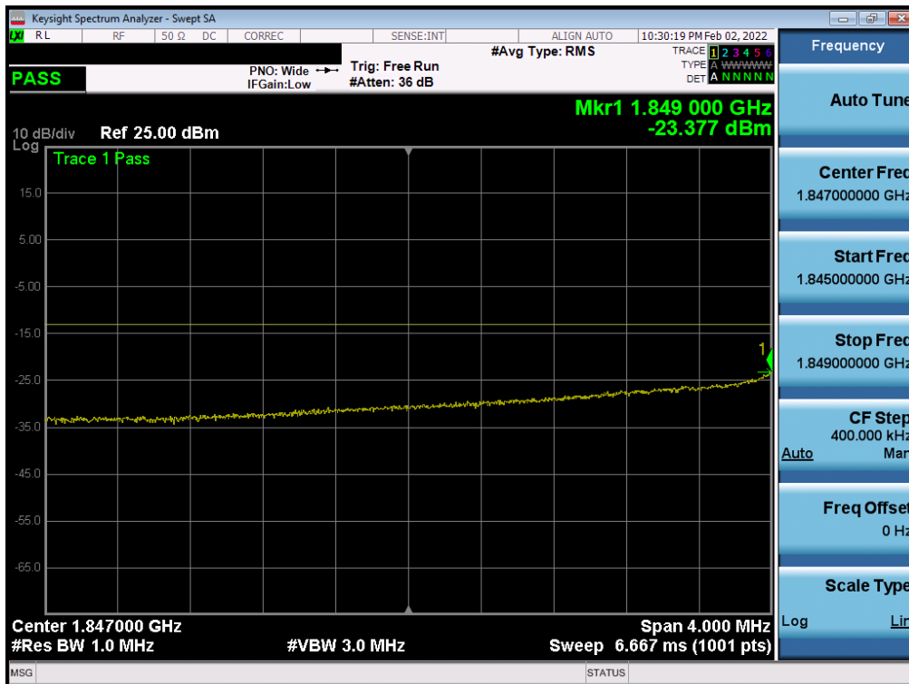
Plot 7-23. Extended Lower Band Edge Plot (NR Band n25/2 - 20MHz QPSK – Full RB)
