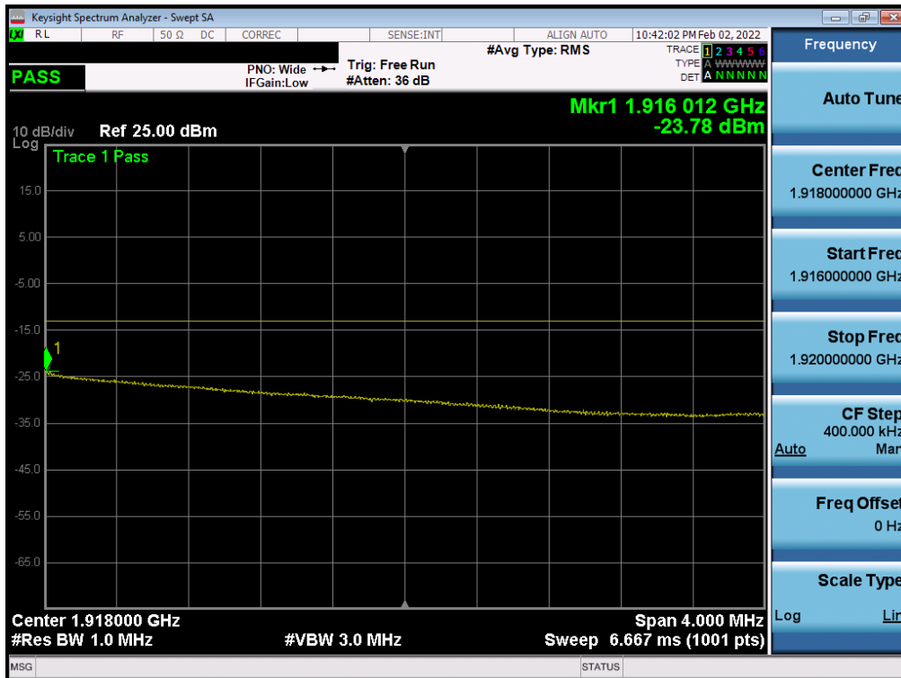
Plot 7-27. Extended Upper Band Edge Plot (NR Band n25 - 20MHz QPSK – Full RB)
