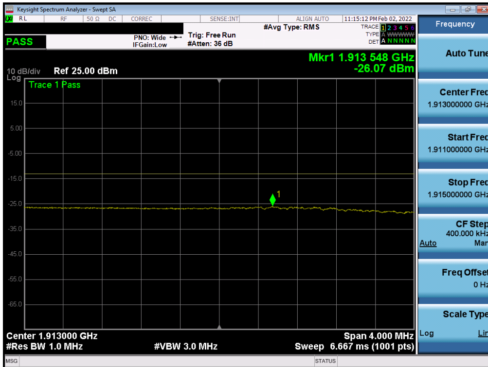
Plot 7-31. Extended Upper Band Edge Plot (NR Band n2 - 15MHz QPSK – Full RB)
