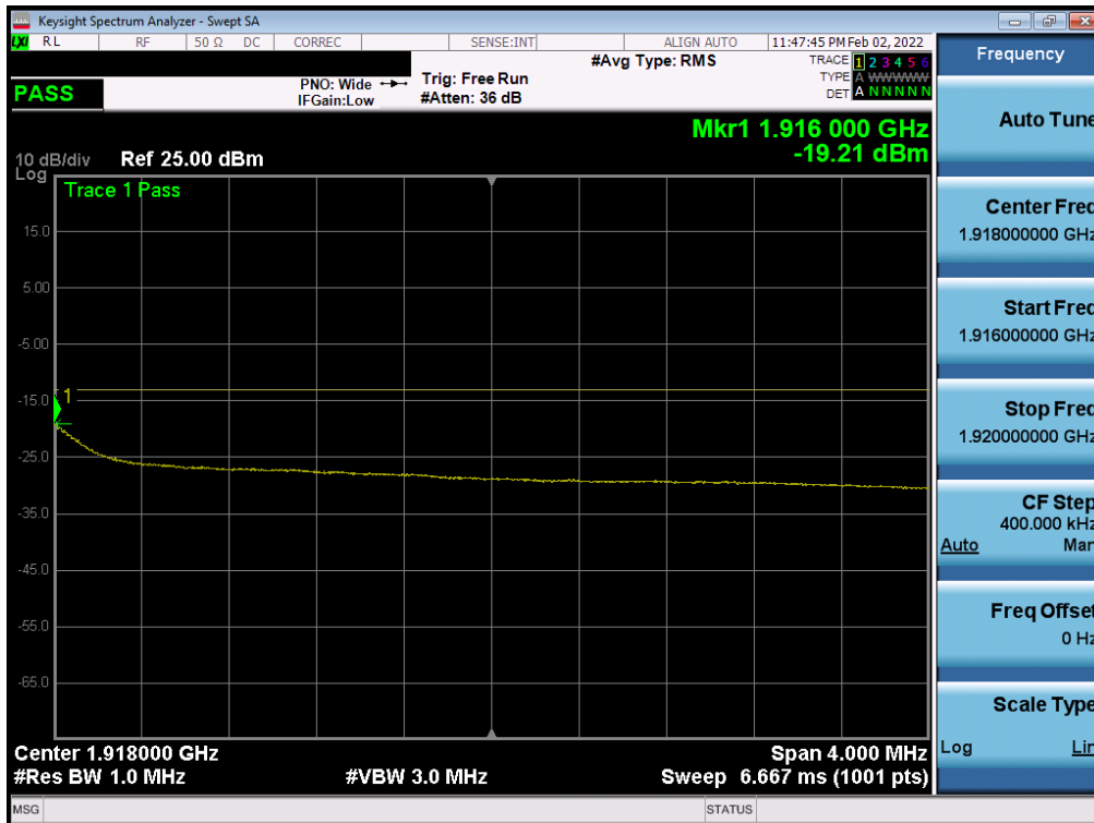
Plot 7-39. Extended Upper Band Edge Plot (NR Band n25 - 10MHz QPSK – Full RB)
