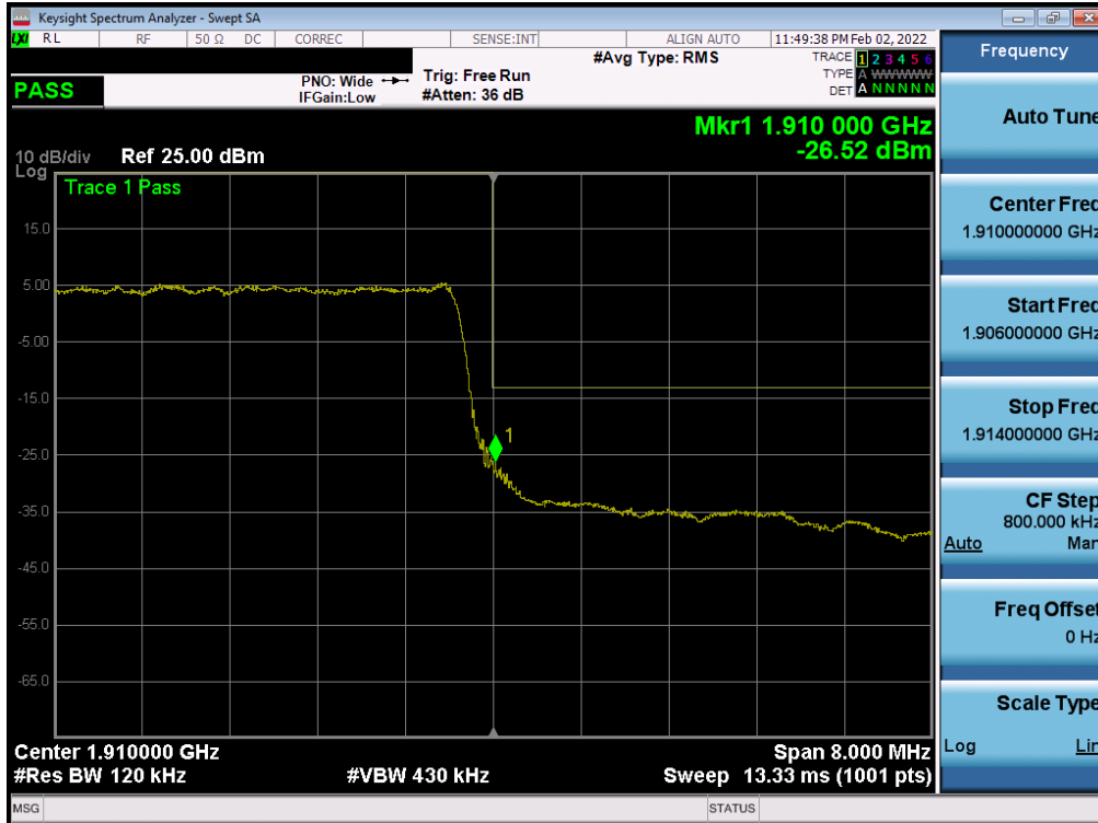
Plot 7-36. Upper Band Edge Plot (NR Band n2 - 10MHz QPSK – Full RB)
