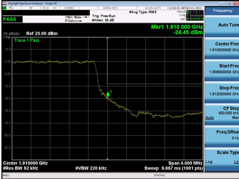
Plot 7-42. Upper Band Edge Plot (NR Band n2 – 5MHz QPSK – Full RB)
