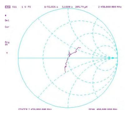
Impedance & Return-Loss Measurement Plot for Head TSL
