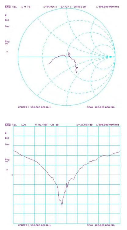
Impedance & Return-Loss Measurement Plot for Head TSL
