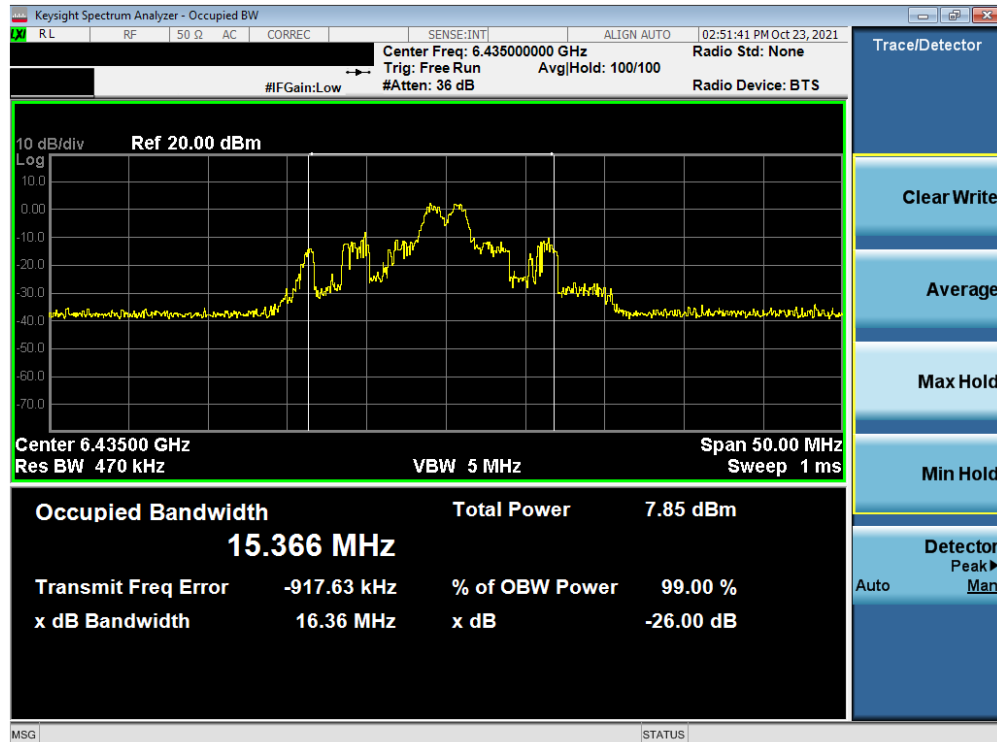
Plot 7-96. 26dB Bandwidth Plot MIMO ANT2 (20MHz BW 802.11ax (26 Tones) (UNII Band 6) – Ch. 97)
