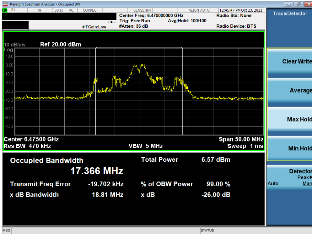
Plot 7-17. 26dB Bandwidth Plot MIMO ANT1 (20MHz BW 802.11ax (26 Tones) (UNII Band 6) – Ch. 105)
