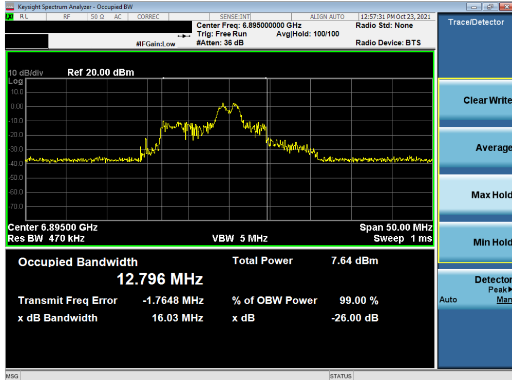
Plot 7-38. 26dB Bandwidth Plot MIMO ANT1 (20MHz BW 802.11ax (26 Tones) (UNII Band 8) – Ch. 189)
