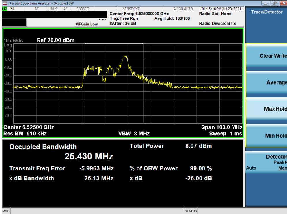
Plot 7-21. 26dB Bandwidth Plot MIMO ANT1 (40MHz BW 802.11ax (26 Tones) (UNII Band 6) – Ch. 115)
