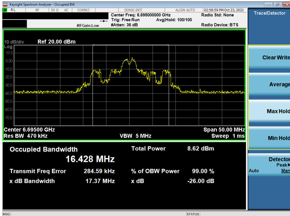
Plot 7-106. 26dB Bandwidth Plot MIMO ANT2 (20MHz BW 802.11ax (26 Tones) (UNII Band 7) – Ch. 149)
