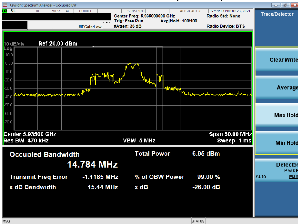
Plot 7-81. 26dB Bandwidth Plot MIMO ANT2 (20MHz BW 802.11ax (26 Tones) UNII Band 5) – Ch. 2)
