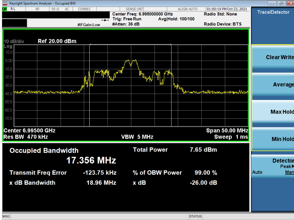
Plot 7-39. 26dB Bandwidth Plot MIMO ANT1 (20MHz BW 802.11ax (26 Tones) (UNII Band 8) – Ch. 209)
