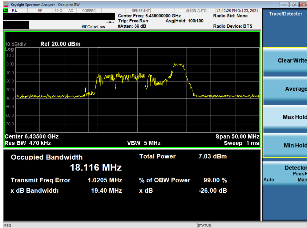
Plot 7-16. 26dB Bandwidth Plot MIMO ANT1 (20MHz BW 802.11ax (26 Tones) (UNII Band 6) – Ch. 97)
