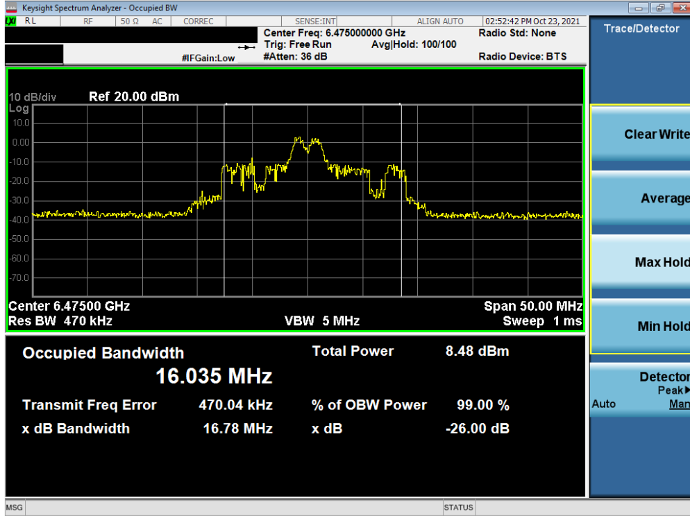
Plot 7-97. 26dB Bandwidth Plot MIMO ANT2 (20MHz BW 802.11ax (26 Tones) (UNII Band 6) – Ch. 105)
