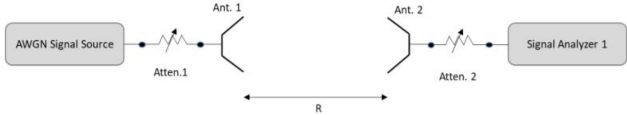
Figure 7-5. Contention-based protocol test setup, radiated method, power measurement
