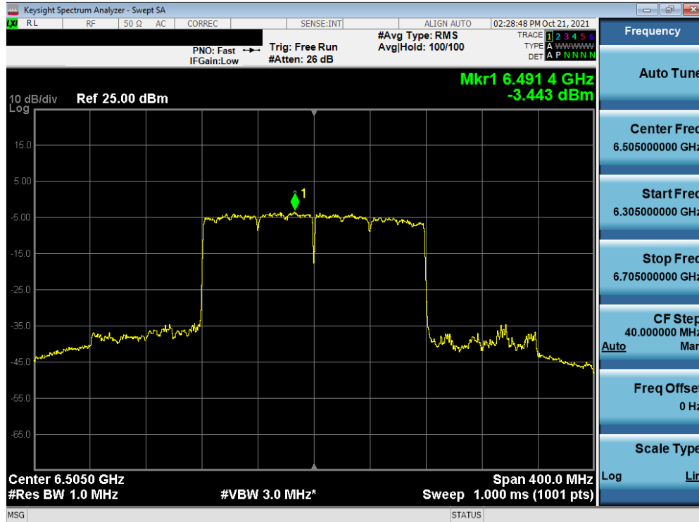
Plot 7-182. Power Spectral Density Measurement Plot MIMO ANT2 (160MHz 802.11ax (UNII Band 6) – Ch. 111)
