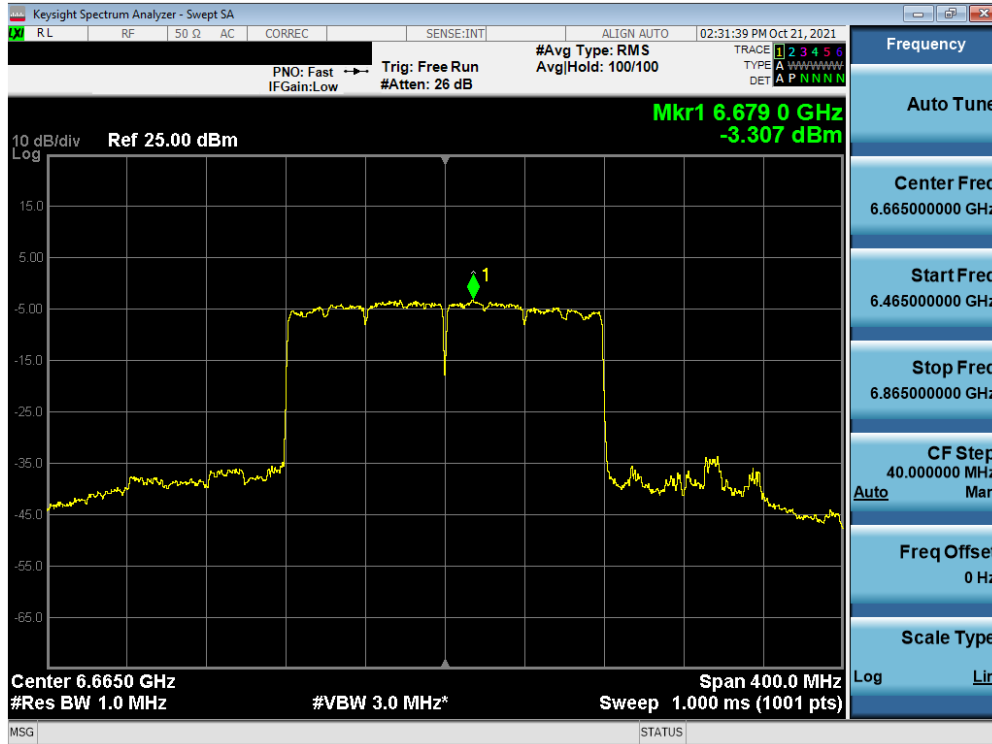
Plot 7-195. Power Spectral Density Measurement Plot MIMO ANT2 (160MHz 802.11ax (UNII Band 7) – Ch. 143)
