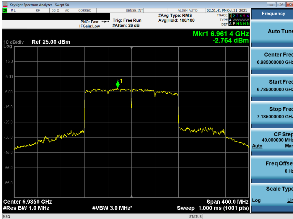
Plot 7-208. Power Spectral Density Measurement Plot MIMO ANT2 (160MHz 802.11ax (UNII Band 8) – Ch. 207)
