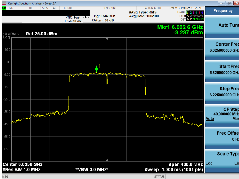
Plot 7-169. Power Spectral Density Measurement Plot MIMO ANT2 (160MHz 802.11 ax (UNII Band 5) – Ch. 15)
