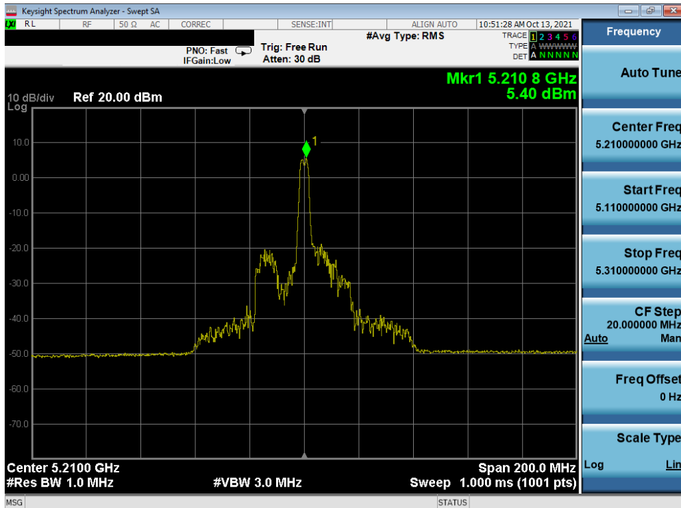
Plot 7-240. Power Spectral Density Plot MIMO ANT2 (80MHz BW 802.11ax – 26 Tones (UNII Band 1) – Ch. 42)
