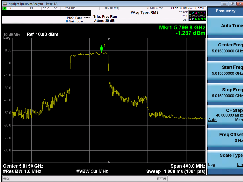
Plot 7-233. Power Spectral Density Plot MIMO ANT1 (160MHz BW (L) 802.11ax – Full Tones (UNII Band 3/4) – Ch. 163)
