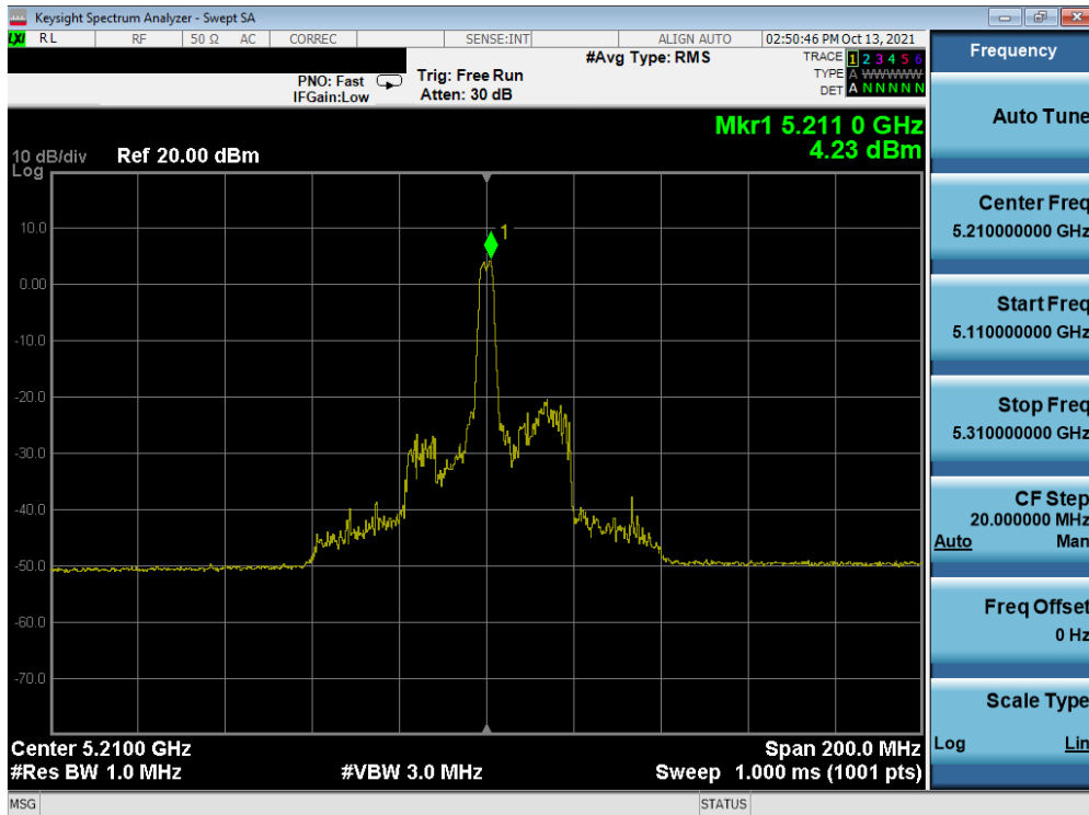
Plot 7-162. Power Spectral Density Plot MIMO ANT1 (80MHz BW 802.11ax – 26 Tones (UNII Band 1) – Ch. 42)
