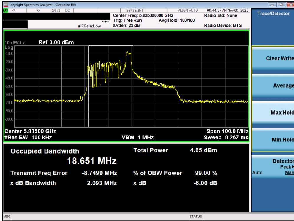
Plot 7-110. 6dB Bandwidth Plot MIMO ANT1 (40MHz BW 802.11ax – 26 Tones (UNII Band 3/4) – Ch. 167)
