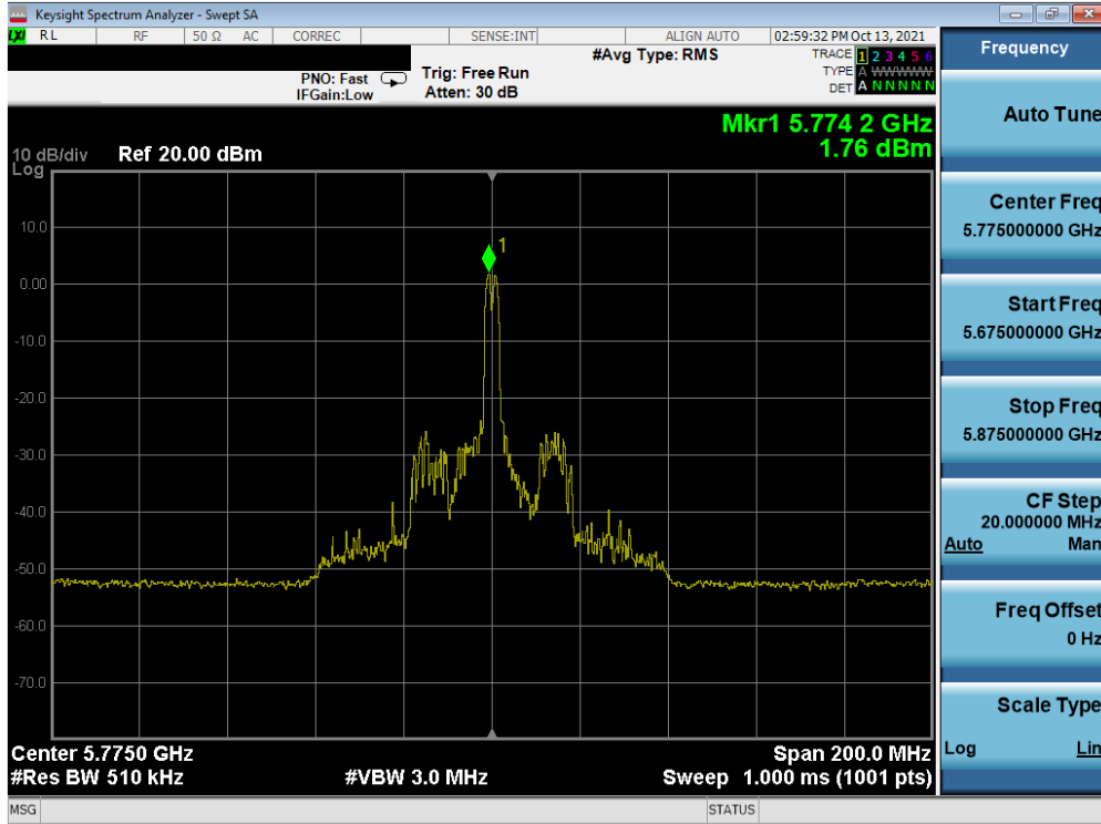
Plot 7-187. Power Spectral Density Plot MIMO ANT1 (80MHz BW 802.11ax – 26 Tones (UNII Band 3) – Ch. 155)
