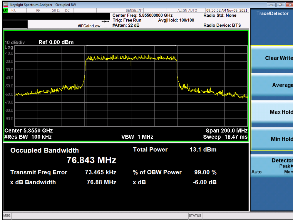
Plot 7-126. 6dB Bandwidth Plot MIMO ANT1 (80MHz BW 802.11ax – 996 Tones (UNII Band 3/4) – Ch. 171)
