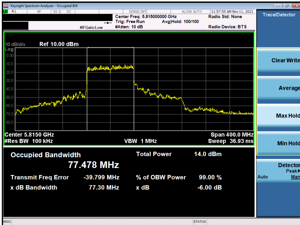
Plot 7-127. 6dB Bandwidth Plot MIMO ANT1 (160MHz BW (L) 802.11ax – 996 Tones (UNII Band 3/4) – Ch. 163)
