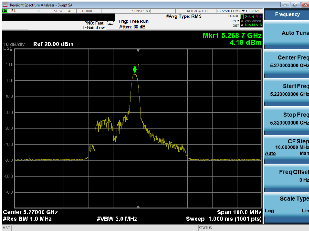
Plot 7-168. Power Spectral Density Plot MIMO ANT1 (40MHz BW 802.11ax – 26 Tones (UNII Band 2A) – Ch. 54)
