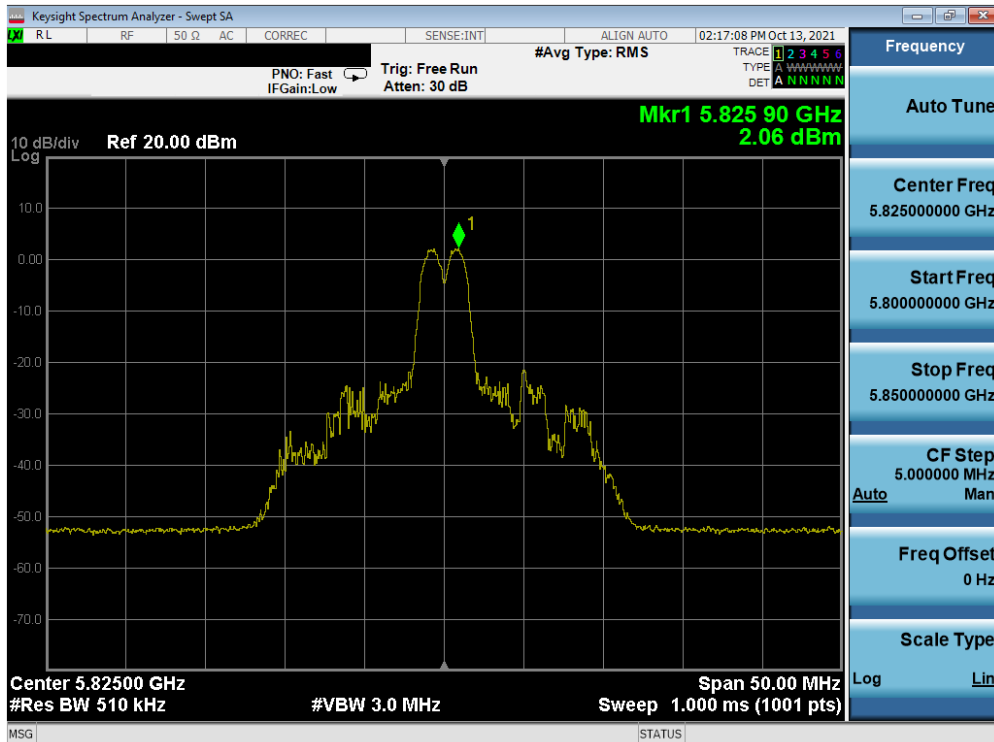
Plot 7-184. Power Spectral Density Plot MIMO ANT1 (20MHz BW 802.11ax – 26 Tones (UNII Band 3) – Ch. 165)
