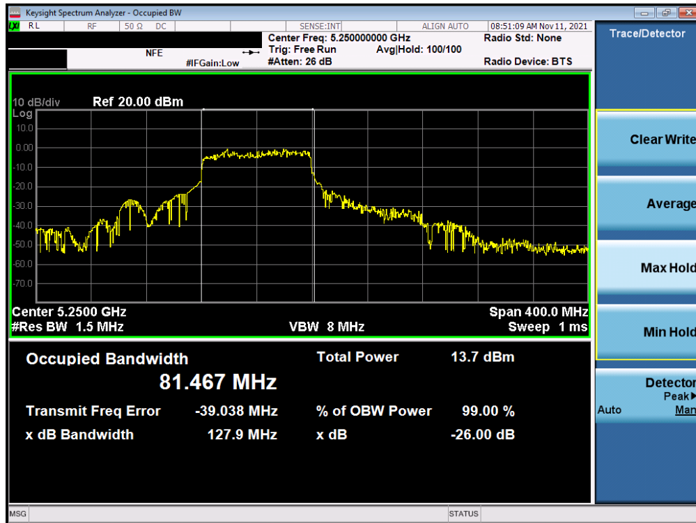
Plot 7-82. 26dB Bandwidth Plot MIMO ANT2 (160MHz BW (L) 802.11ax – 996 Tones (UNII Band 1/2A) – Ch. 50)
