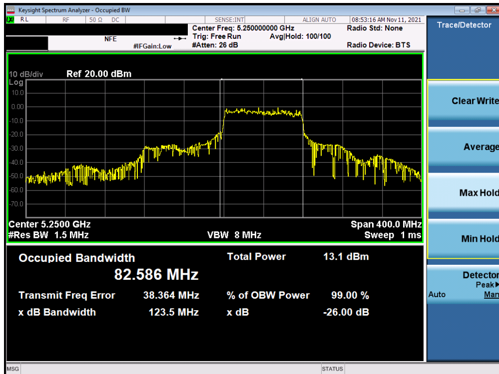
Plot 7-83. 26dB Bandwidth Plot MIMO ANT2 (160MHz BW (U) 802.11ax – 996 Tones (UNII Band 1/2A) – Ch. 50)
