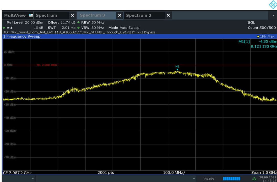
Plot 7-65. UWB Peak Power Measurement - ANT 2 - CH.9 – BPRF
