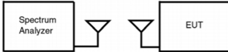
Figure 7-2. Test Instrument and Measurement Setup
