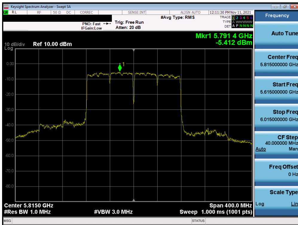
Plot 7-347. Power Spectral Density Plot MIMO ANT2 (160MHz BW 802.11ac (UNII Band 3/4) – Ch. 163)
