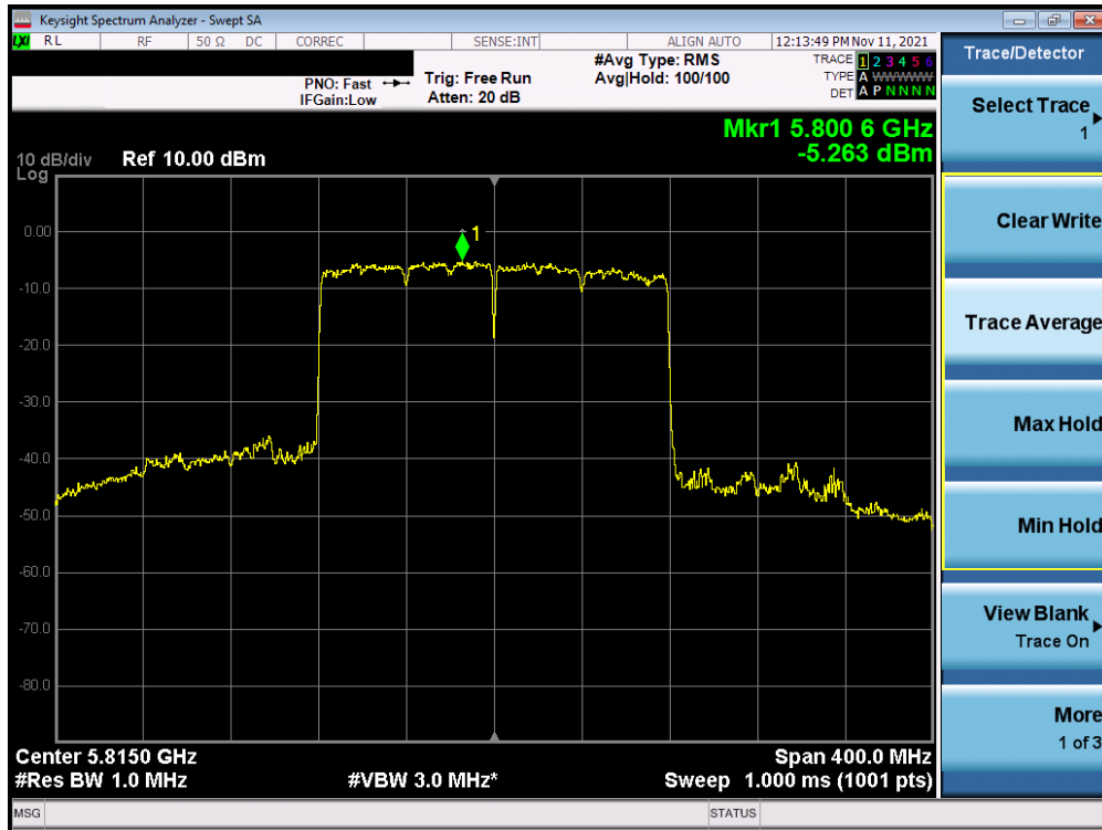
Plot 7-348. Power Spectral Density Plot MIMO ANT2 (160MHz BW 802.11ax (UNII Band 3/4) – Ch. 163)
