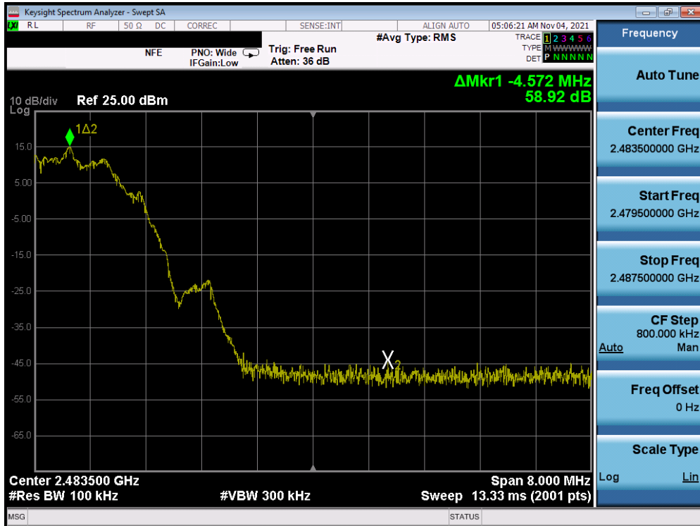
Plot 7-124. Band Edge Plot (Bluetooth (LE), 2Mbps, – Ch. 39) Antenna 2
