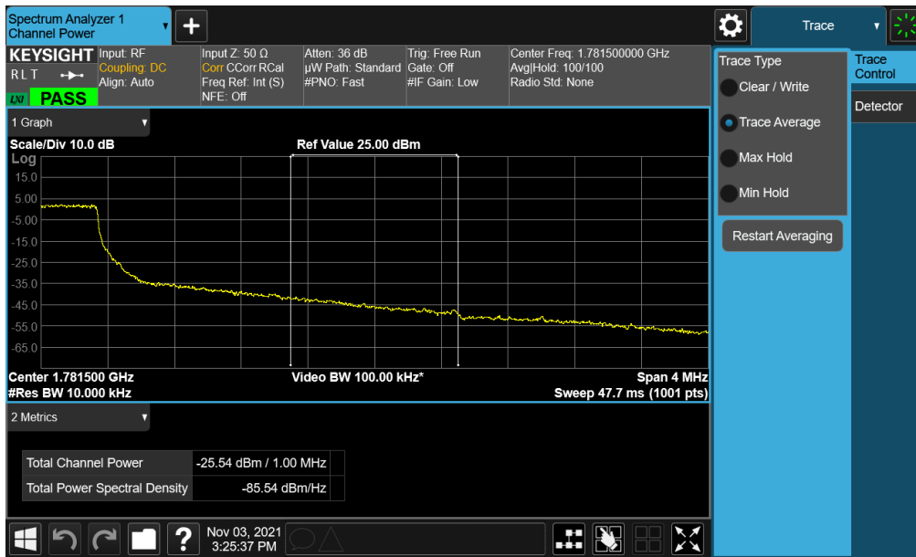
Plot 7-113. Upper Extended Band Edge Plot (LTE Band 66 – 1.4MHz QPSK – Full RB)
