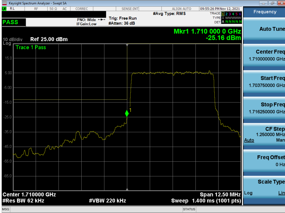
Plot 7-37. Lower Band Edge Plot (NR Band n66 – 5.0MHz - Full RB – ANT1)
