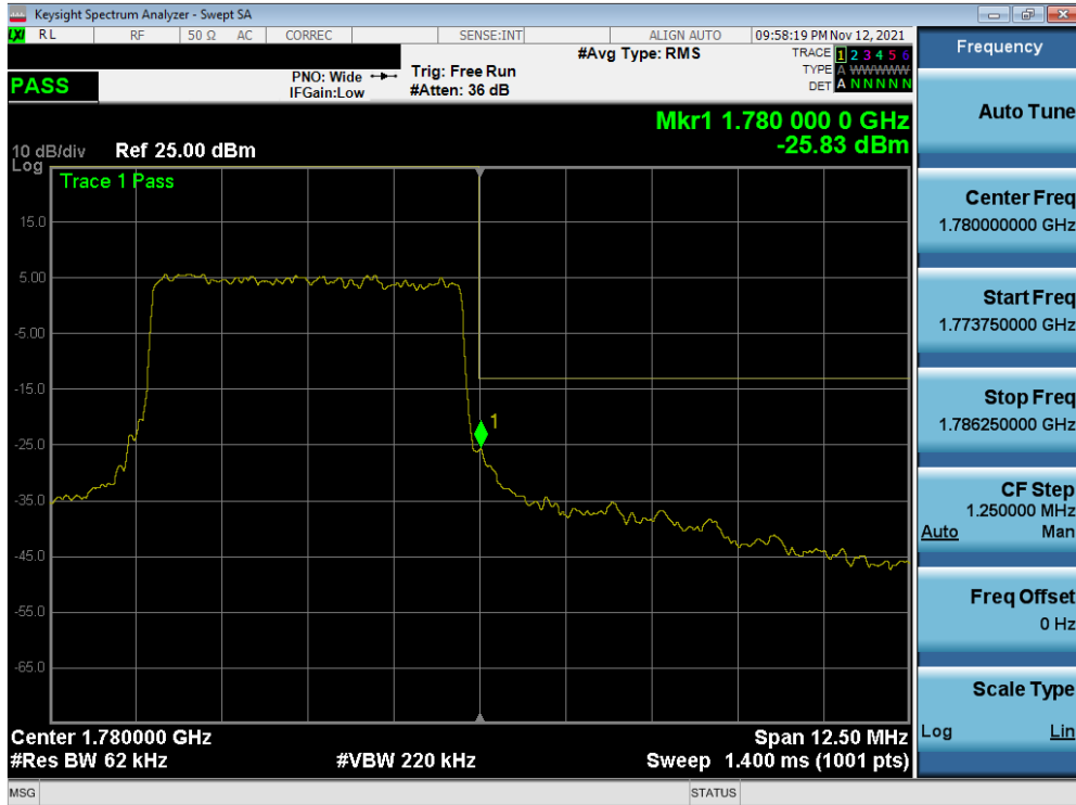
Plot 7-39. Upper Band Edge Plot (NR Band n66 – 5.0MHz - Full RB – ANT1)
