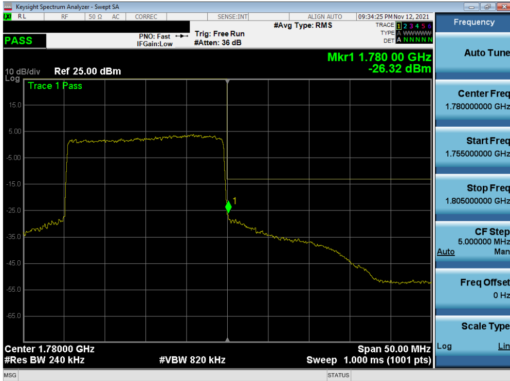
Plot 7-27. Upper Band Edge Plot (NR Band n66 – 20.0MHz - Full RB – ANT1)
