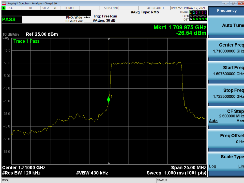
Plot 7-33. Lower Band Edge Plot (NR Band n66 – 10.0MHz - Full RB – ANT1)
