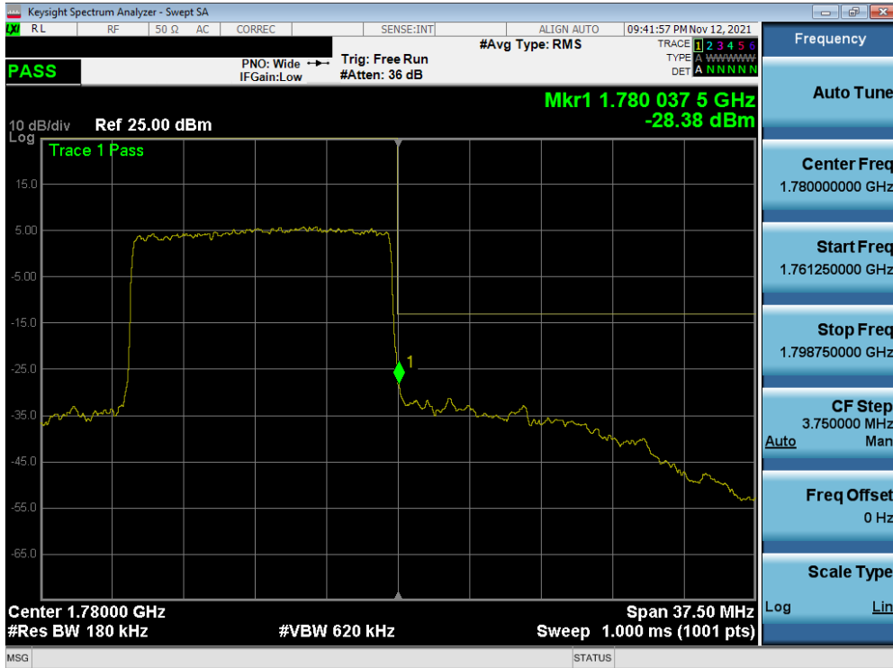
Plot 7-31. Upper Band Edge Plot (NR Band n66 – 15.0MHz - Full RB – ANT1)
