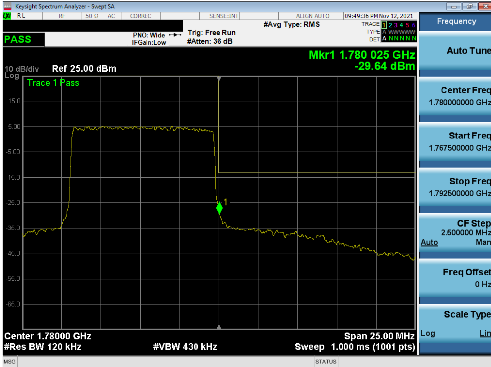
Plot 7-35. Upper Band Edge Plot (NR Band n66 – 10.0MHz - Full RB – ANT1)
