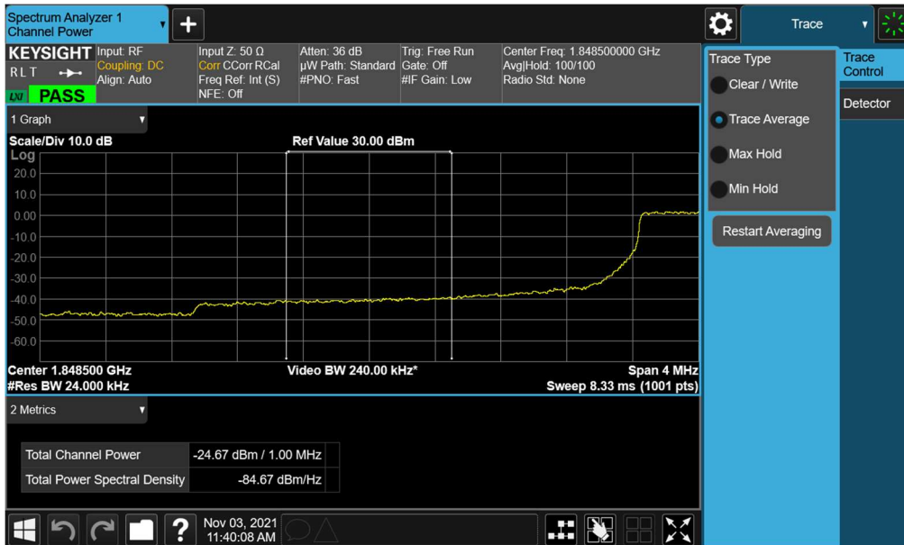
Plot 7-68. Extended Lower Band Edge Plot (LTE Band 25/2 - 3MHz QPSK – Full RB)
