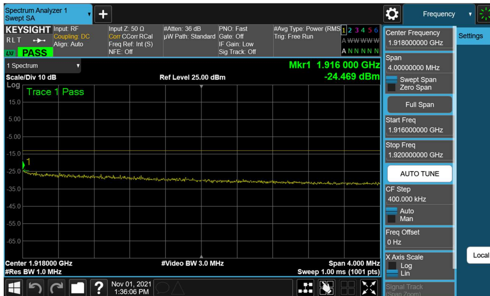
Plot 7-60. Extended Upper Band Edge Plot (LTE Band 25 - 10MHz QPSK – Full RB)
