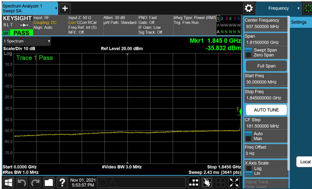
Plot 7-34. Conducted Spurious Plot (WCDMA Ch. 9262)
