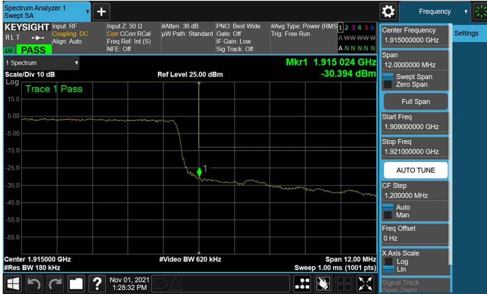
Plot 7-53. Upper Band Edge Plot (LTE Band 25 - 15MHz QPSK – Full RB)
