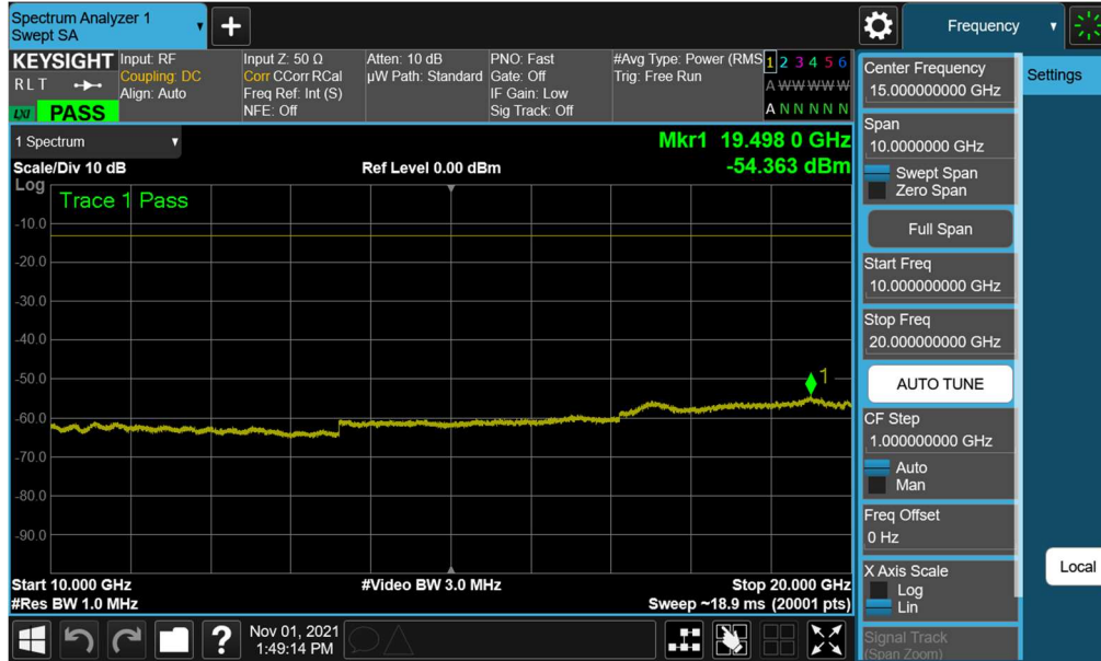
Plot 7-18. Conducted Spurious Plot (LTE Band 25/2 - 20MHz QPSK - 1RB - Low Channel)
