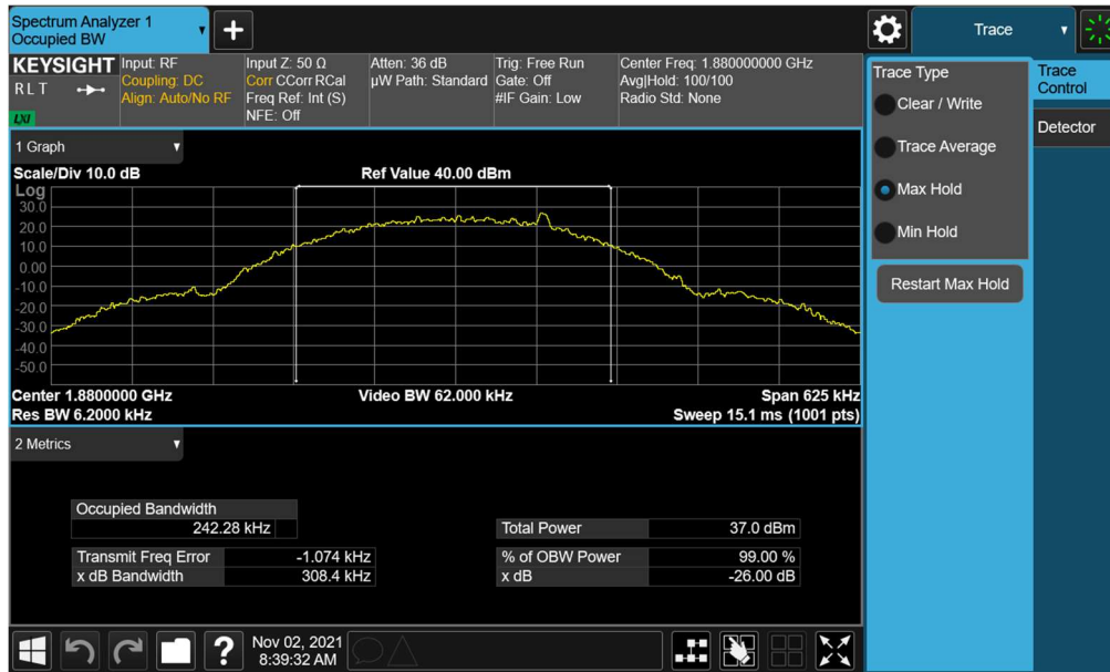
Plot 7-13. Occupied Bandwidth Plot (GPRS, Ch. 661)
