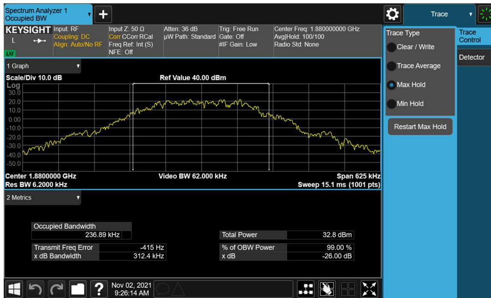
Plot 7-14. Occupied Bandwidth Plot (EDGE, Ch. 661)
