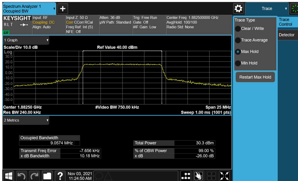
Plot 7-6. Occupied Bandwidth Plot (LTE Band 25/2 - 10MHz 16-QAM - Full RB)
