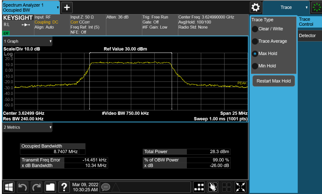
Plot 7-11. Occupied Bandwidth Plot (NR Band n48 - 10MHz QPSK - Full RB Configuration)
