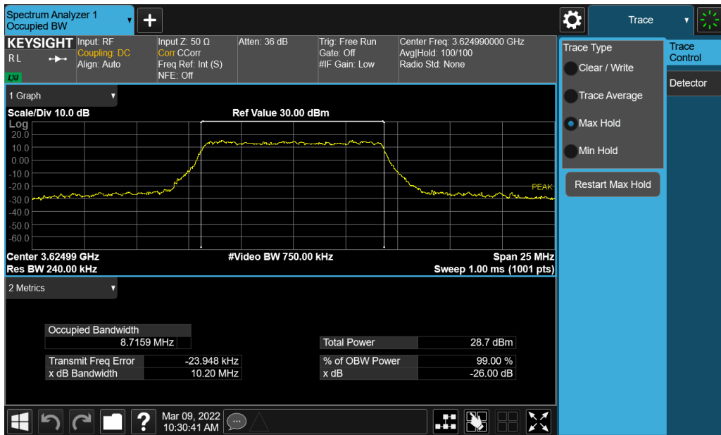
Plot 7-12. Occupied Bandwidth Plot (NR Band n48 - 10MHz 16-QAM - Full RB Configuration)
