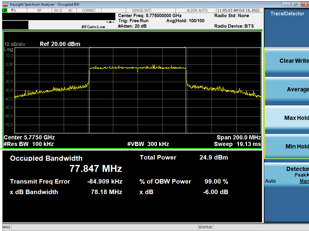
Plot 7-102. 6dB Bandwidth Plot SISO ANT1 (80MHz BW 802.11ax – 996 Tones (UNII Band 3) – Ch. 155)
