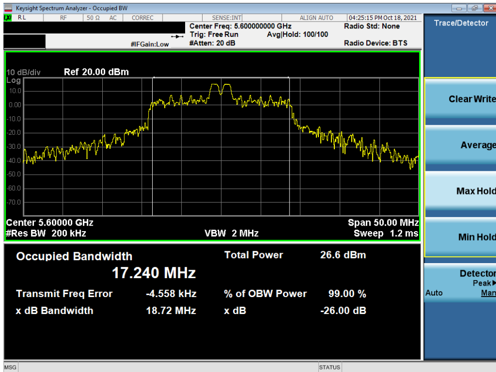
Plot 7-56. 26dB Bandwidth Plot SISO ANT2 (20MHz BW 802.11ax – 26 Tones (UNII Band 2C) – Ch. 120)
