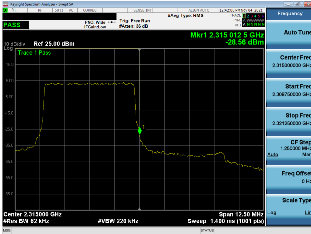
Plot 7-288. Upper Band Edge Plot (LTE Band 30 - 5MHz QPSK – Full RB – Ant A)
