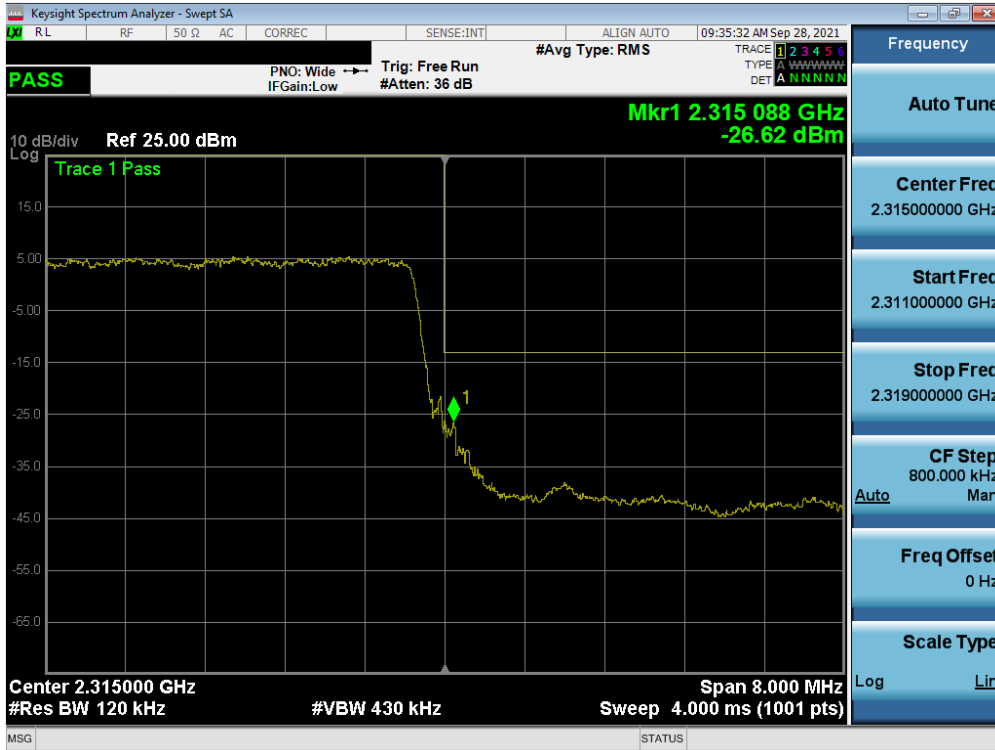
Plot 7-301. Upper Band Edge Plot (NR Band n30 - 10MHz CP-OFDM-QPSK – Full RB – Ant F)
