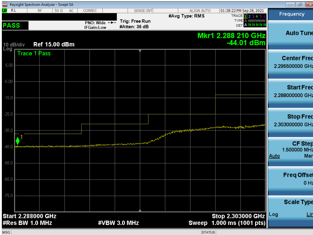
Plot 7-295. Extended Lower Band Edge Plot (NR Band n30 - 5MHz CP-OFDM-QPSK – Full RB – Ant A)
