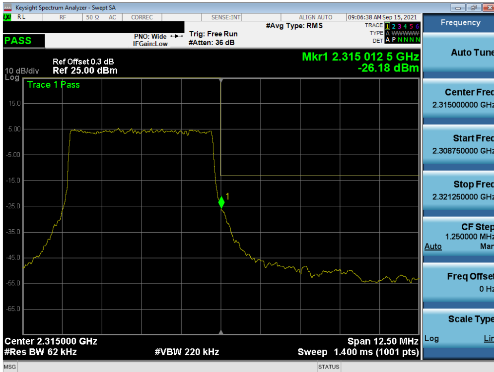
Plot 7-240. Upper Band Edge Plot (NR Band n30 - 5MHz CP-OFDM-QPSK – Full RB – Ant B)
