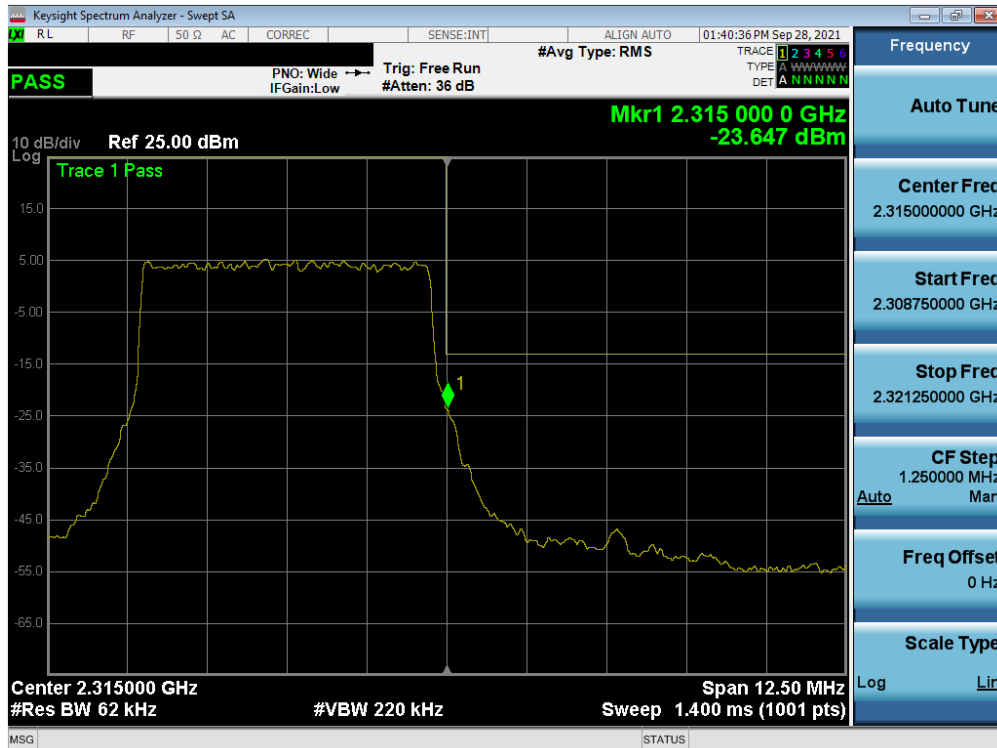
Plot 7-297. Upper Band Edge Plot (NR Band n30 - 5MHz CP-OFDM-QPSK – Full RB – Ant A)
