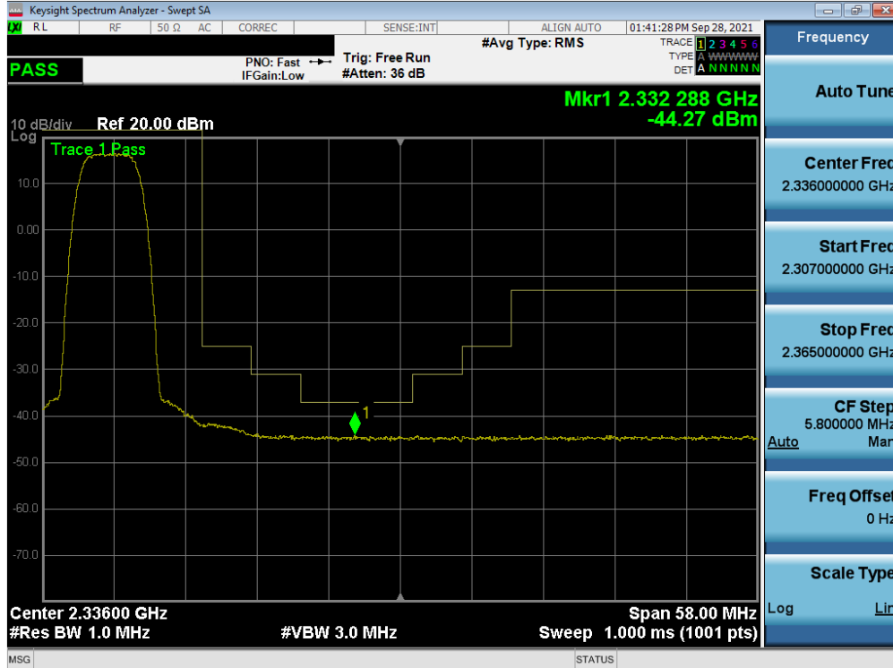
Plot 7-298. Extended Upper Band Edge Plot (NR Band n30 - 5MHz CP-OFDM-QPSK – Full RB – Ant A)
