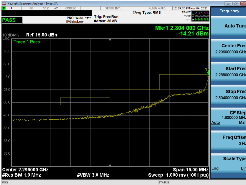
Plot 7-287. Extended Lower Band Edge Plot (LTE Band 30 - 5MHz QPSK – Full RB – Ant A)
