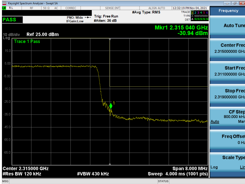
Plot 7-284. Upper Band Edge Plot (LTE Band 30 - 10MHz QPSK – Full RB – Ant A)
