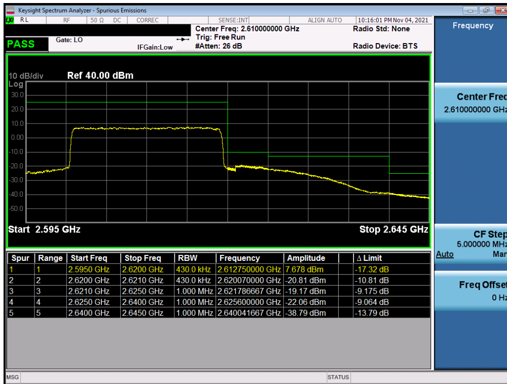
Plot 7-277. Upper Band Edge Plot (NR Band n38 - 20MHz CP-OFDM-QPSK – Full RB - Ant F)
