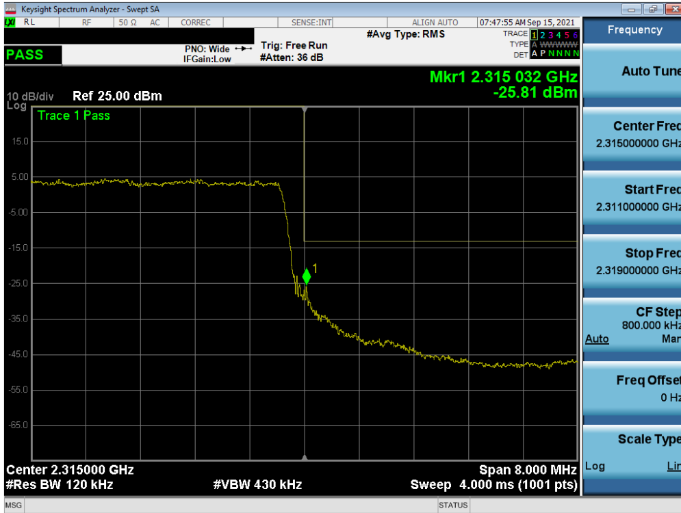
Plot 7-235. Upper Band Edge Plot (NR Band n30 - 10MHz CP-OFDM-QPSK – Full RB – Ant B)
