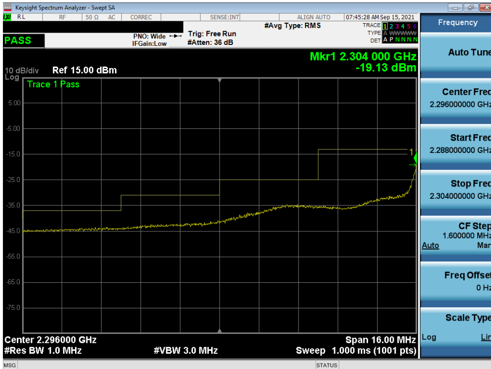
Plot 7-234. Extended Lower Band Edge Plot (NR Band n30 - 10MHz CP-OFDM-QPSK – Full RB – Ant B)
