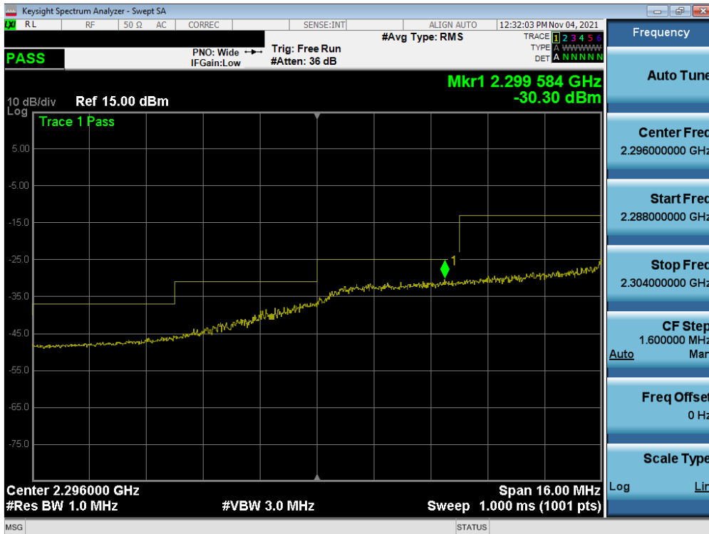
Plot 7-283. Extended Lower Band Edge Plot (LTE Band 30 - 10MHz QPSK – Full RB – Ant A)
