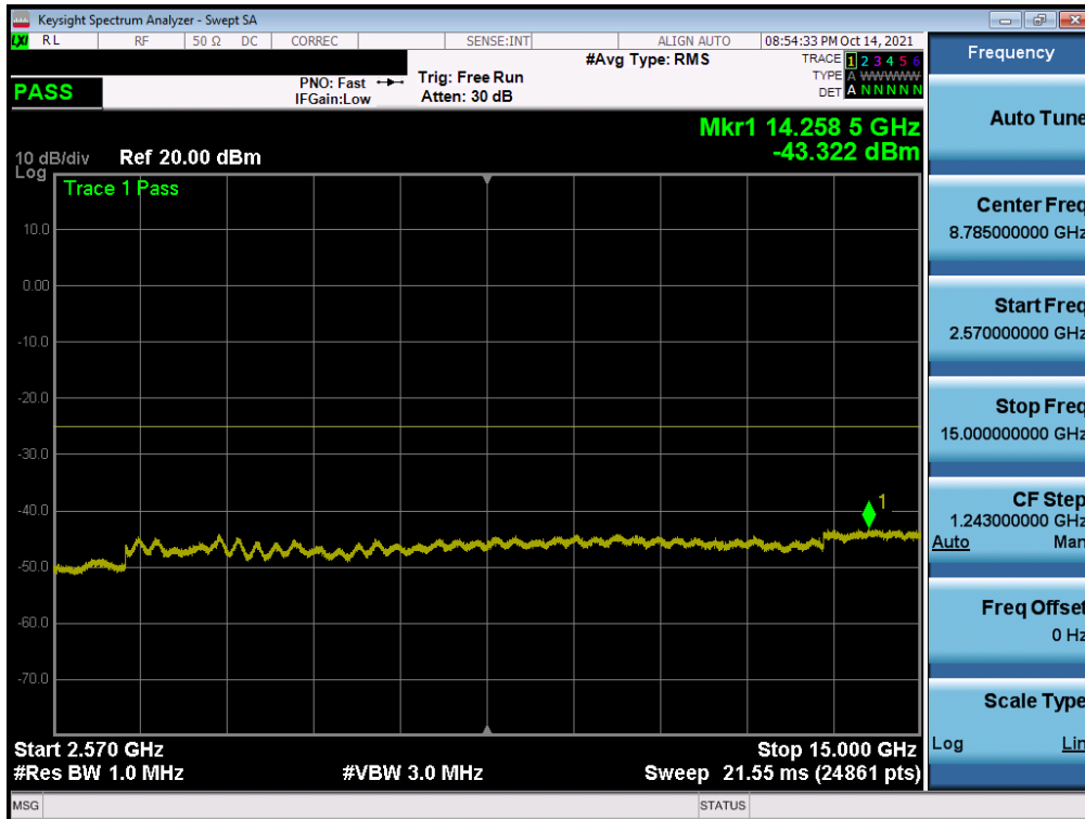
Plot 7-133. Conducted Spurious Plot (NR Band n7 – 40MHz QPSK – RB Size 1, RB Offset 0 – Low Channel Ant B)
