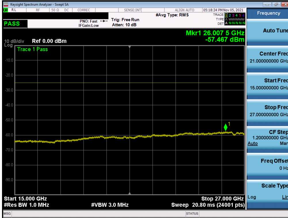
Plot 7-140. Conducted Spurious Plot (NR Band n7 – 40MHz QPSK – RB Size 1, RB Offset 0 – High Channel Ant B)
