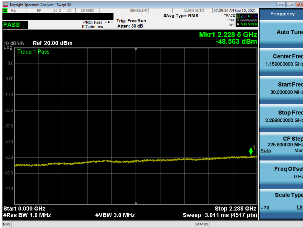
Plot 7-129. Conducted Spurious Plot (NR Band n30 – 10MHz QPSK – RB Size 1, RB Offset 0 – Ant B)
