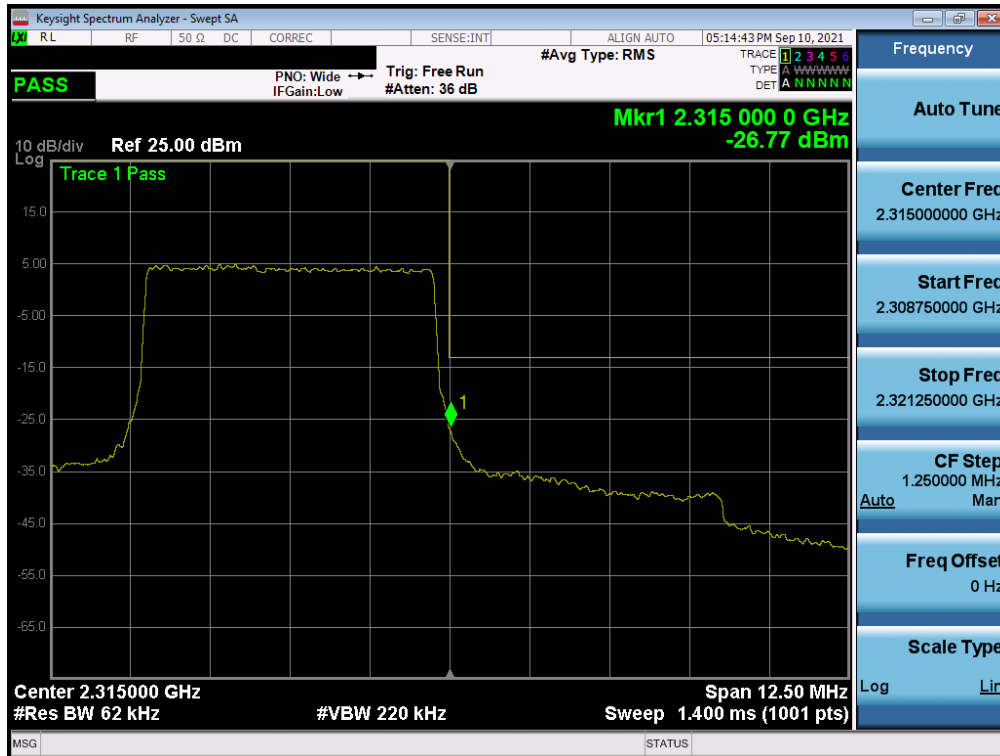
Plot 7-199. Upper Band Edge Plot (LTE Band 30 - 5MHz QPSK – Full RB – Ant B)
