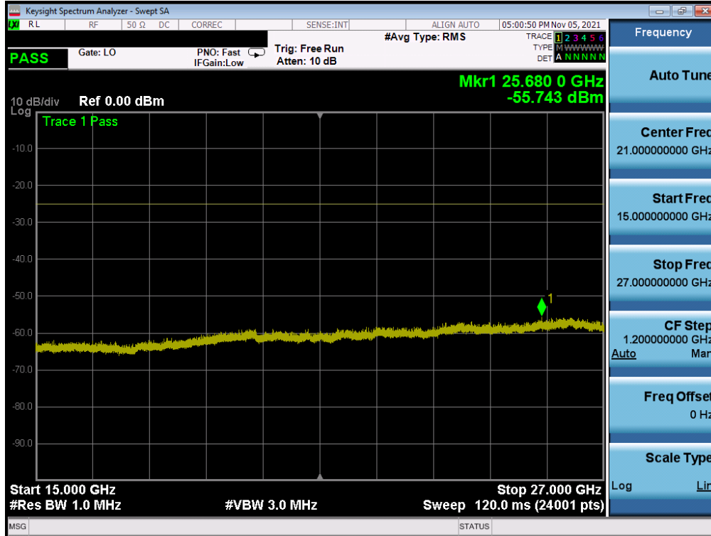
Plot 7-128. Conducted Spurious Plot (LTE Band 41(PC3)/38 – 20MHz QPSK – RB Size 1, RB Offset 0 – High Channel)
