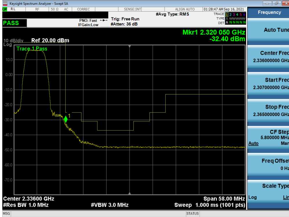
Plot 7-200. Extended Upper Band Edge Plot (LTE Band 30 - 5MHz QPSK – Full RB – Ant B)
