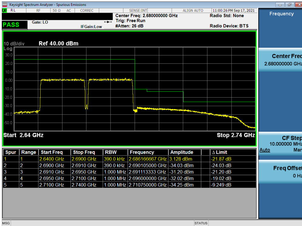
Plot 7-188. Upper ACP Plot (ULCA LTE B41(PC3) - 20MHz QPSK - Full RB)
