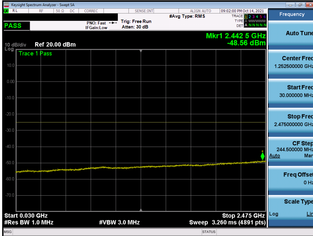
Plot 7-138. Conducted Spurious Plot (NR Band n7 – 40MHz QPSK – RB Size 1, RB Offset 0 – High Channel Ant B)
