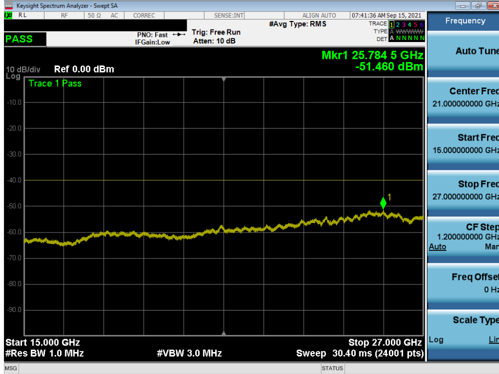
Plot 7-131. Conducted Spurious Plot (NR Band n30 – 10MHz QPSK – RB Size 1, RB Offset 0 – Ant B)
