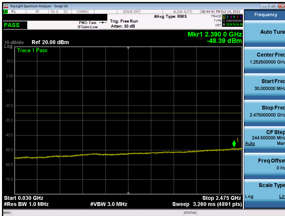
Plot 7-135. Conducted Spurious Plot (NR Band n7 – 40MHz QPSK – RB Size 1, RB Offset 0 – Mid Channel Ant B)
