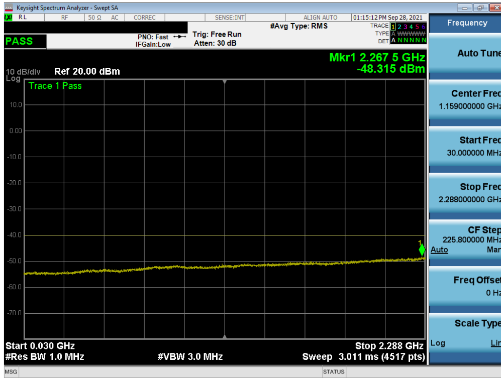
Plot 7-153. Conducted Spurious Plot (NR Band n30 – 10MHz QPSK – RB Size 1, RB Offset 0 – Ant A)
