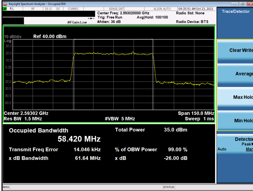
Plot 7-72. Occupied Bandwidth Plot (NR Band n41 – 60MHz \pi/2 BPSK – Full RB – Ant F)
