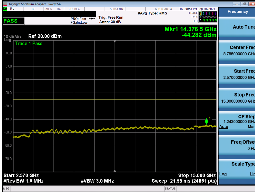
Plot 7-106. Conducted Spurious Plot (LTE Band 7 – 20MHz QPSK – RB Size 1, RB Offset 0 – Mid Channel)
