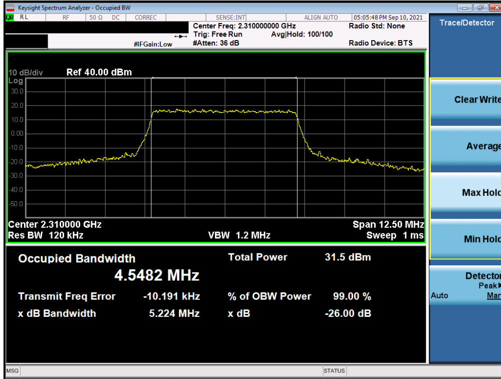
Plot 7-3. Occupied Bandwidth Plot (LTE Band 30 – 5MHz QPSK – Full RB – Ant B)
