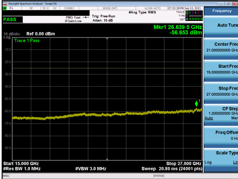
Plot 7-104. Conducted Spurious Plot (LTE Band 7 – 20MHz QPSK – RB Size 1, RB Offset 0 – Low Channel)
