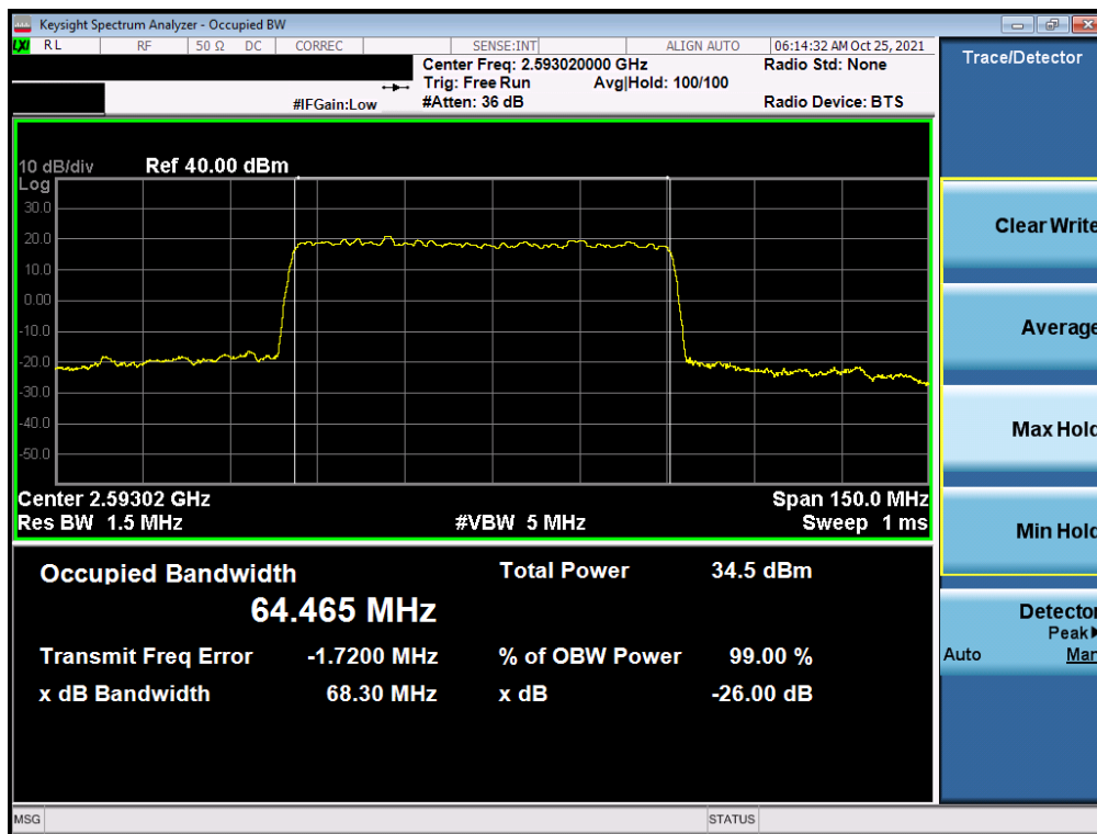
Plot 7-69. Occupied Bandwidth Plot (NR Band n41 – 70MHz \pi/2 BPSK – Full RB – Ant F)
