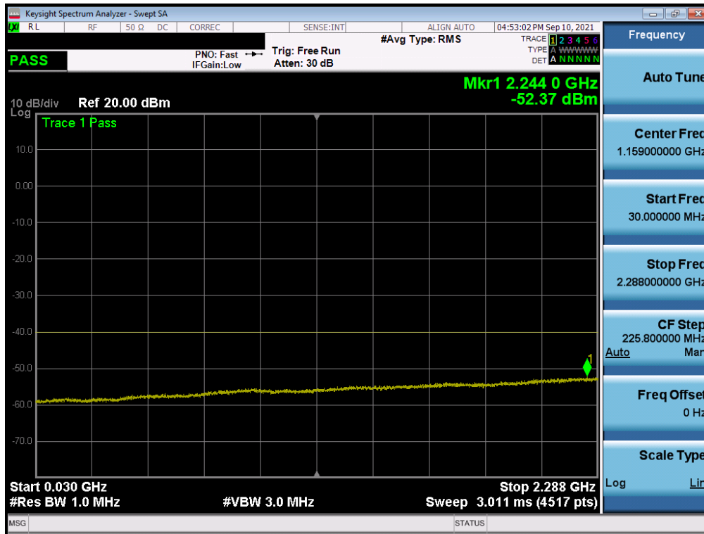
Plot 7-99. Conducted Spurious Plot (LTE Band 30 – 10MHz QPSK – RB Size 1, RB Offset 0 – Ant B)
