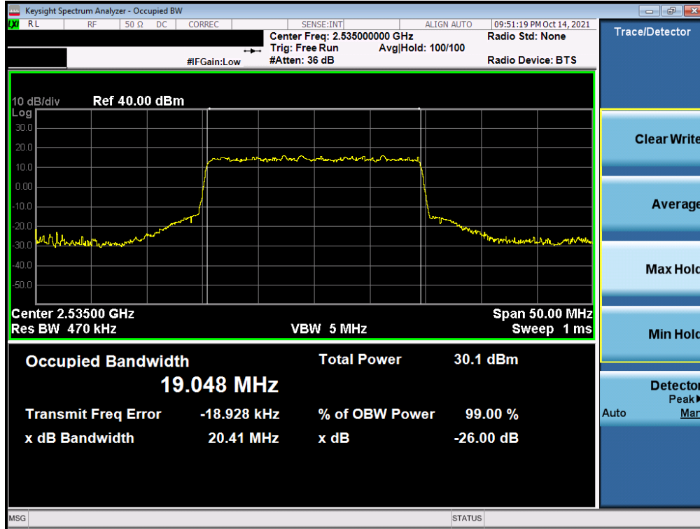
Plot 7-49. Occupied Bandwidth Plot (NR Band n7 – 20MHz QPSK – Full RB – Ant B)
