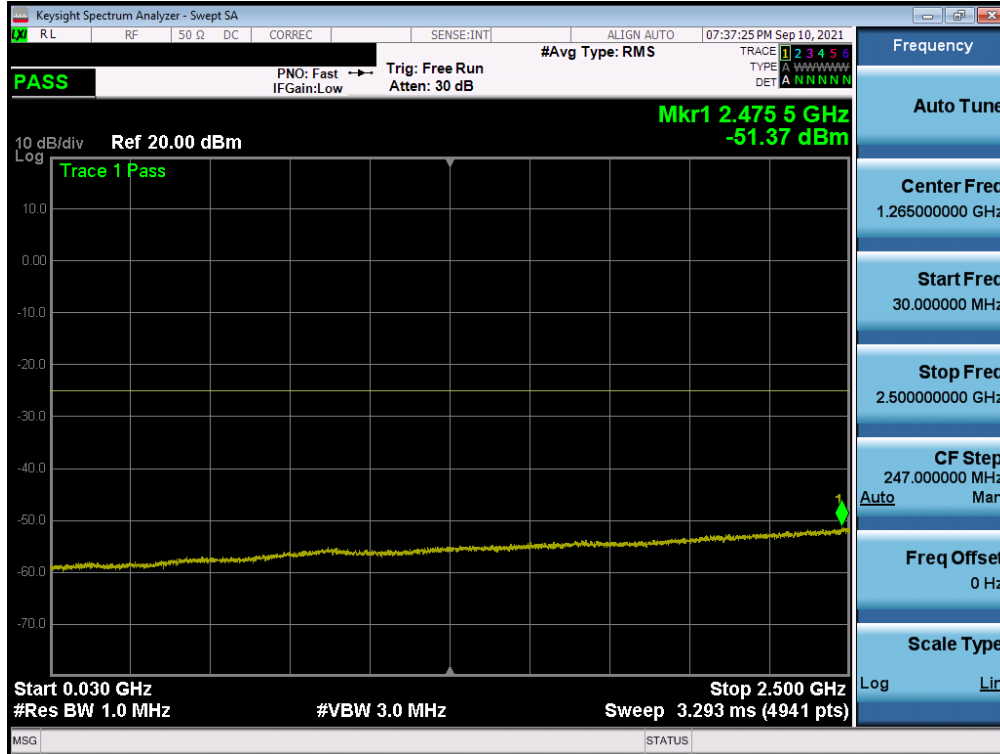
Plot 7-108. Conducted Spurious Plot (LTE Band 7 – 20MHz QPSK – RB Size 1, RB Offset 0 – High Channel)
