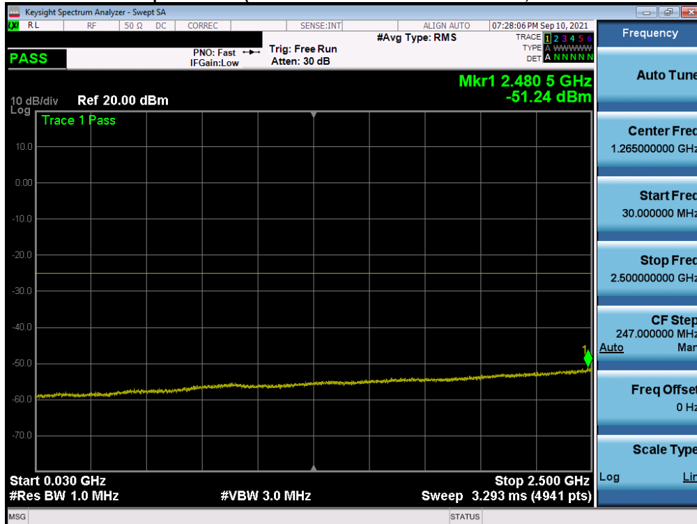
Plot 7-105. Conducted Spurious Plot (LTE Band 7 – 20MHz QPSK – RB Size 1, RB Offset 0 – Mid Channel)
