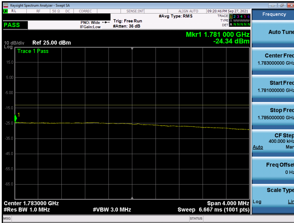
Plot 7-283. Upper Extended Band Edge Plot (NR Band n66 – 40.0MHz - Full RB – ANT F)
