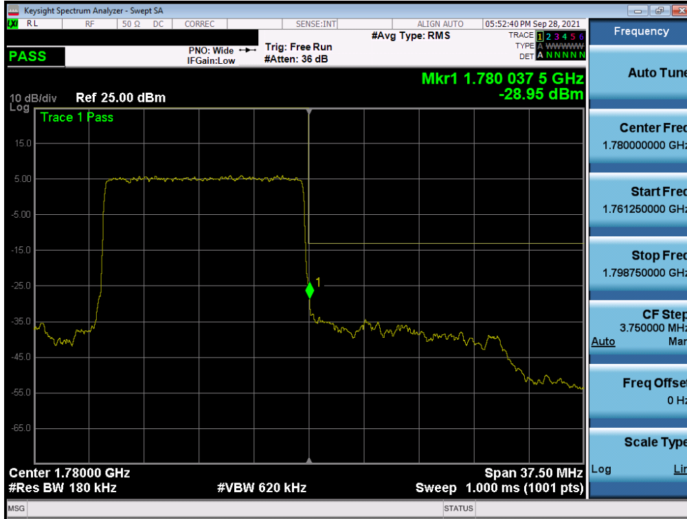
Plot 7-294. Upper Band Edge Plot (NR Band n66 – 15.0MHz - Full RB – ANT F)
