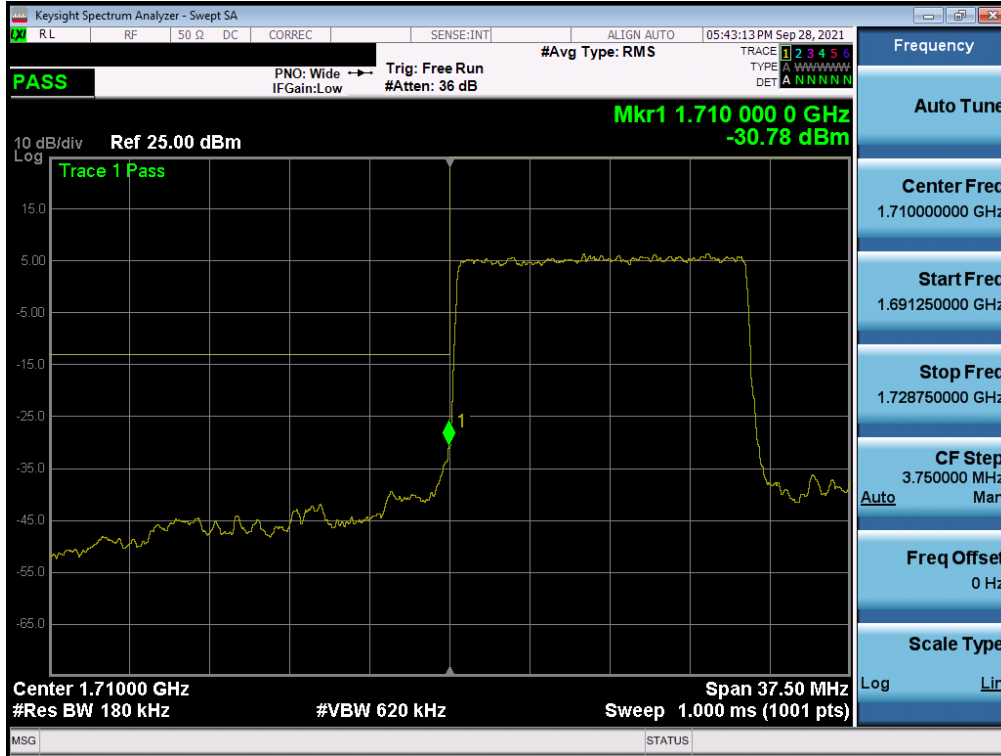
Plot 7-292. Lower Band Edge Plot (NR Band n66 – 15.0MHz - Full RB – ANT F)
