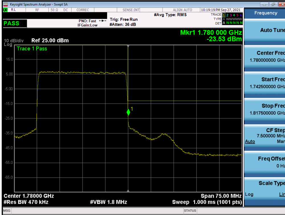
Plot 7-286. Upper Band Edge Plot (NR Band n66 – 30.0MHz - Full RB – ANT F)
