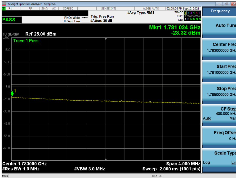
Plot 7-263. Upper Extended Band Edge Plot (NR Band n66 – 30.0MHz - Full RB – ANT A)
