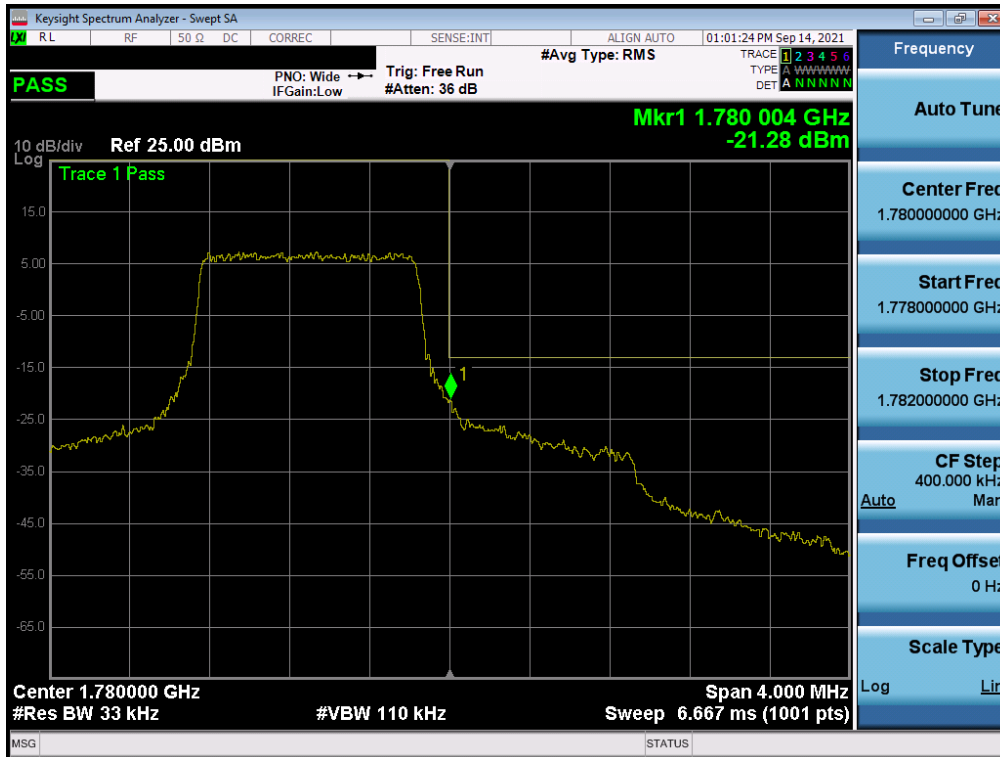
Plot 7-254. Upper Band Edge Plot (LTE Band 66 – 1.4MHz QPSK – Full RB)
