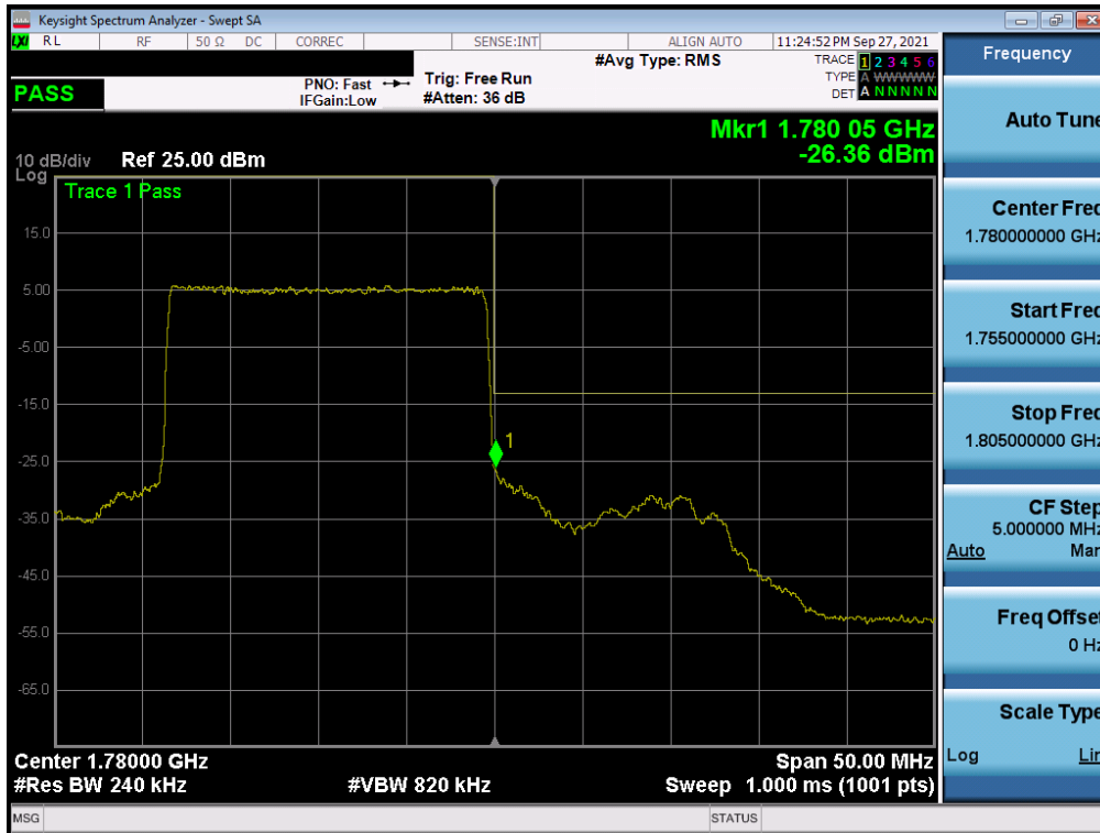
Plot 7-290. Upper Band Edge Plot (NR Band n66 – 20.0MHz - Full RB – ANT F)
