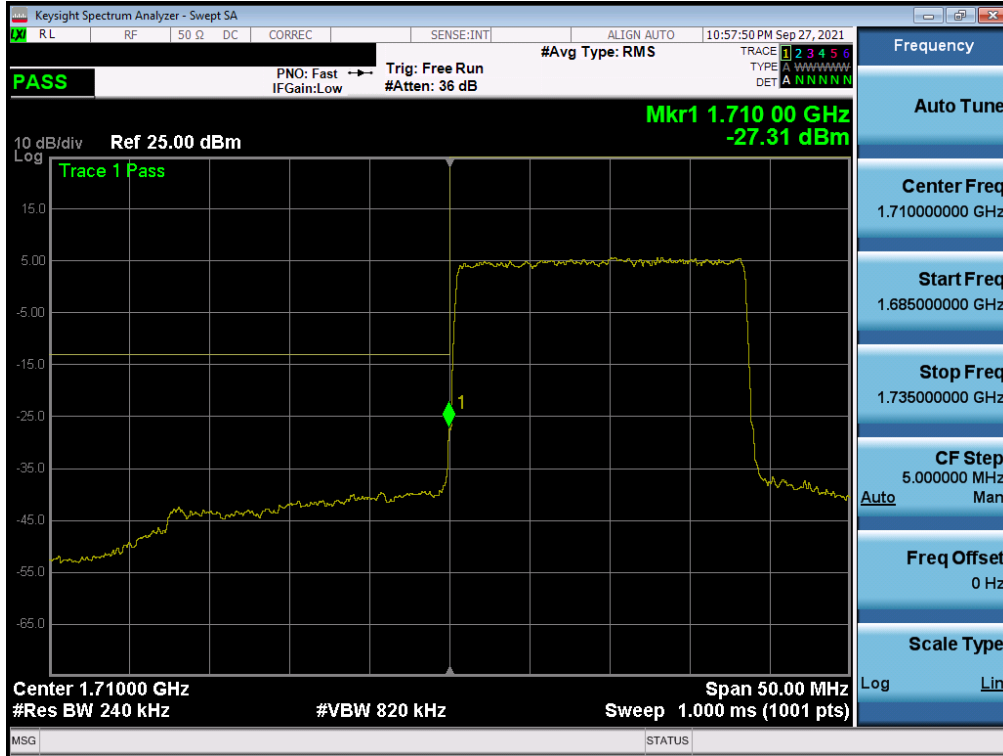
Plot 7-288. Lower Band Edge Plot (NR Band n66 – 20.0MHz - Full RB – ANT F)
