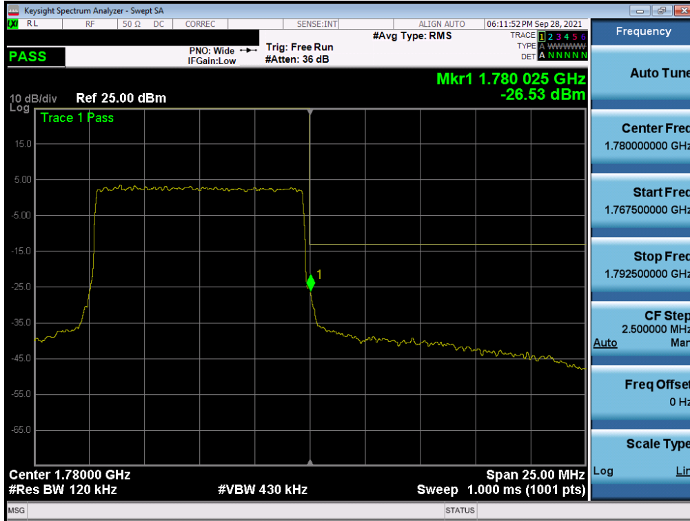
Plot 7-298. Upper Band Edge Plot (NR Band n66 – 10.0MHz - Full RB – ANT F)
