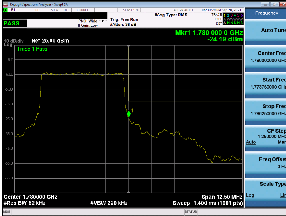
Plot 7-302. Upper Band Edge Plot (NR Band n66 – 5.0MHz - Full RB – ANT F)
