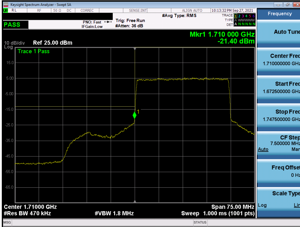
Plot 7-284. Lower Band Edge Plot (NR Band n66 – 30.0MHz - Full RB – ANT F)
