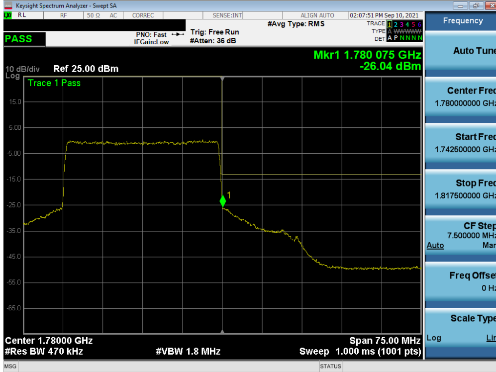
Plot 7-262. Upper Band Edge Plot (NR Band n66 – 30.0MHz - Full RB – ANT A)
