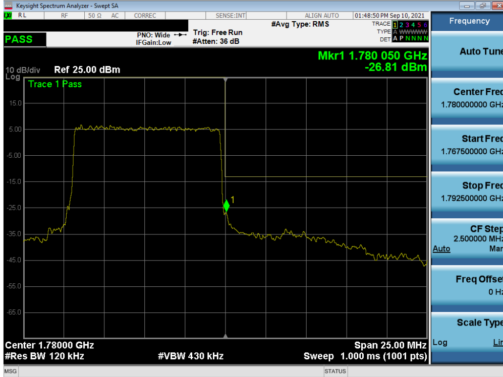
Plot 7-274. Upper Band Edge Plot (NR Band n66 – 10.0MHz - Full RB – ANT A)
