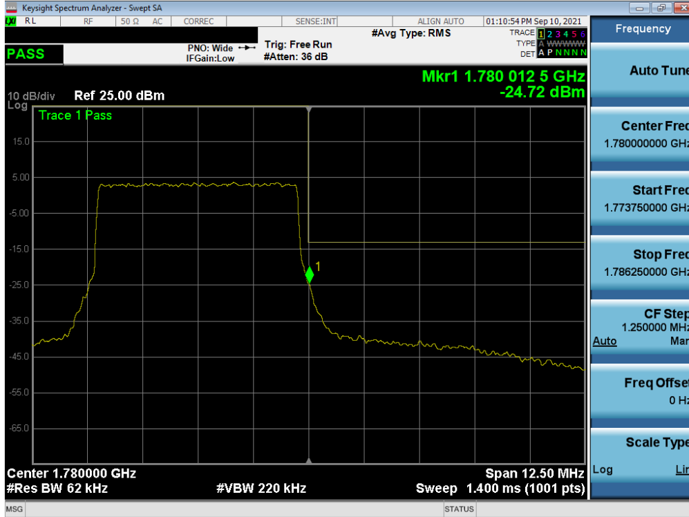
Plot 7-278. Upper Band Edge Plot (NR Band n66 – 5.0MHz - Full RB – ANT A)
