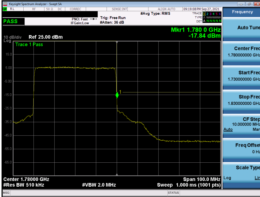
Plot 7-282. Upper Band Edge Plot (NR Band n66 – 40.0MHz - Full RB – ANT F)
