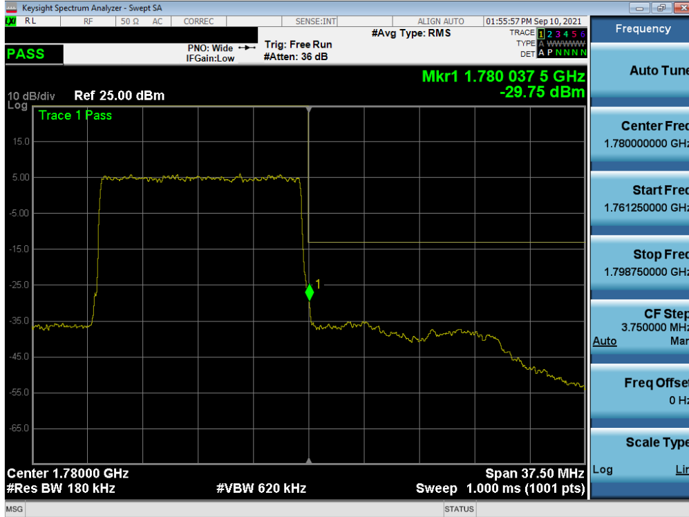
Plot 7-270. Upper Band Edge Plot (NR Band n66 – 15.0MHz - Full RB – ANT A)
