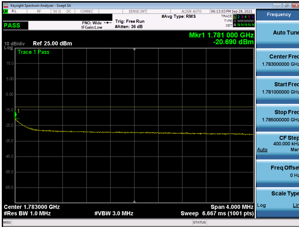
Plot 7-299. Upper Extended Band Edge Plot (NR Band n66 – 10.0MHz - Full RB – ANT F)
