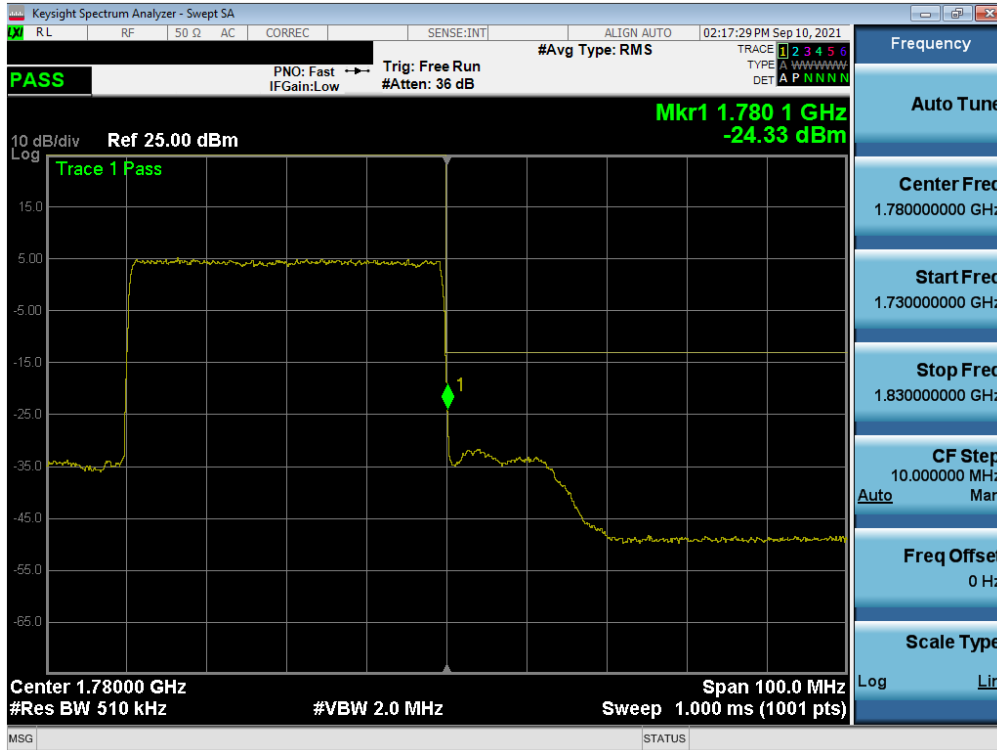
Plot 7-258. Upper Band Edge Plot (NR Band n66 – 40.0MHz - Full RB – ANT A)
