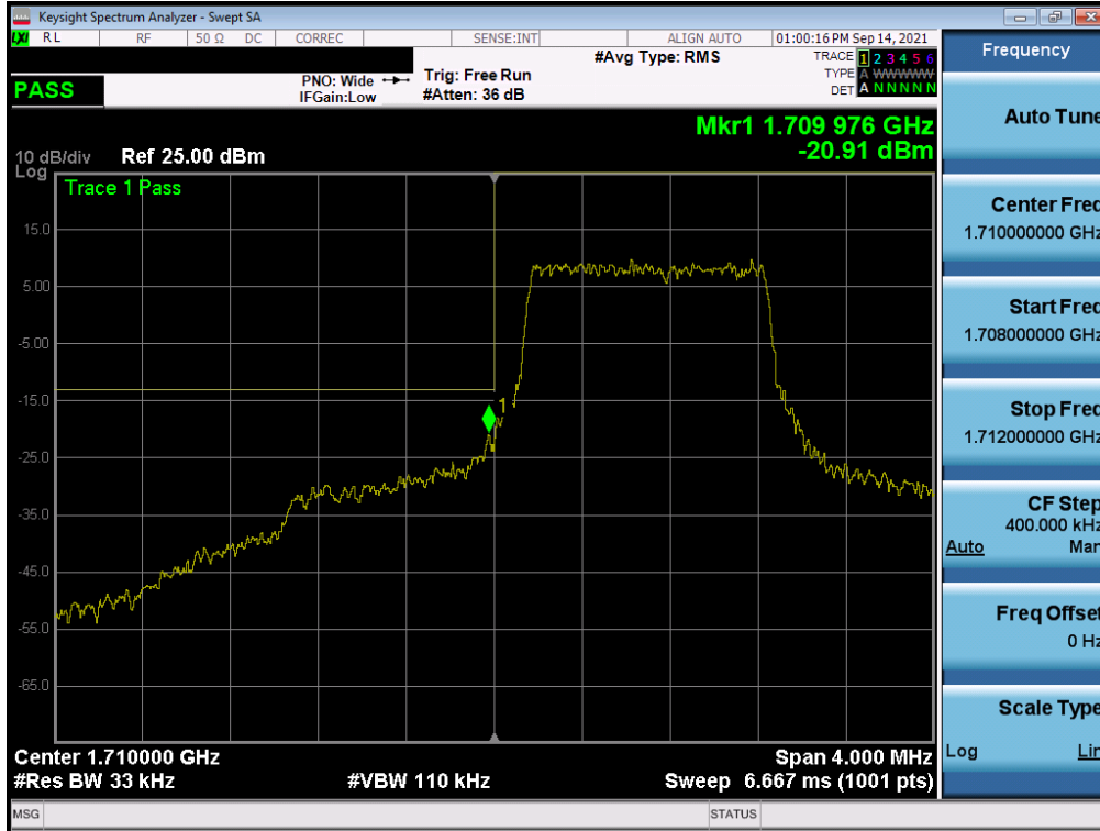
Plot 7-250. Lower Band Edge Plot (LTE Band 66/4 – 1.4MHz QPSK – Full RB)
