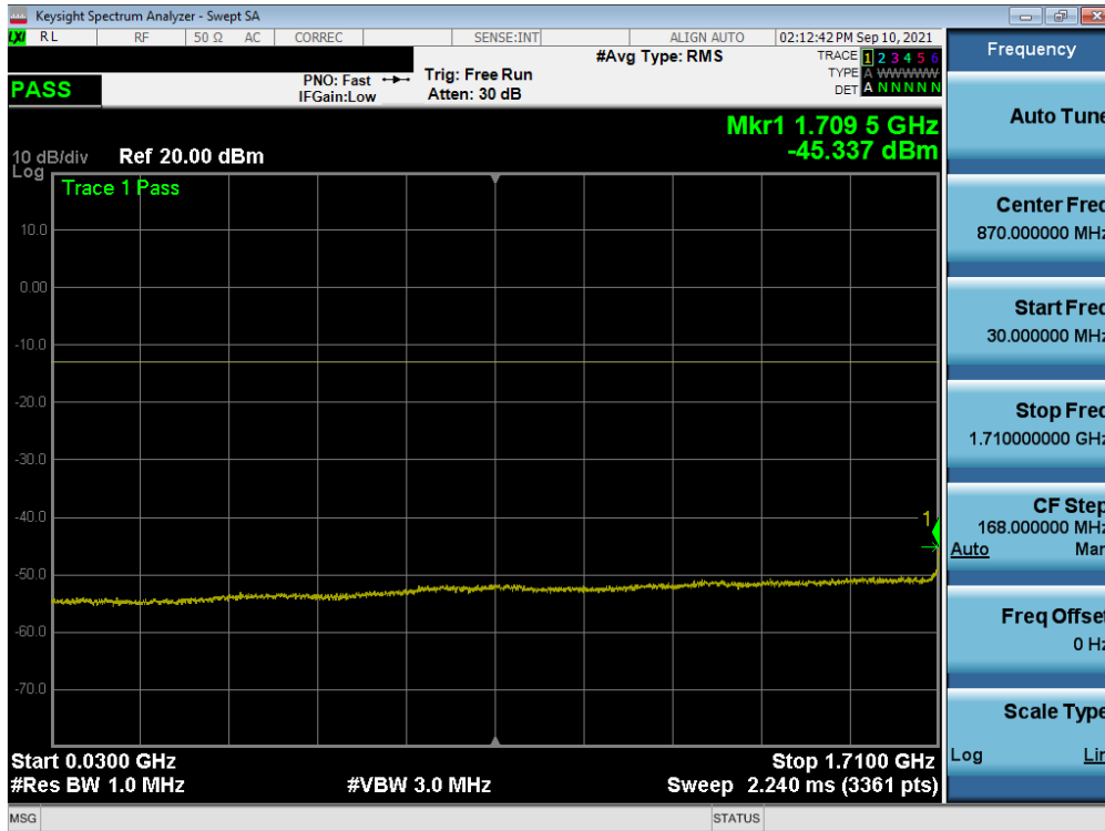
Plot 7-148. Conducted Spurious Plot (NR Band n66 -40.0MHz - 1 RB - Low Channel – ANT A)
