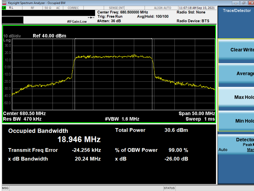
Plot 7-23. Occupied Bandwidth Plot (NR Band n71 - 20MHz CP-OFDM 16-QAM - Full RB)
