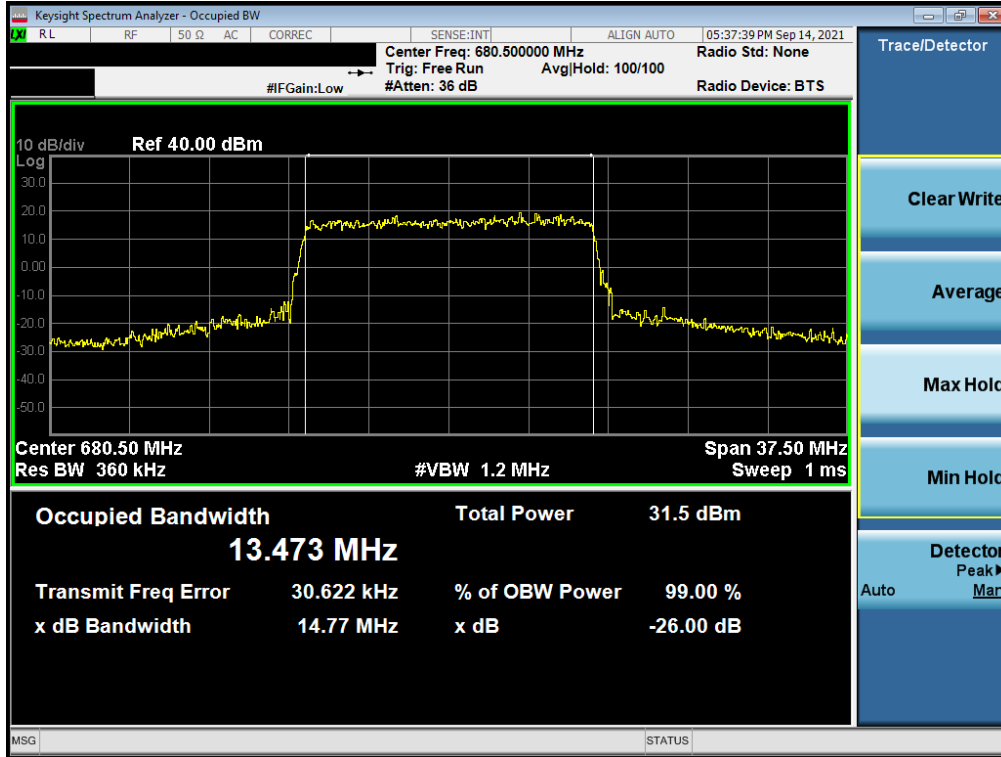
Plot 7-3. Occupied Bandwidth Plot (LTE Band 71 - 15MHz QPSK - Full RB)
