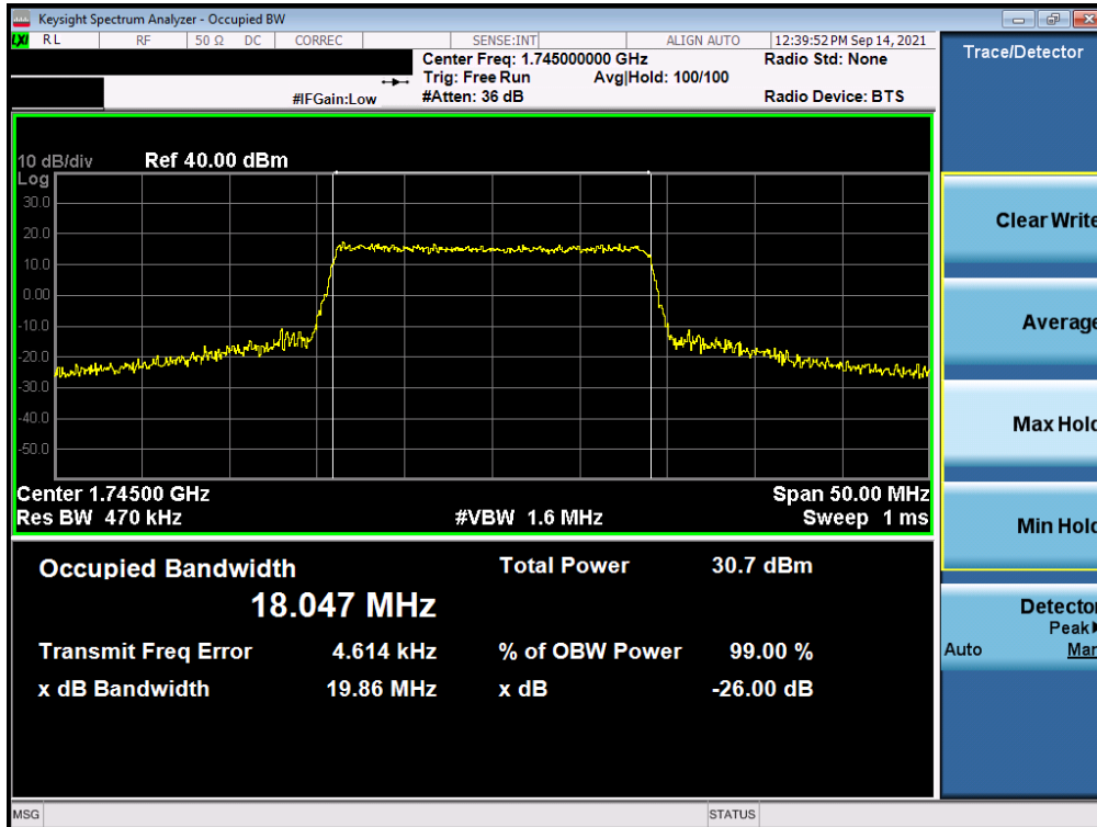
Plot 7-44. Occupied Bandwidth Plot (LTE Band 66/4 - 20MHz 16-QAM - Full RB)
