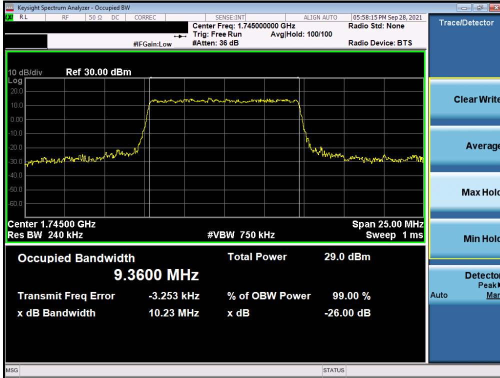
Plot 7-87. Occupied Bandwidth Plot (NR Band n66 - 10.0MHz CP-OFDM 16QAM - Full RB - ANT F)
