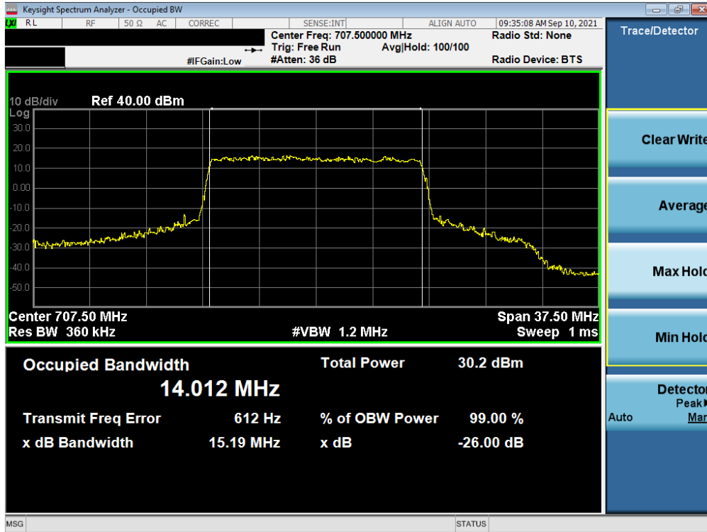
Plot 7-35. Occupied Bandwidth Plot (NR Band n12 - 15MHz CP-OFDM 16-QAM - Full RB)
