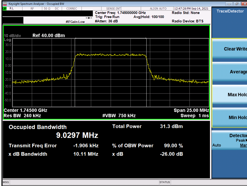
Plot 7-47. Occupied Bandwidth Plot (LTE Band 66/4 - 10MHz QPSK - Full RB)
