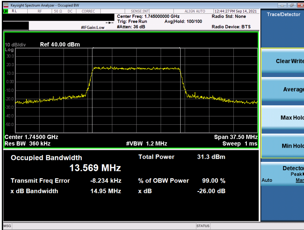
Plot 7-45. Occupied Bandwidth Plot (LTE Band 66/4 - 15MHz QPSK - Full RB)
