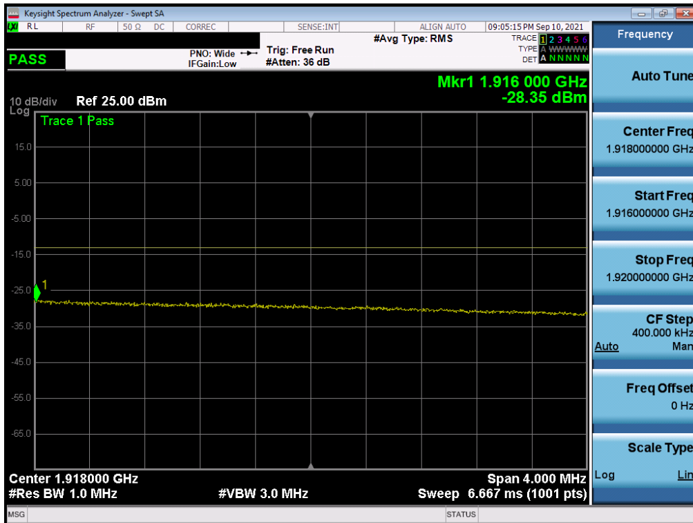
Plot 7-108. Extended Upper Band Edge Plot (LTE Band 25 - 20MHz QPSK – Full RB)
