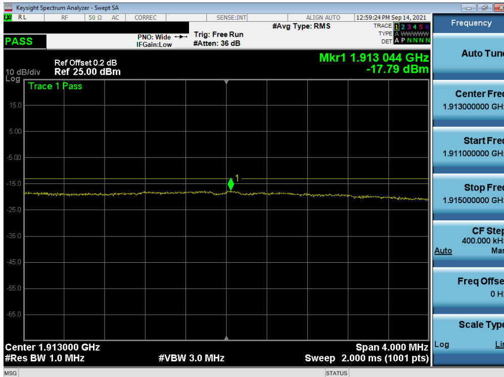
Plot 7-160. Extended Upper Band Edge Plot (NR Band n2 - 15MHz QPSK – Full RB - Ant A)
