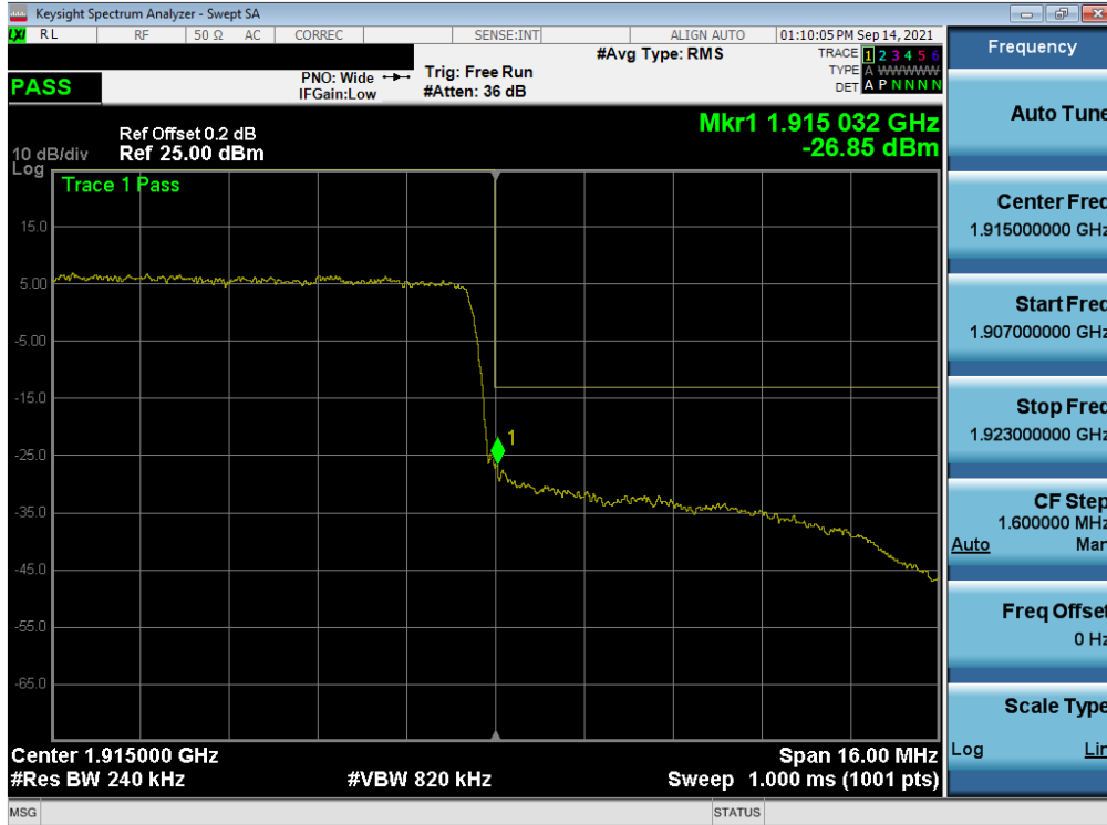
Plot 7-155. Upper Band Edge Plot (NR Band n25 - 20MHz QPSK – Full RB - Ant A)
