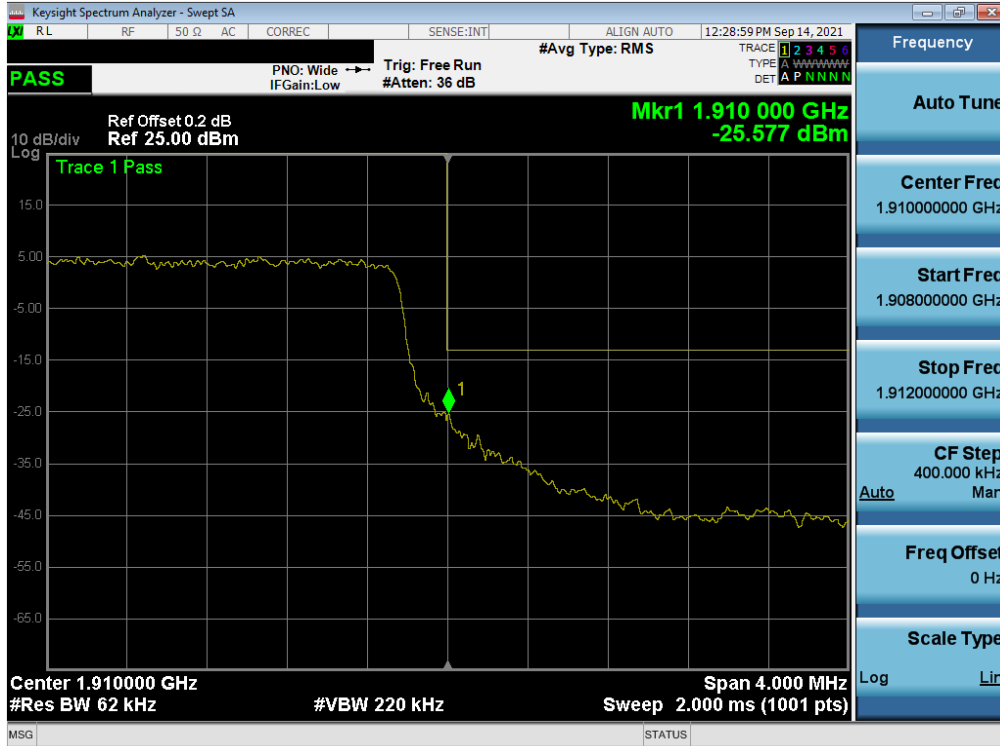
Plot 7-171. Upper Band Edge Plot (NR Band n2 – 5MHz QPSK – Full RB - Ant A)
