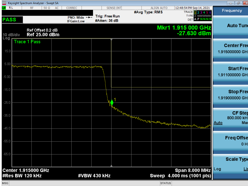
Plot 7-167. Upper Band Edge Plot (NR Band n25 - 10MHz QPSK – Full RB - Ant A)
