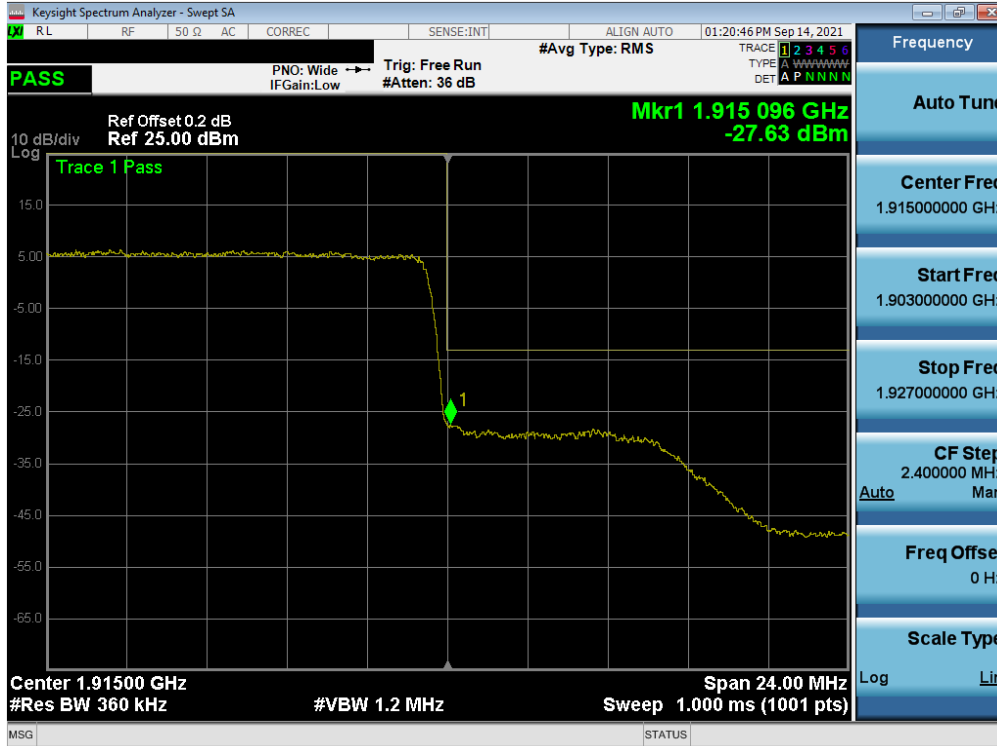
Plot 7-145. Upper Band Edge Plot (NR Band n25 - 30MHz QPSK – Full RB - Ant A)
