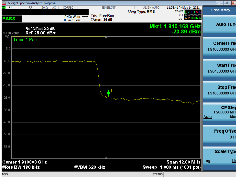
Plot 7-159. Upper Band Edge Plot (NR Band n2 - 15MHz QPSK – Full RB - Ant A)
