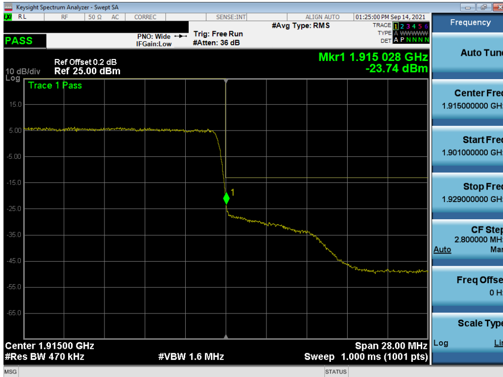
Plot 7-141. Upper Band Edge Plot (NR Band n25 - 40MHz QPSK – Full RB - Ant A)
