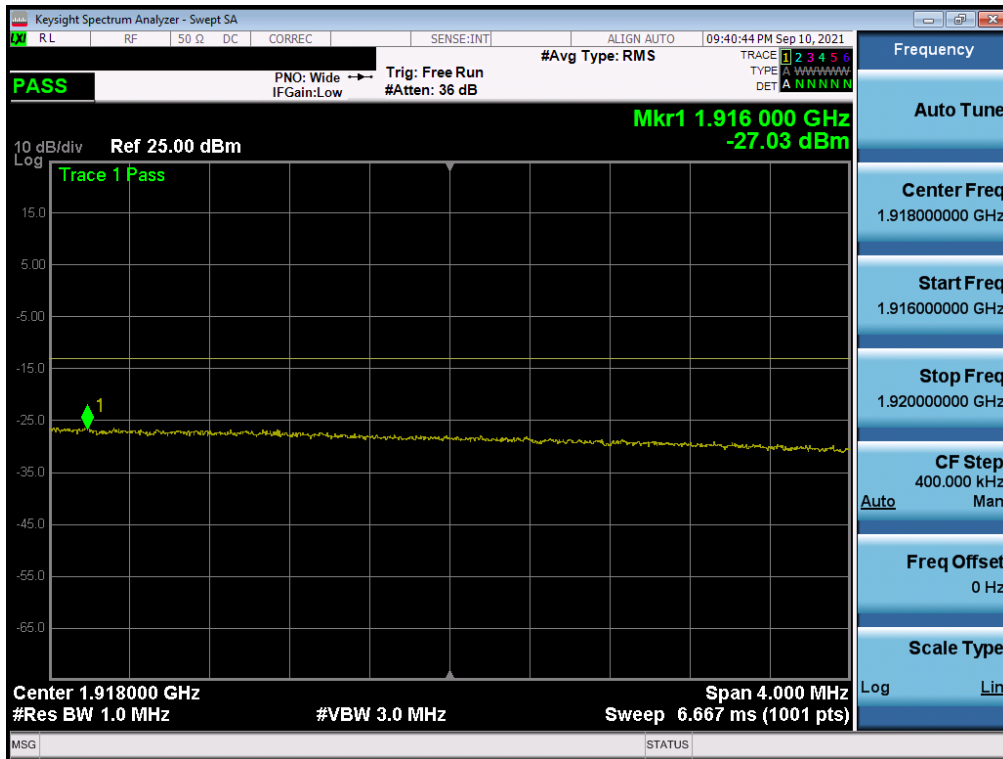
Plot 7-114. Extended Upper Band Edge Plot (LTE Band 25 - 15MHz QPSK – Full RB)
