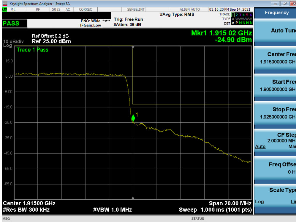
Plot 7-149. Upper Band Edge Plot (NR Band n25 - 25MHz QPSK – Full RB - Ant A)
