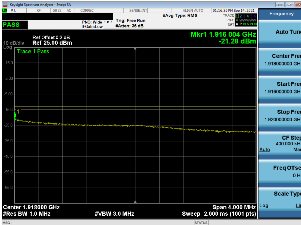
Plot 7-150. Extended Upper Band Edge Plot (NR Band n25 - 25MHz QPSK – Full RB - Ant A)
