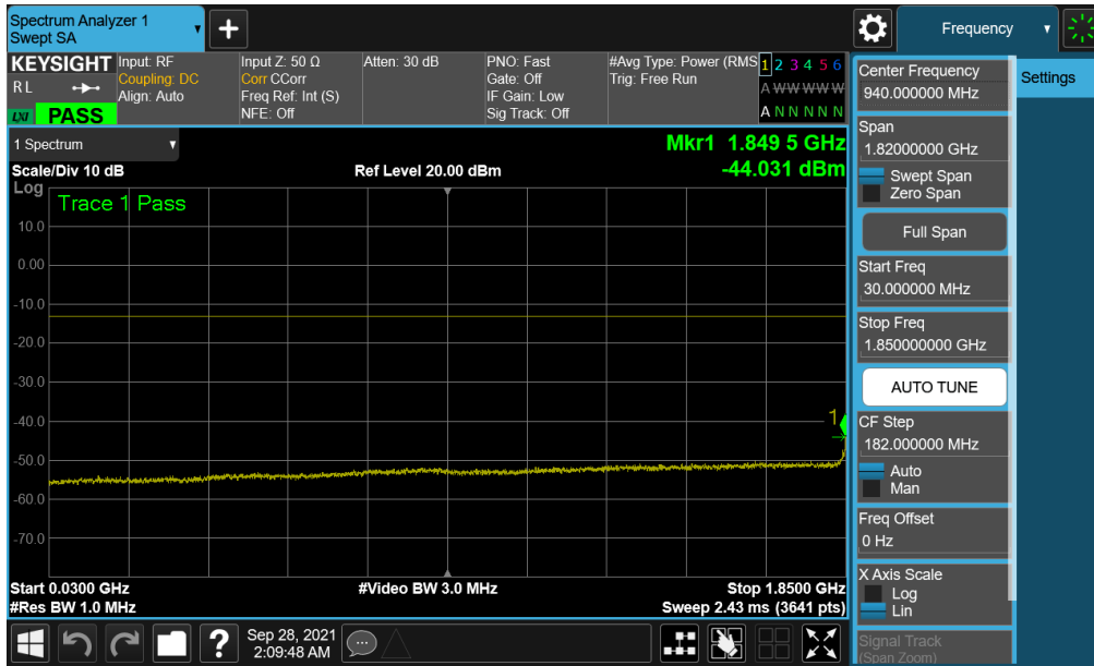
Plot 7-76. Conducted Spurious Plot (NR Band n25/2 -40.0MHz - 1RB - Low Channel - Ant F)
