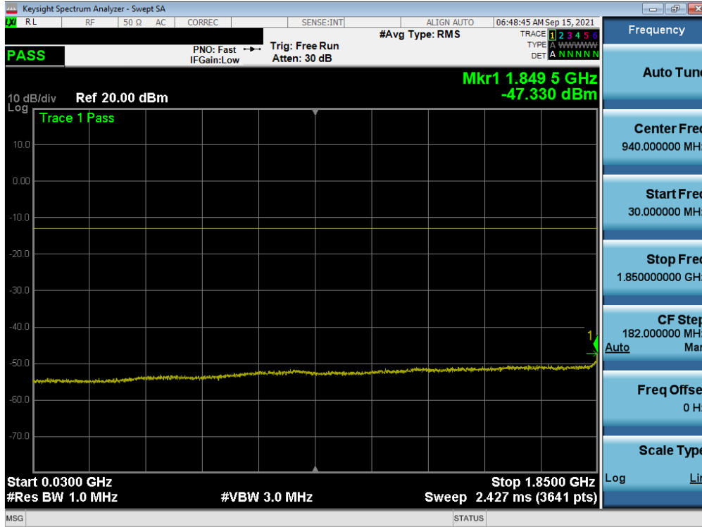
Plot 7-67. Conducted Spurious Plot (NR Band n25/2 -40.0MHz - 1RB - Low Channel - Ant A)
