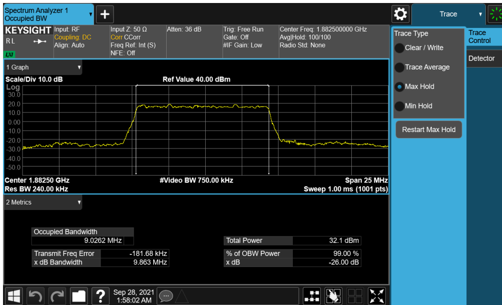
Plot 7-49. Occupied Bandwidth Plot (NR Band n25/2 - 10.0MHz DFT-s-OFDM BPSK - Full RB - ANT F)
