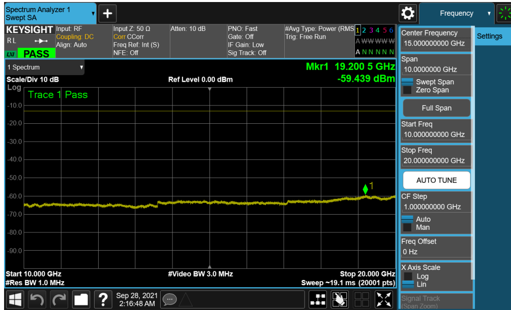
Plot 7-84. Conducted Spurious Plot (NR Band n25/2 - 40.0MHz - 1RB - High Channel - Ant F)
