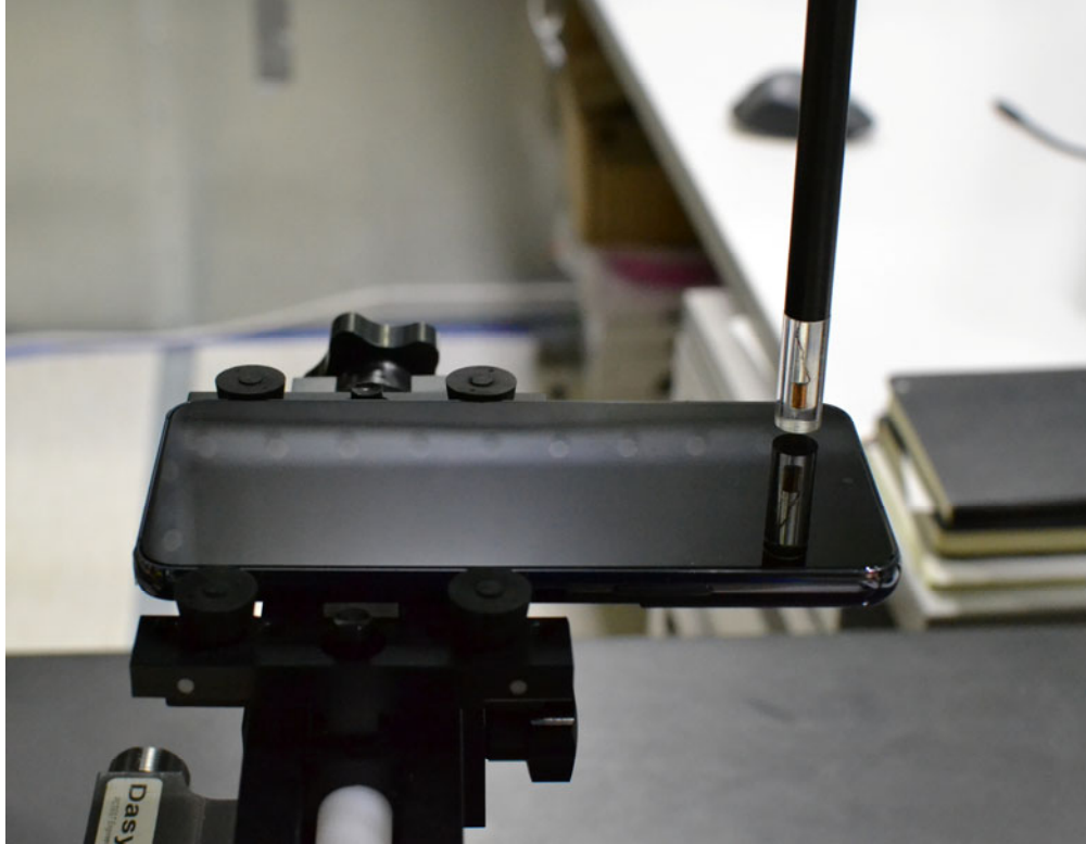
Figure 17-1 Test Setup for Wireless Device
