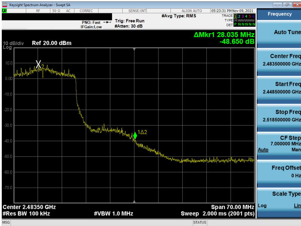
Plot 7-105. Band Edge Plot SISO ANT2 (802.11ax (2.4GHz) – Ch. 10)
