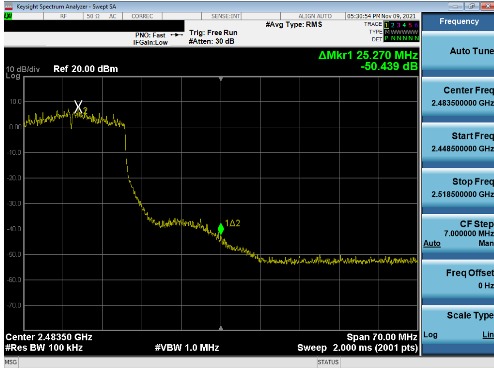
Plot 7-87. Band Edge Plot SISO ANT1 (802.11ax (2.4GHz) – Ch. 10)
