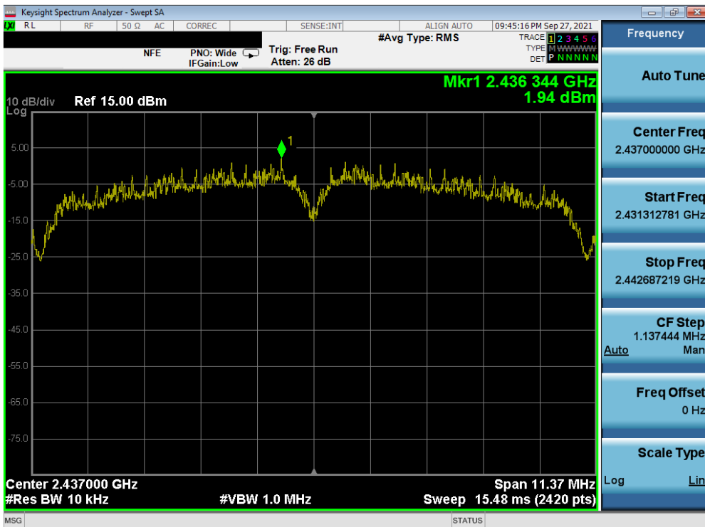
Plot 7-62. Power Spectral Density Plot MIMO ANT2 (802.11b (2.4GHz) – Ch. 6)
