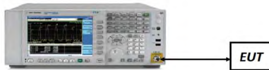
Figure 7-1. Test Instrument & Measurement Setup
