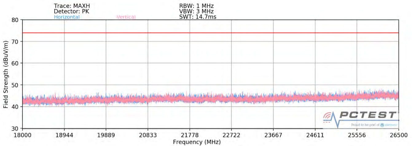
Plot 7-74. Radiated Spurious Plot above 18GHz SISO ANT1 (802.11ax OFDMA – 242 Tones)
