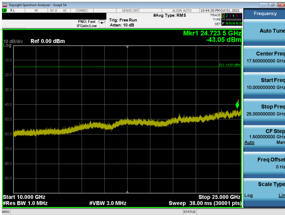
Plot 7-46. Conducted Spurious Plot SISO ANT1 (802.11ax OFDMA – 26 Tones – Ch. 6)
