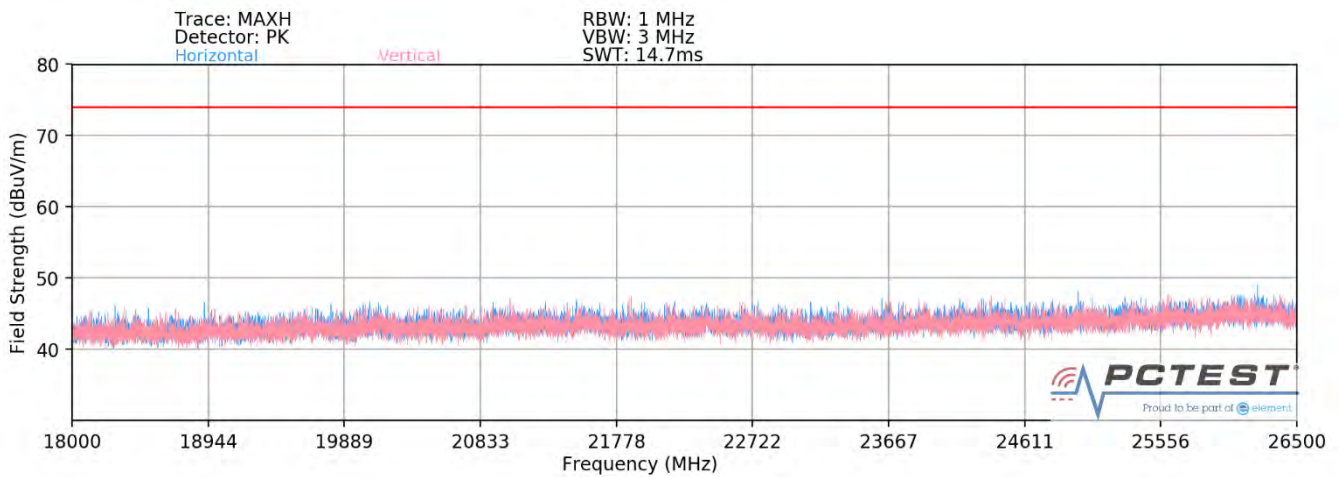
Plot 7-82. Radiated Spurious Plot above 18GHz SISO ANT2 (802.11ax OFDMA – 242 Tones)
