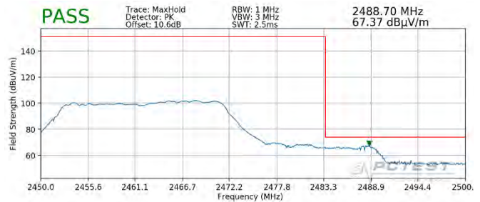
Plot 7-122. Radiated Restricted Upper Band Edge Measurement SISO ANT2 (Peak – 242 Tones)
