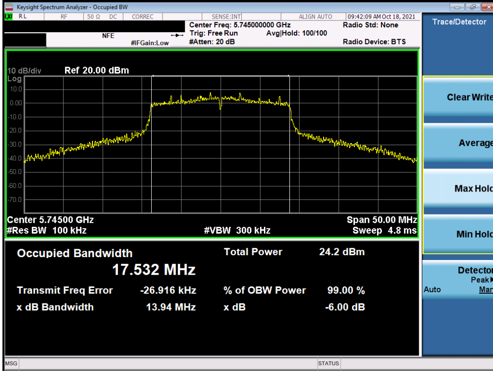
Plot 7-106. 6dB Bandwidth Plot SISO ANT1 (20MHz BW 802.11n (UNII Band 3) – Ch. 149)
