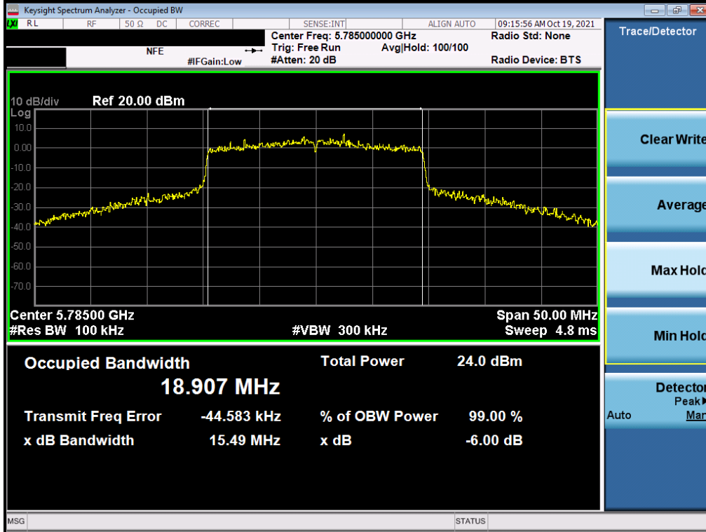
Plot 7-110. 6dB Bandwidth Plot SISO ANT1 (20MHz BW 802.11ax (UNII Band 3) – Ch. 157)
