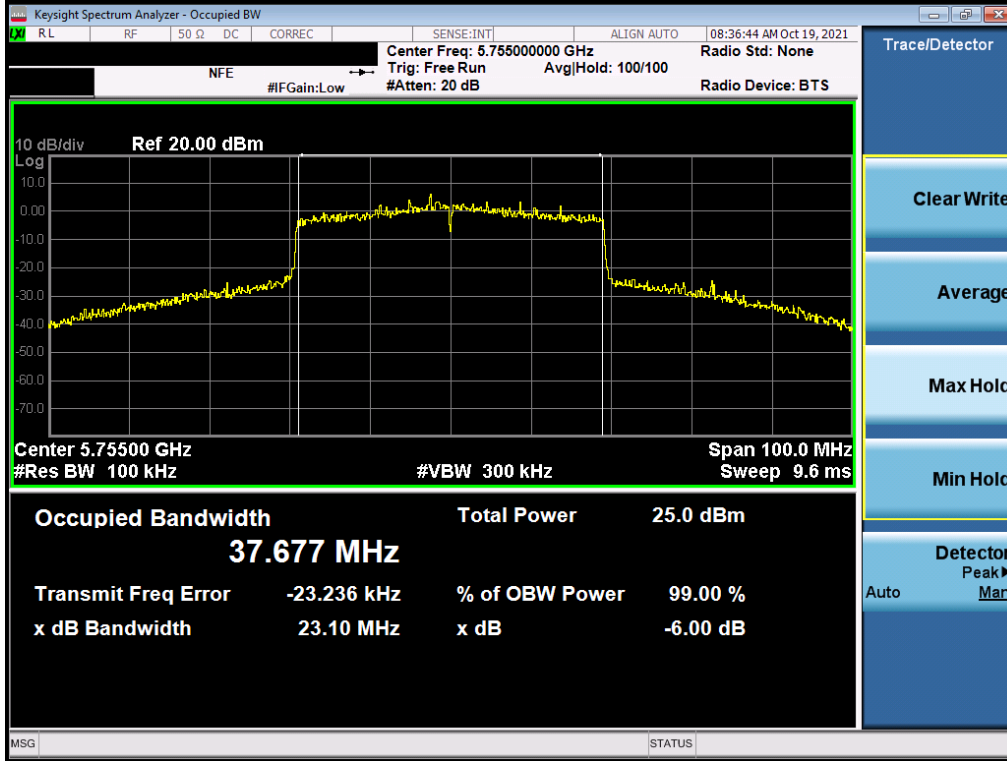
Plot 7-143. 6dB Bandwidth Plot SISO ANT2 (40MHz BW 802.11ax (UNII Band 3) – Ch. 151)
