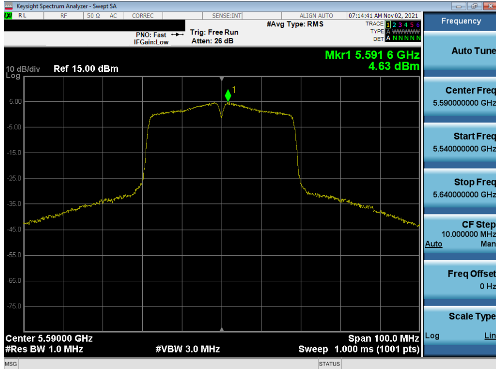
Plot 7-201. Power Spectral Density Plot SISO ANT1 (40MHz BW 802.11n (UNII Band 2C) – Ch. 118)
