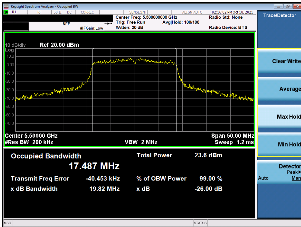
Plot 7-85. 26dB Bandwidth Plot SISO ANT2 (20MHz BW 802.11n (UNII Band 2C) – Ch. 100)
