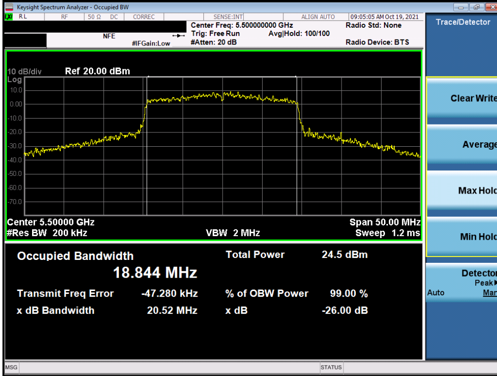
Plot 7-37. 26dB Bandwidth Plot SISO ANT1 (20MHz BW 802.11ax (UNII Band 2C) – Ch. 100)
