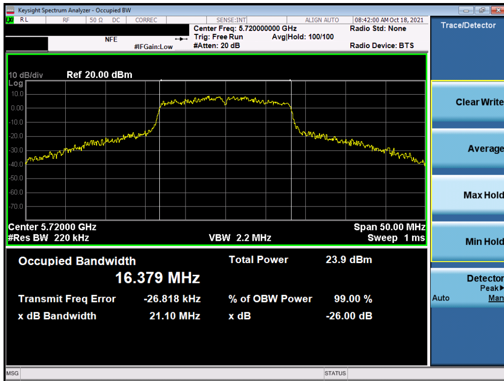
Plot 7-33. 26dB Bandwidth Plot SISO ANT1 (802.11a (UNII Band 2C) – Ch. 144)
