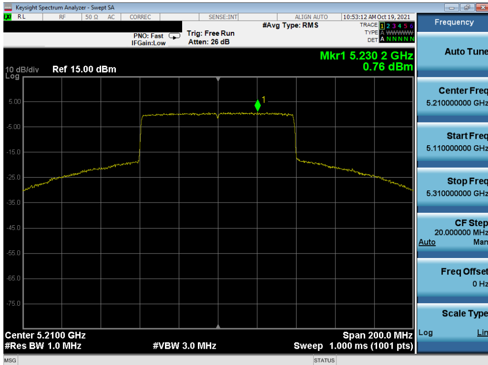
Plot 7-171. Power Spectral Density Plot SISO ANT1 (80MHz BW 802.11ax – Full Tones (UNII Band 1) – Ch. 42)
