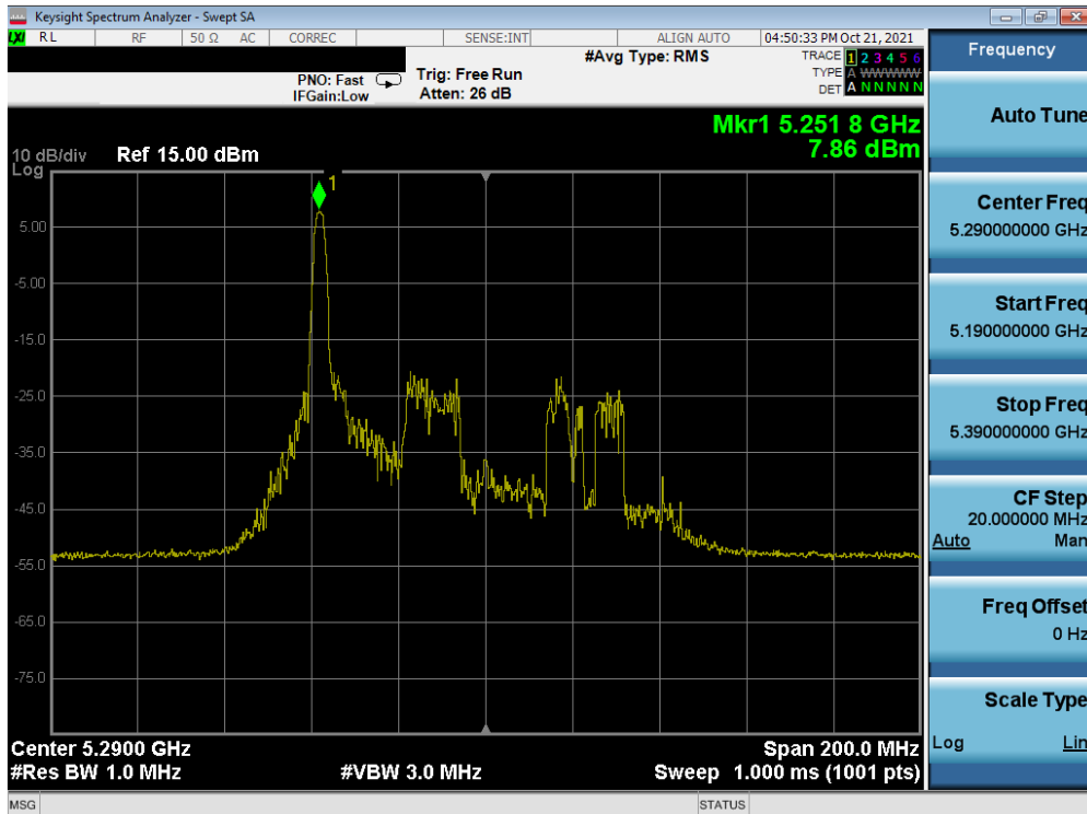
Plot 7-210. Power Spectral Density Plot SISO ANT2 (80MHz BW 802.11ax – 26 Tones (UNII Band 2A) – Ch. 58)
