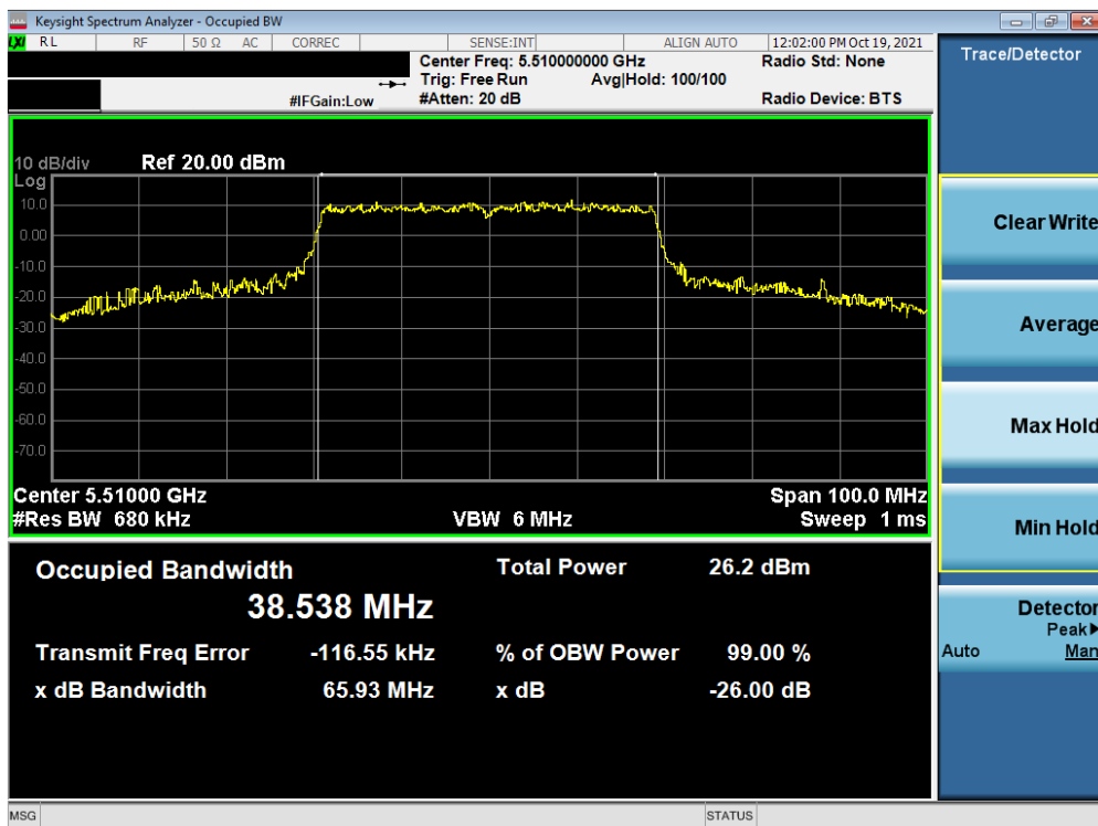
Plot 7-79. 26dB Bandwidth Plot SISO ANT2 (40MHz BW 802.11ax – 484 Tones (UNII Band 2C) – Ch. 102)
