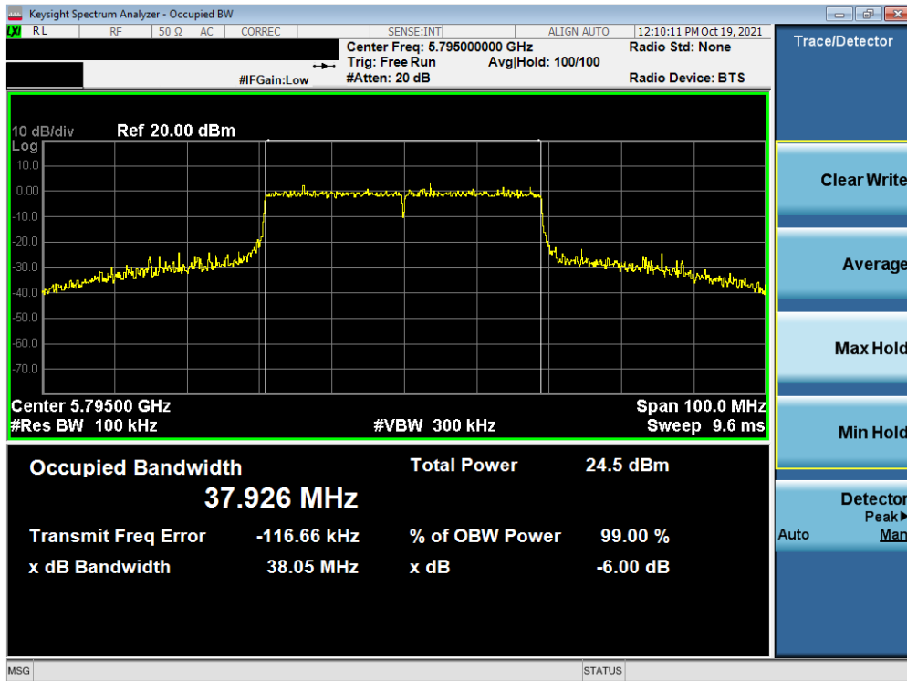
Plot 7-125. 6dB Bandwidth Plot SISO ANT2 (40MHz BW 802.11ax – 484 Tones (UNII Band 3) – Ch. 159)
