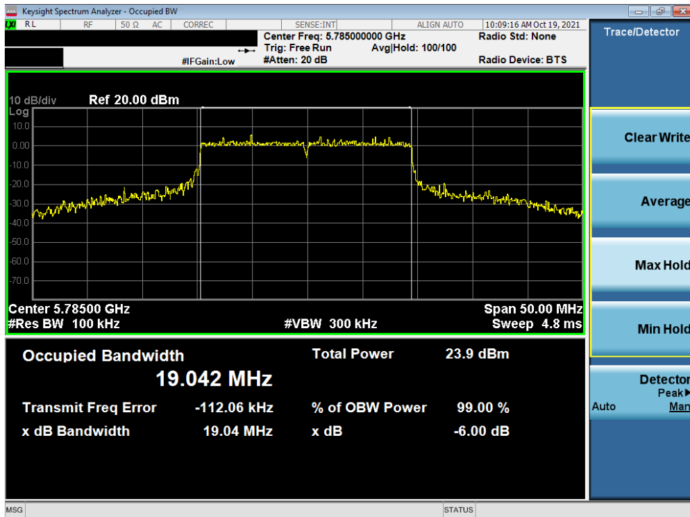
Plot 7-98. 6dB Bandwidth Plot SISO ANT1 (20MHz BW 802.11ax – 242 Tones (UNII Band 3) – Ch. 157)
