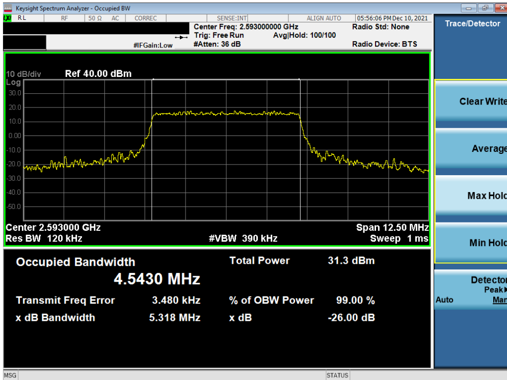
Plot 7-8. Occupied Bandwidth Plot (LTE Band 41(PC3) - 5MHz 16-QAM - Full RB)
