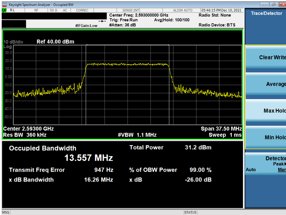
Plot 7-4. Occupied Bandwidth Plot (LTE Band 41(PC3) - 15MHz 16-QAM - Full RB)
